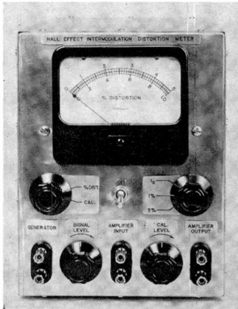
Fig. 12—Hall-Effect Intermodulation Distortion Meter, front view.
