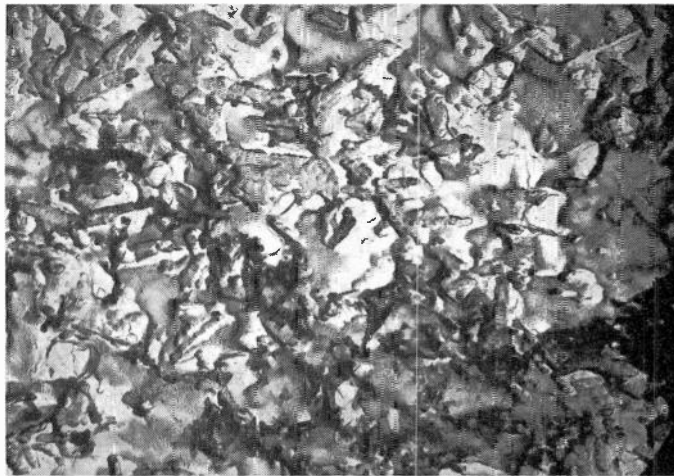
Fig. 1—A replicate of the surface of tape D at 10,000 \times direct magnification.
