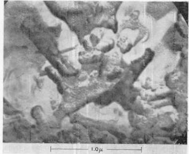
Fig. 4—A replica of the surface of tape D at 40,000X direct magnification.
