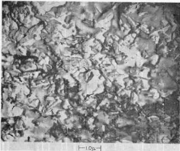
Fig. 3—A replica of the surface of tape D at 10,000X direct magnification.
