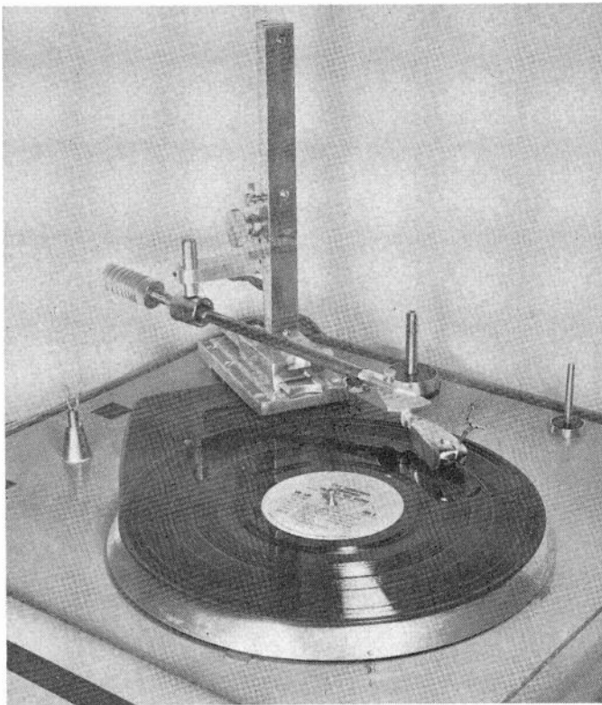
Fig. 11—Turntable and arm arrangement for playing a record forward, backward, at various tracking angles.
