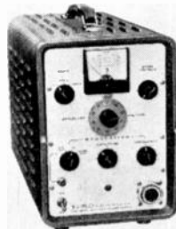
PRD 809-A Klystron Power Supply
