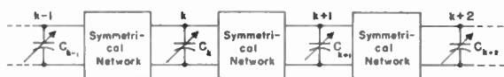
Fig. 1—Symmetrical networks and variable capacitors in cascade. C_k = C_0 + C_1 \cos(\omega t - \gamma k) .
