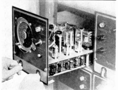
Modular chassis interchangeable with instrument case for dual function or as transport case for replacement chassis.
