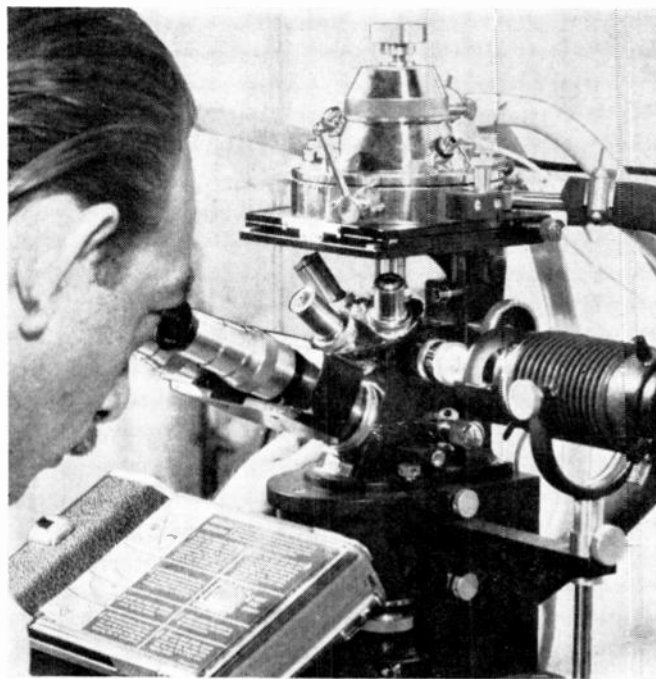
High-power metallurgical microscope with electric furnace—typical of PCI facilities for quality control, reliability and research.
