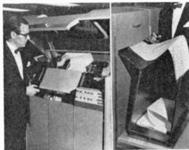
Sales leads through the "Lead-Master" electronic convention process come out of the High Speed Printer at 1500 lines per minute. Each pre-gummed, perforated label contains the personal information of an individual who visited a particular booth. The cost to that booth's exhibitor for this lead is about 3¢. Data Patterns, Incorporated, New York business system specialists, developed the process which will be used for the first time at this year's IRE Convention and Show for 80,000 electronics engineers.
