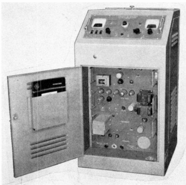
Fig. 22—Mass-spectrometer leak detector (General Electric, M-60).
