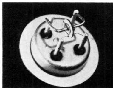
Fig. 17—Field-effect tetrode mounted on header.
