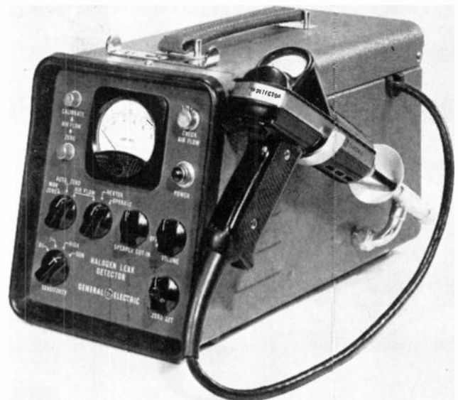
Fig. 24—Gun-type halogen leak detector (General Electric, H-2).
