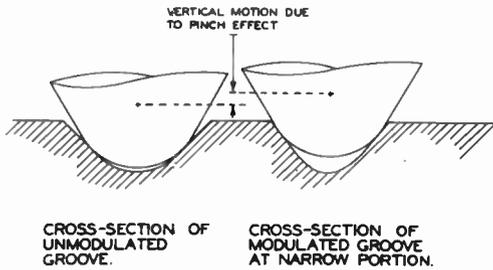
CROSS-SECTION OF UNMODULATED GROOVE. CROSS-SECTION OF MODULATED GROOVE AT NARROW PORTION.
