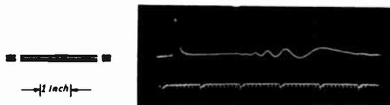
Impulse Response, Helical Delay Line, Phase Corrected
