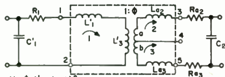
FIG. 5b TRANSFORMER ARRANGED FOR NODAL PROGRAM
