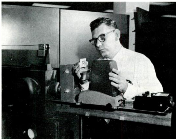
Fig. 1. Photograph of "Dervish." Constructed from 35 mm Cinescanner, with projector replacing flying spot scanner on front end.
