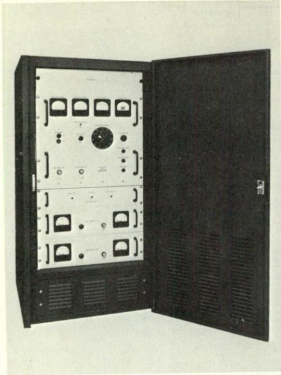
Fig. 10. Transmitter and modulator equipment.
