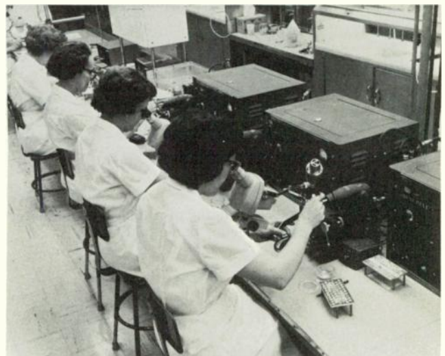
Fig. 7. A portion of the general electric ultrasonic welding facility for the production of silicon rectifiers.
