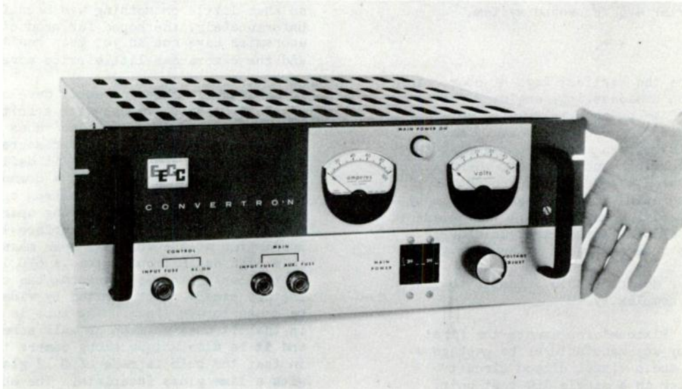
Fig. 21. Photograph of 2 kw, dc output, regulated VWP power supply.
