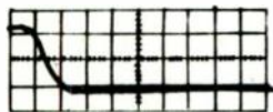
Fig. 5. Input and output waveforms of X40 current amplifier. Time scale 0.1 \mu \text{sec/cm} .
