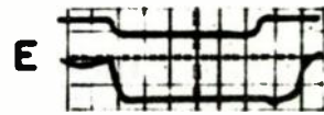
Fig. 6. Overload performance. Input and output waveforms for normal, X 3, X 10, X 30 and X 100 maximum linear operation. Time scale 0.5 \mu \text{sec/cm} .
