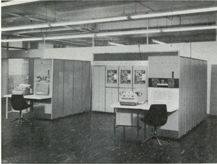
Fig. 3. Dual central processor and magnetic tape transport configuration.
