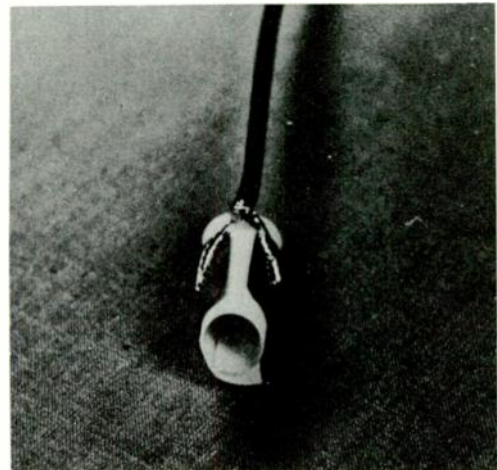
Fig. 4. Capacitive epivascular micrometer during construction.
