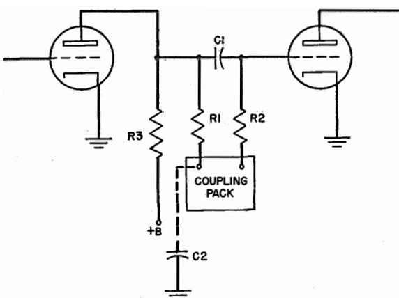
Fig. 8—Method of coupling for low frequencies.
