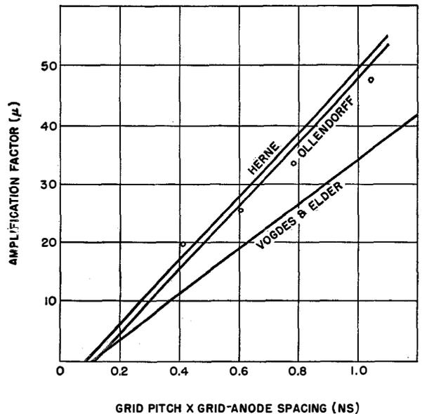
Fig. 4—Experimental and theoretical variation of  $\mu$  with grid-anode spacing for a shadow ratio ( $Nd$ ) = 0.394. The lines are calculated from the formulae of the authors named, while the points represent experimental values.
