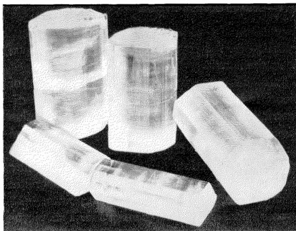
Fig. 3—Large Rochelle salt crystals.
