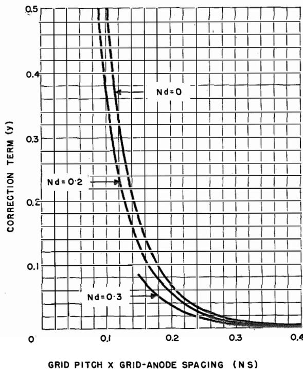
Fig. 11—Curves to be used in correcting Miller's formula when the grid approaches the anode very closely. The correction term  $y$  is obtained from the equation  $\frac{1}{\mu_{11}} = \frac{1}{\mu_M} - y$ , where  $\mu_M$  is Miller's result.
