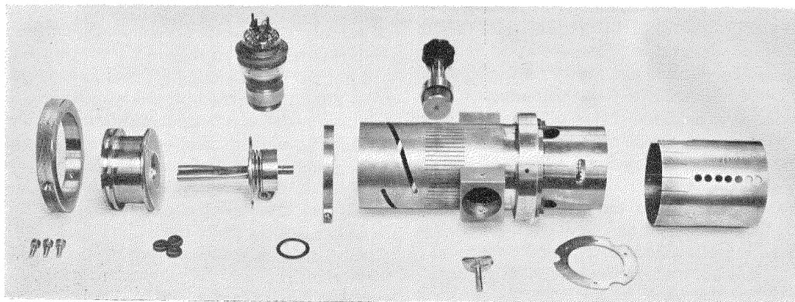
Fig. 6—Exploded view of coaxial amplifier using 6C22 tube at 490 megacycles.
