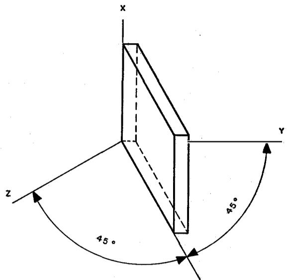
Fig. 11—Rochelle salt plate cut along the *X* axis with its principal plane faces at 45 degrees to the *Y* and *Z* axes. Similar cuts may have the principal face along the *Y* or *Z* axis and at 45 degrees to the other two axes.
