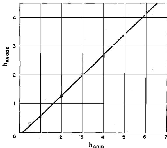
Fig. 9—Results obtained in the measurement of amplification factor on the rubber-sheet model. Grid shadow ratio ( $Nd$ )=0.05, grid-cathode distance ( $l_g$ )=1.6 times grid pitch ( $N$ ), anode-grid distance ( $S$ )=0.2 times grid pitch ( $N$ ).
