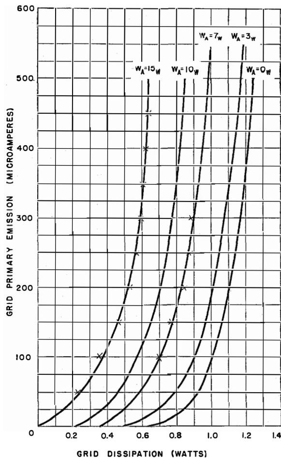
Fig. 3—Grid emission and dissipation for low-power-output valve.
