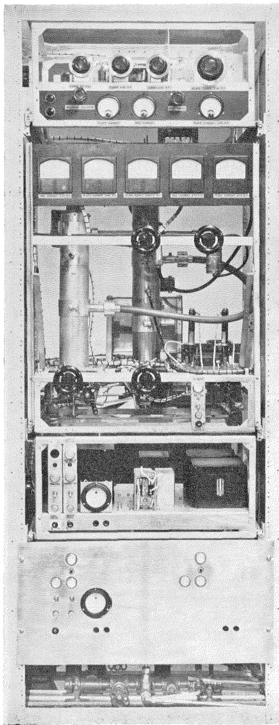
**Fig. 3**—A single cabinet accommodates the 6.805-megacycle crystal oscillator and following stages, which multiply frequency and power to 490 megacycles and 300 watts to drive the penultimate and final stages.
