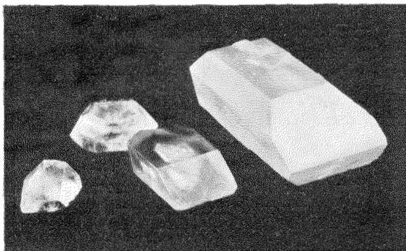
Fig. 5—A large saccharose crystal is at the right and three benzophenone crystals are at the left.
