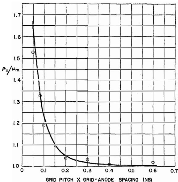
Fig. 10—Variation of amplification factor with grid-anode spacing. The full line represents  $\mu_{11}$  in terms of  $\mu_M$ , where  $\mu_{11}$  is the value given by equation (11), and  $\mu_M$  is Miller's value. The points marked indicate values found experimentally with the rubber sheet.
