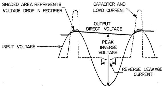
Fig. 4—Voltage and current waveforms obtained with selenium rectifier and capacitive-input filter.
