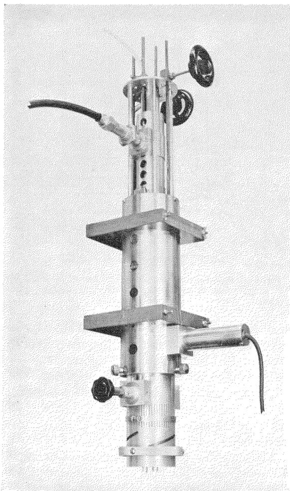
Fig. 5—Coaxial amplifier using 6C22 tube at 490 megacycles.
