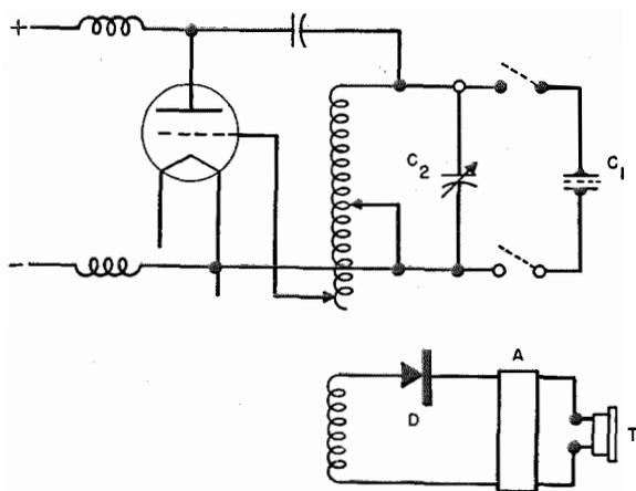
Fig. 1—Circuit for dynamic testing for piezoelectric activity of small irregular particles which are placed between the plates of  $C_1$  and subjected to an electric field which may be varied continuously between frequencies of 1 and 10 megacycles by adjustment of  $C_2$ . Piezoelectric activity produces clicks in the telephone receiver of the detector-amplifier circuit.
