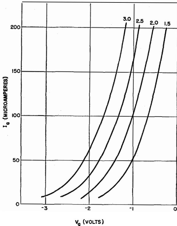
Fig. 8—Anode current-grid voltage for different values of anode voltage  $V_a$  in kilovolts. The following dimensions were employed: Shadow ratio ( $Nd$ )=0.665; grid pitch ( $N$ )=0.73 millimeter, cathode-grid spacing ( $l_c$ )=0.85 and, anode-grid spacing ( $S$ )=0.67.
