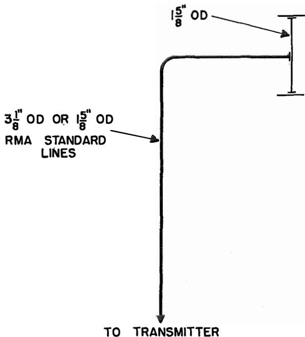
Fig. 8—Coaxial-line feed system for a two-loop array.
