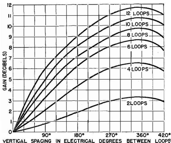
Fig. 7—The power gain of the square-loop antenna can be greatly increased by vertically stacking a number of loops. Note that the highest gain is obtained with one-wavelength spacings between loops.
