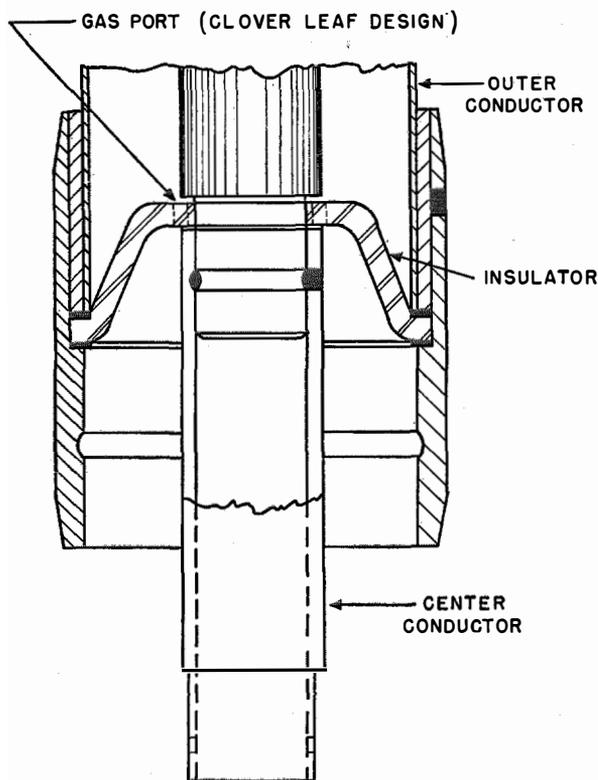
Fig. 15—Cross-sectional view of an anchor insulator which will support the inner conductor of a vertical 100-foot length of coaxial line. This unit is incorporated in a single assembly with a double-bellows expansion joint.
