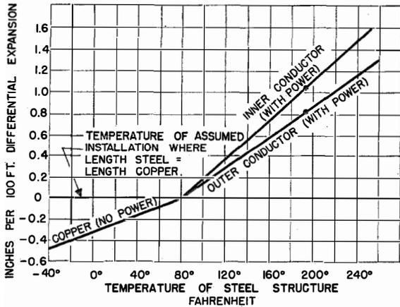
Fig. 17—Expansion of a 100-foot vertical span of coaxial line mounted in a steel tower. The copper and steel have different temperature coefficients of expansion, resulting in a change in the length of the line with respect to the length of the tower with temperature variations. Heating resulting from power transmitted through the line must also be considered. The installation of expansion joints prevents the line from buckling.
