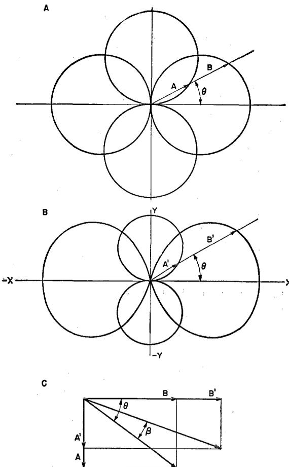
Fig. 10—A perfect set of figure-of-eight patterns are shown in A. In B the patterns are not symmetrical. The vectors in C illustrate the correction  $\beta$  which must be applied to the indicated bearing to obtain the correct bearing.
