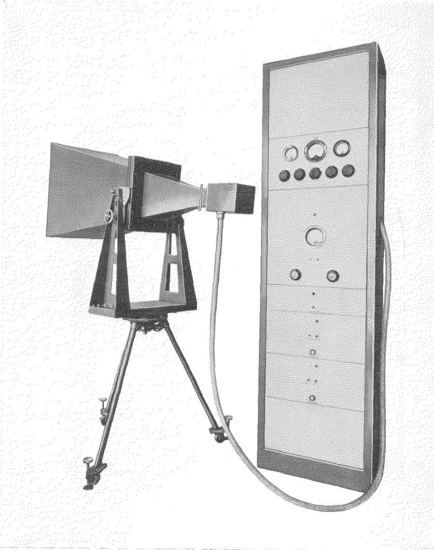
Fig. 12—9-centimeter receiver of the Paris-Montmorency radio link.
