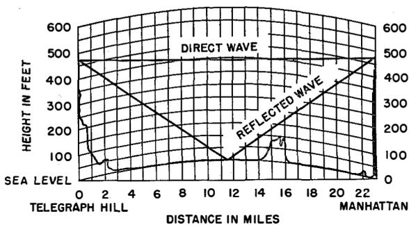
Fig. 3—Topographic paths of the three links in the circuit between the lower tip of Manhattan in New York City and Trenton, New Jersey.
