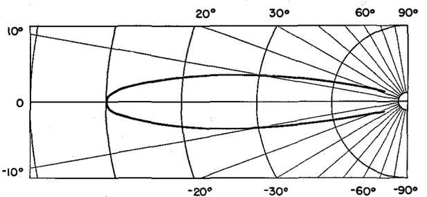
Fig. 3—Vertically polarized radiation from the horn in the horizontal plane. The beam angle is 14 degrees at the 3-decibel points of relative voltage.
