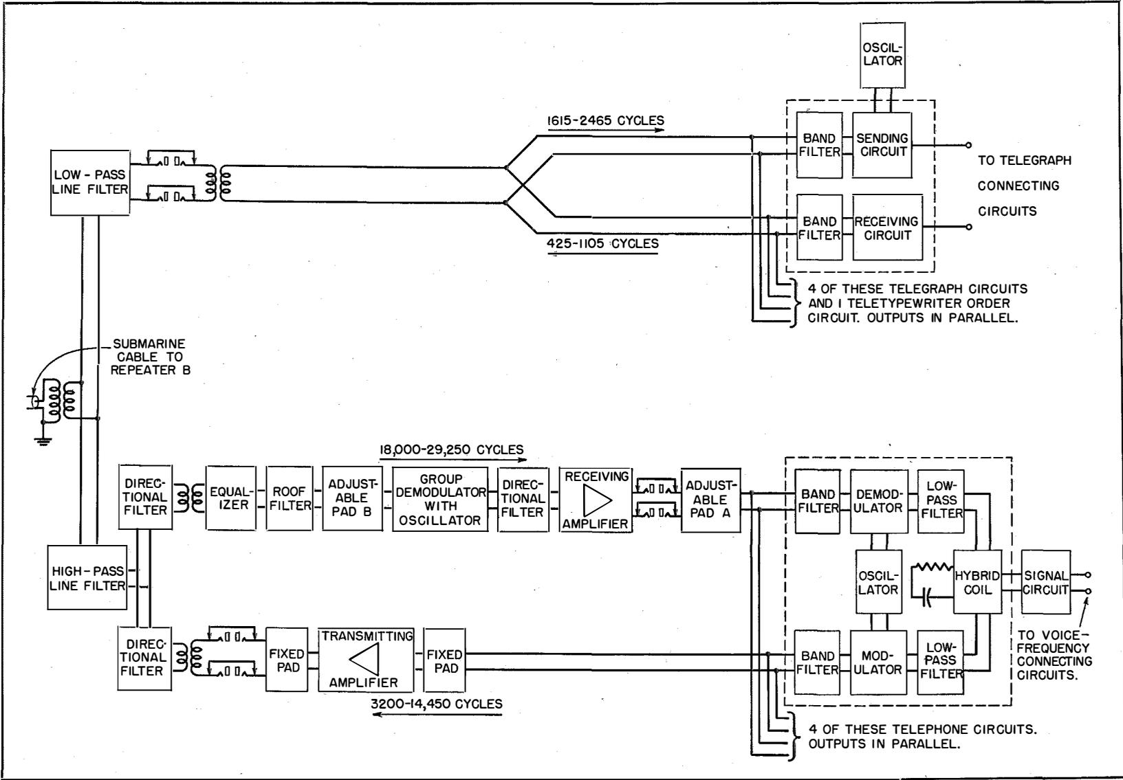
Fig. 4—Schematic arrangement of Terminal C equipment.
