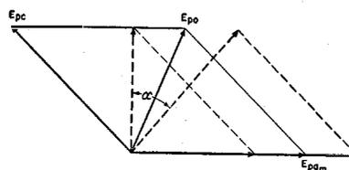
Fig. 5—Vector analysis of the operation of the circuit of Fig. 4.  $E_{pc}$  and  $E_{p0m}$  are the voltages on  $Z_p$  as a result of  $E_r$  being applied through  $C_{gp}$  and through the conductance of the tube, respectively. A voltage  $E_a$  applied to the grid, changes the magnitude of  $E_{p0m}$  without affecting  $E_{pc}$ , producing a phase variation  $\alpha$  in the resultant output radio-frequency voltage  $E_{p0}$ .
