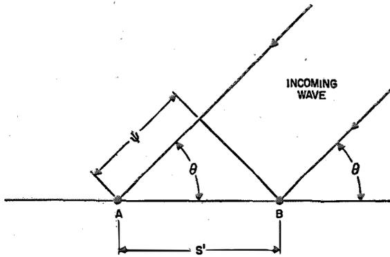
Fig. 2—Factors involved in calculating the receiving pattern of the two-element array (Fig. 1).  $\theta$  = angle of reception to plane of array.  $S'$  = spacing angle =  $360 S/\lambda$ , where  $S$  = actual spacing.  $\psi = S' \cos \theta$ .
