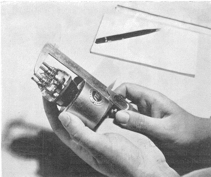
10 kilowatts of output power when driven by a pair of 7C26's.
