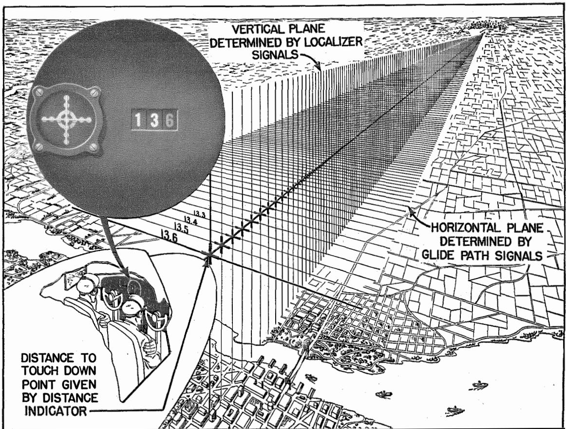
Fig. 10—Instrument landing system principle used in Navaglide.
