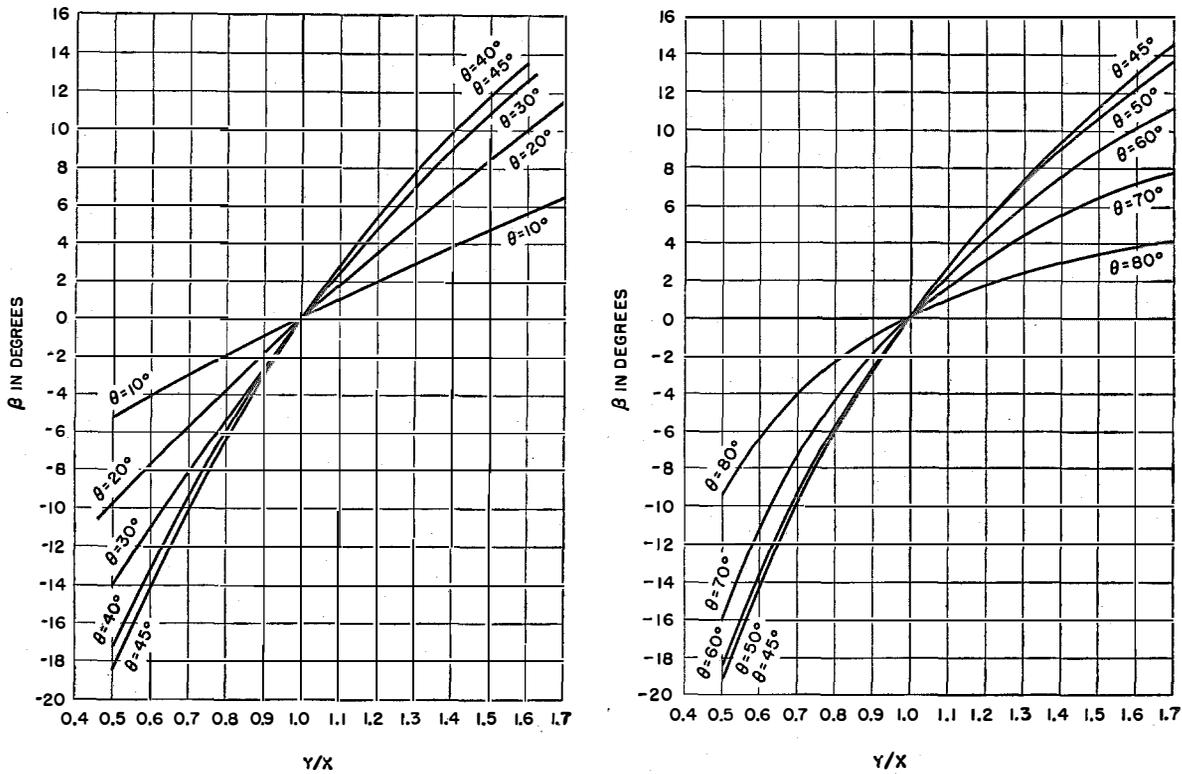
Fig. 11—Correction term  $\beta$  as a function of the angle of reception  $\theta$  for different ratios of relative amplitude between reception from  $X$  and  $Y$  figure-of-eight patterns (Fig. 10B). At the left, for angles up to 45 degrees, the error increases, after which it again decreases as at the right.
