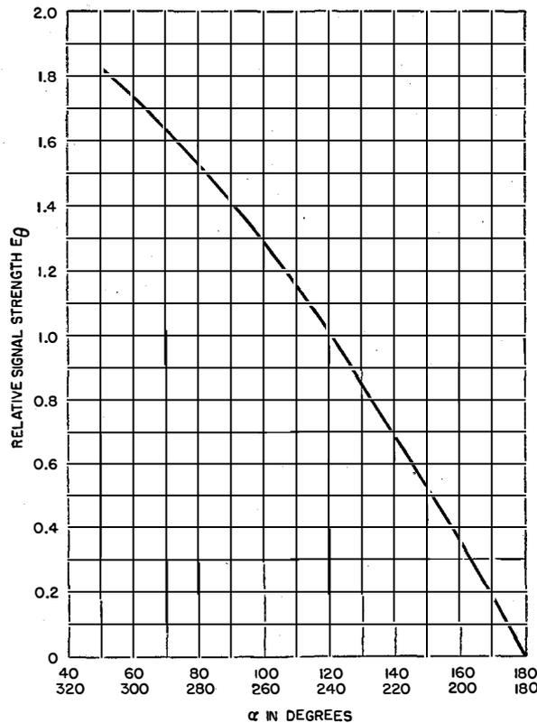
Fig. 5—Variation of  $E_\theta$  with  $\alpha$  for  $k=1$ .
