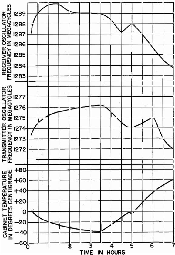
Fig. 8—Frequency variation of transmitting and receiving oscillators during 7 hours in which the temperature was changed from 0 to -38 to +60 degrees centigrade.
