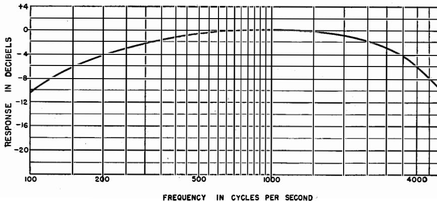
Fig. 2—Response-frequency characteristic of the mobile equipment. Reference level is the response at 1000 cycles.
