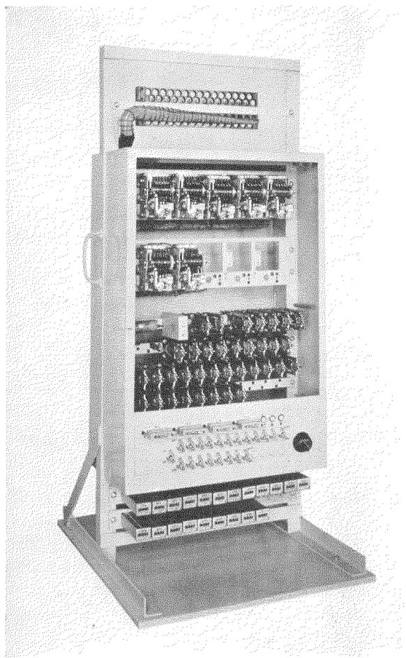
subgroups. The number of paths in the groups being observed need not be in multiples of 10. If some of the arc contacts of the selector switches are not connected to circuit paths, tests in these positions will of course never cause an operation of the message register, and the traffic recorded will be that on the paths connected through terminals of the recorder to the selector arcs.
