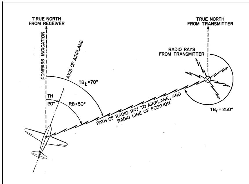
Fig. 2—Principle of airborne direction finding.
