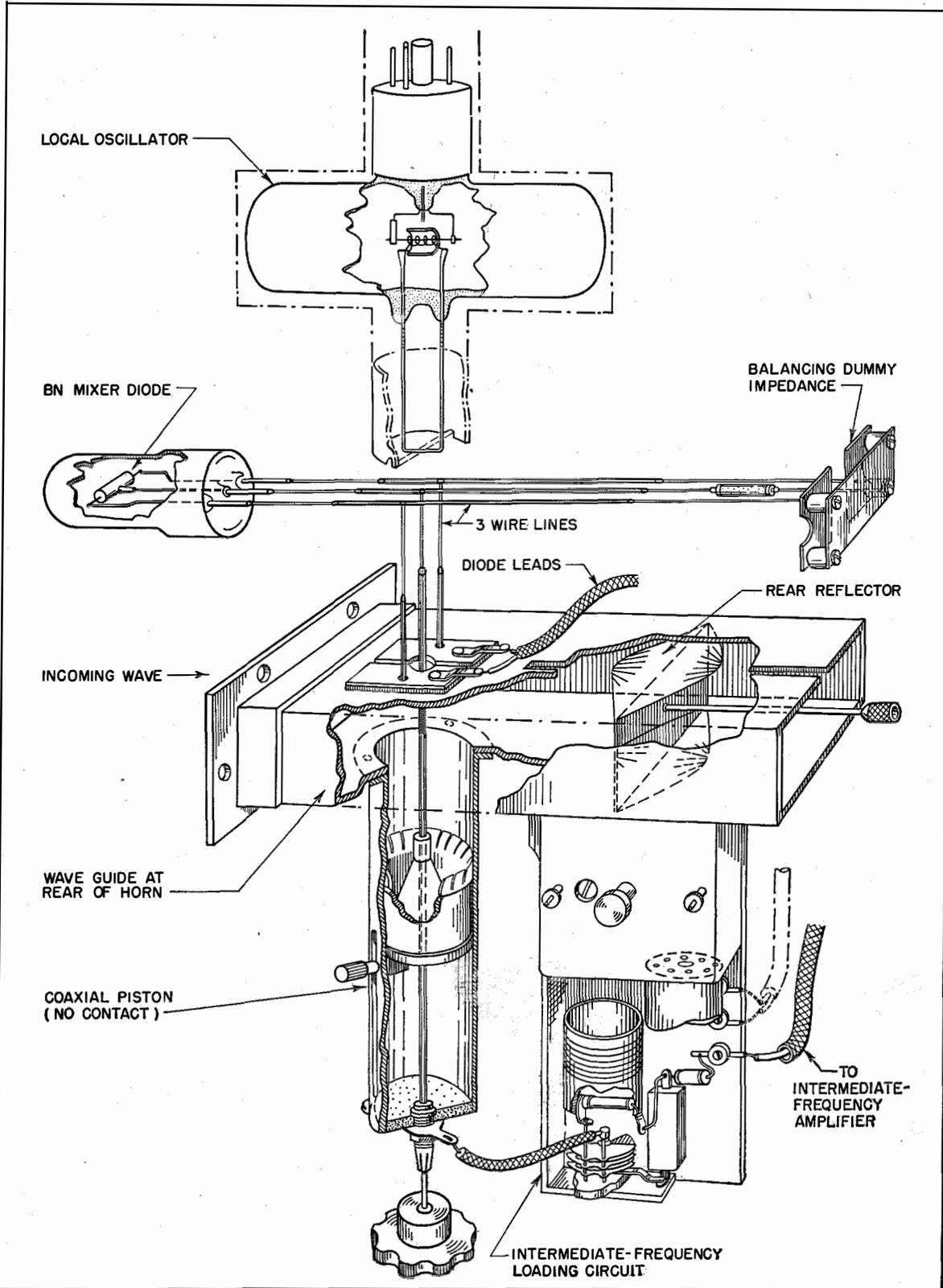
Fig. 14—Balanced mixer used in receiver. This entire equipment is mounted in the box at the rear of the horn as shown in Fig. 12.
