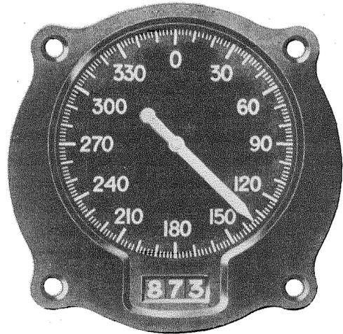
Simple meter type of presentation for an R $\theta$  radio navigational system. Distance in miles and tenths is shown by the number-wheel type of indicator; bearing or azimuth is shown in degrees by the pointer. As distance and bearing are indicated simultaneously from the same radio landmark, complete information for a position fix is constantly presented in direct terms.
