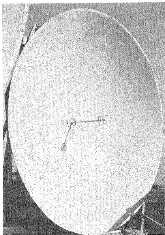
Fig. 14—Typical dipole and parabolic reflector for use in the 1000- to 3000-megacycle region. The enclosure around the dipole protects it from rain, snow, and sleet.
