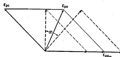
Fig. 5—Vector analysis of the operation of the circuit of Fig. 4.  $E_{pc}$  and  $E_{p0m}$  are the voltages on  $Z_p$  as a result of  $E_r$  being applied through  $C_{gp}$  and through the conductance of the tube, respectively. A voltage  $E_a$  applied to the grid, changes the magnitude of  $E_{p0m}$  without affecting  $E_{pc}$ , producing a phase variation  $\alpha$  in the resultant output radio-frequency voltage  $E_{p0}$ .
