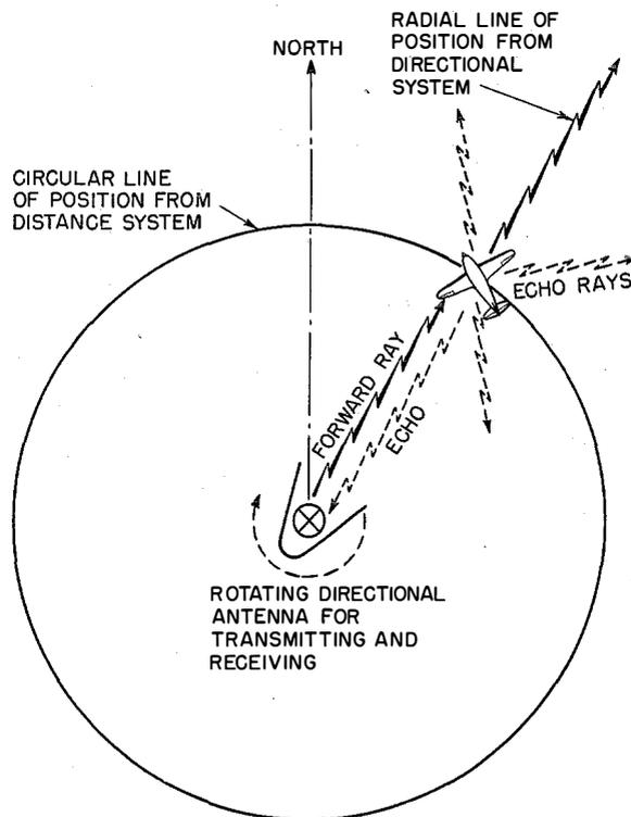
Fig. 6—Radar principle using plan-position type of indication.
