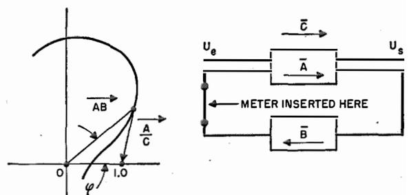
Fig. 9—Simplified method of obtaining data for plotting Nyquist diagrams. Only measurements of gain are required.
