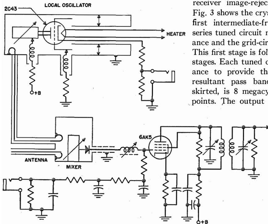
Fig. 3—Input end of the receiver showing local oscillator, input tuning, mixer, and first stage of intermediate-frequency preamplifier.
