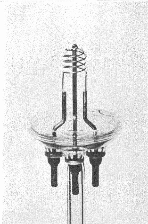
Fig. 4—Filament mounted on molded glass flare.
