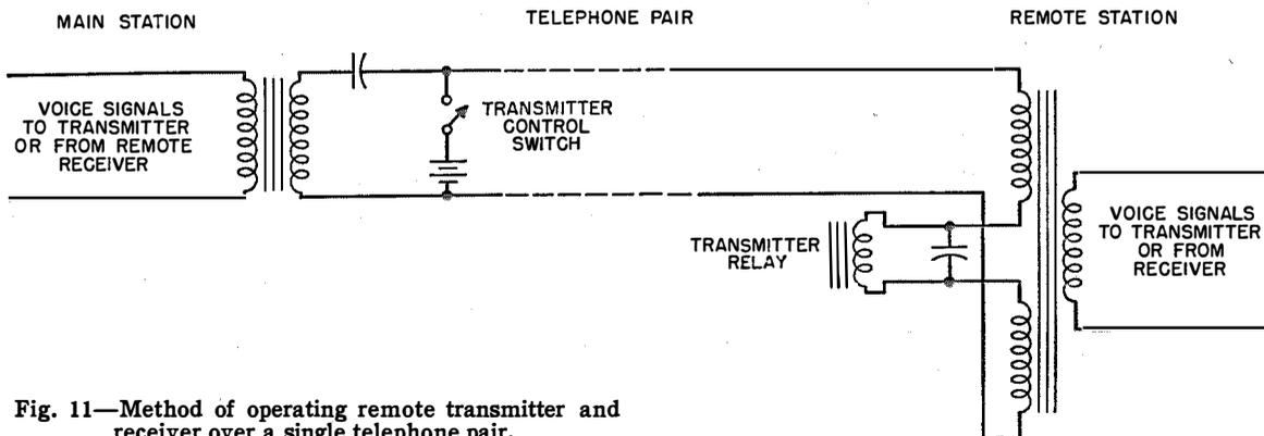
Fig. 11—Method of operating remote transmitter and receiver over a single telephone pair.
