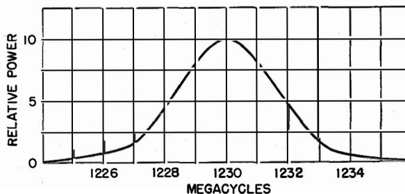
Fig. 9—Frequency spectrum of transmitter during pulse modulation.
