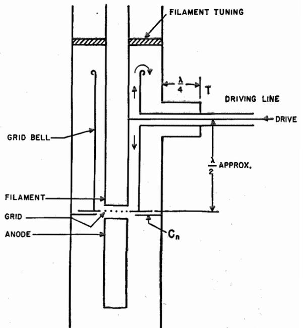
Fig. 12—Neutralization arrangement.
