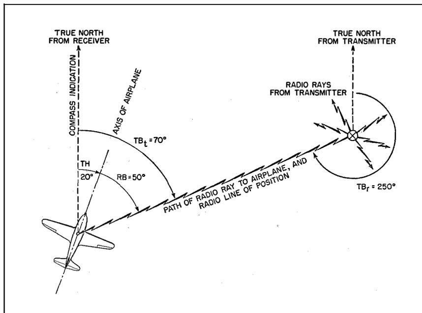
Fig. 2—Principle of airborne direction finding.
