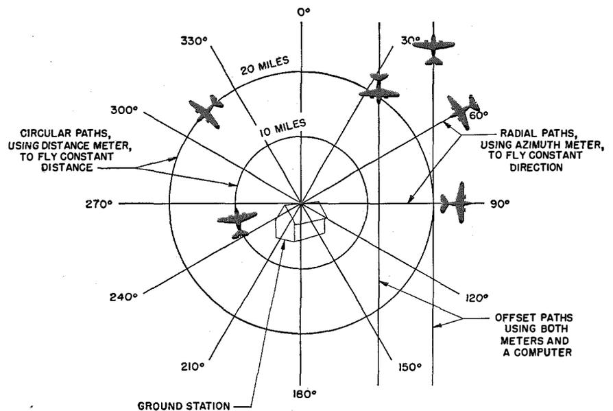
Fig. 11—Useful types of flight paths possible in an Rθ or distance-bearing radio navigational system. Tracks may be accurately followed by reference to a distance-azimuth meter like that shown in a previous illustration.
