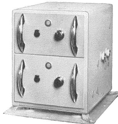
microphone hook, and whip antenna. Both the receiver and transmitter are on separate plug-in chassis, which are inserted in either a vertical or horizontal housing. The control box is normally mounted on the instrument panel of the automobile.
