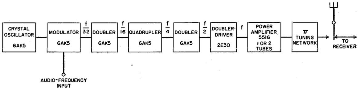
frequency multipliers which operate as saturated class-C amplifiers. The output of the power amplifier stage, also operating class C, is coupled to the antenna through a tuned  $\pi$  network. The transmitter may be operated at any frequency between 30 and 44 megacycles by inserting a crystal of the proper frequency and adjusting the tuned circuits.
