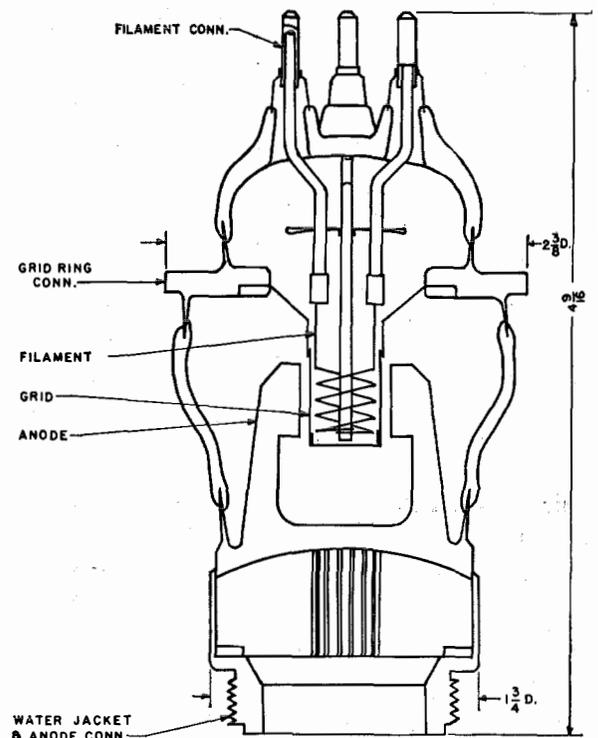
Fig. 2—Cross-sectional view of 6C22.
