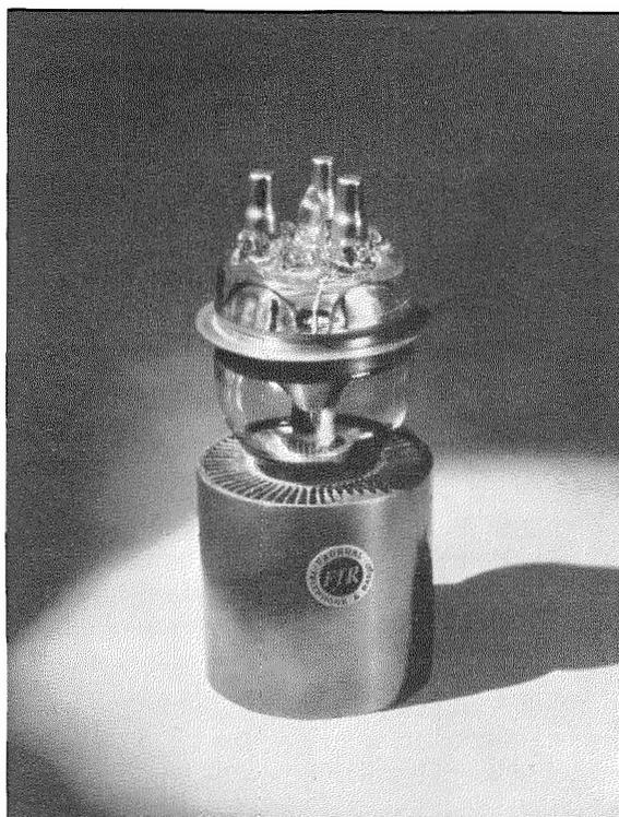
**Fig. 4—7C27 air-cooled triode capable of giving 5 kilowatts of power at 110 megacycles.**
