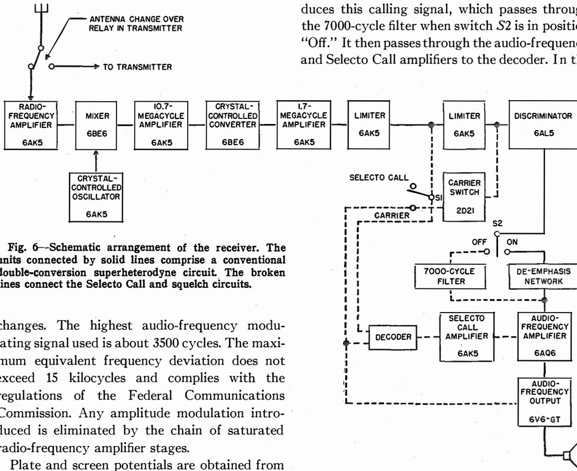
Fig. 6—Schematic arrangement of the receiver. The units connected by solid lines comprise a conventional double-conversion superheterodyne circuit. The broken lines connect the Selecto Call and squelch circuits.
