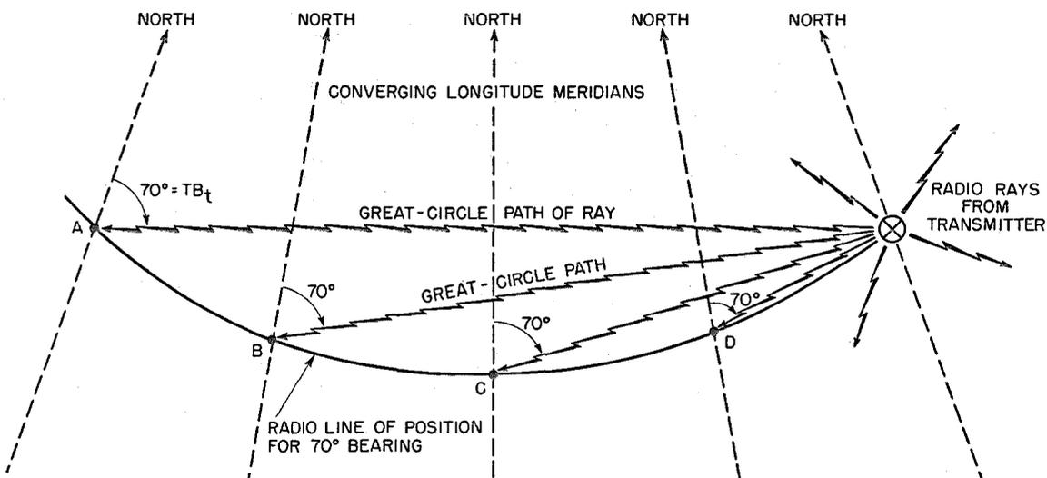
Fig. 3—Direction-finding complications at long distances.  $TB_r = TB_i + 180$  degrees + meridian convergence correction.
