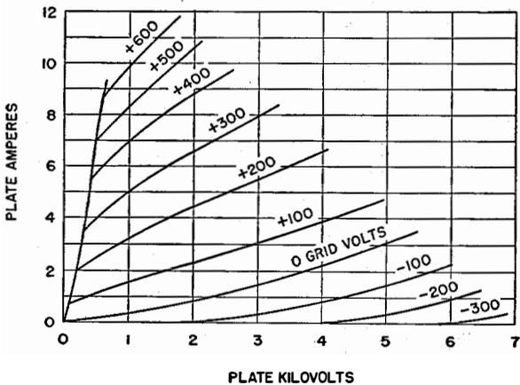
Fig. 3—Average plate characteristics of the 7C26.
