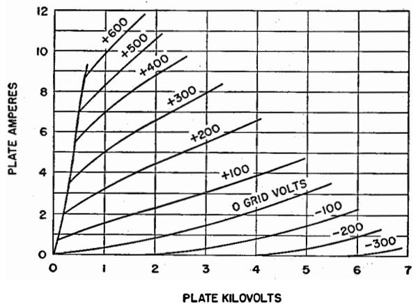
Fig. 3—Average plate characteristics of the 7C26.
