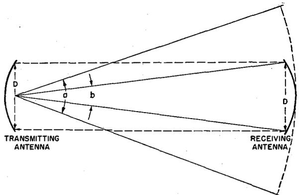
Fig. 1—Free-space attenuation is a function of the beam characteristics of the antennas. The angle in which the radiation is concentrated when using dipole radiators and parabolic reflectors is  $a = 1.7 (\lambda/D)$ . The angle in which the receiving antenna is viewed from the transmitting point is  $b = D/L$ , where  $L$  is the distance between transmitting and receiving antennas.
