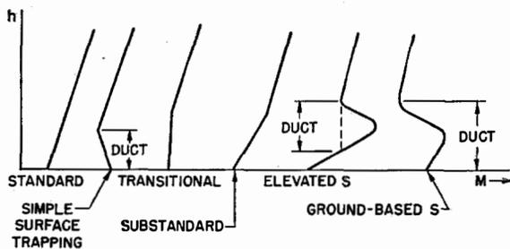
Fig. 2.—Variations of refractive index of the atmosphere  $M$  with height  $h$ . The regions marked "duct" are capable of propagating waves over very long distances with little attenuation.
