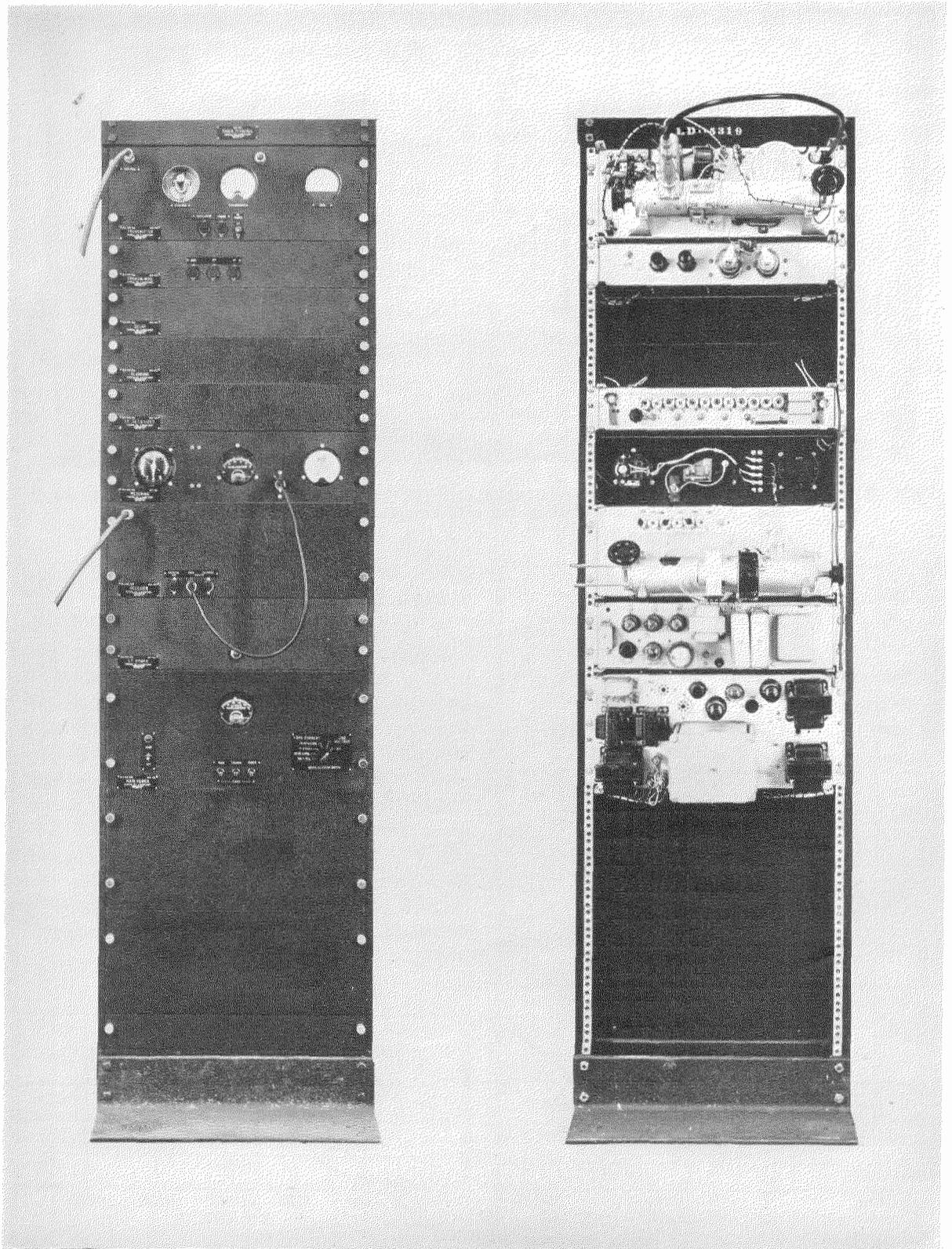
**Figs. 10 and 11—Front and rear views of radio repeater rack in which both the receiver and transmitter assemblies are mounted.**
