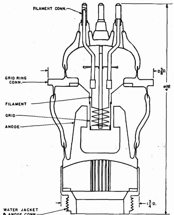
Fig. 2—Cross-sectional view of 6C22.
