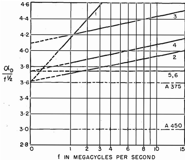
Figure 1— $\alpha_D/f^{1/2}$  plotted against  $f^{1/2}$  for the corresponding indicated values of frequency in megacycles per second for coaxial pairs at 10 degrees centigrade (50 degrees Fahrenheit). The constant  $K_1$  is obtained by extrapolating the curves to  $f^{1/2}=0$ . The upper 5 curves are for cables listed in Table 1. The curves A375 and A450 are for ideal coaxial pairs of 0.375 and 0.450 inch (9.5 and 11.4 millimetres) respectively.
