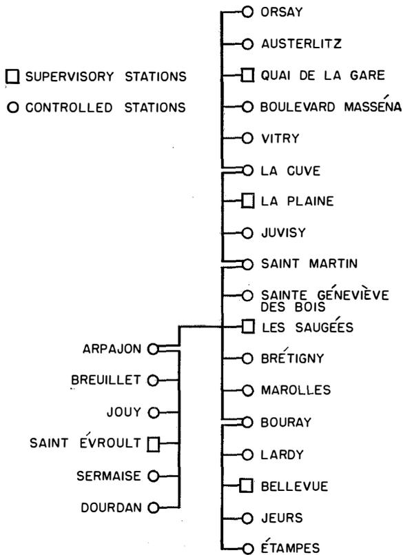
Figure 1—Arrangement of control and controlled stations in the Paris-Orleans railway system.
