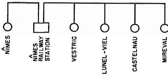
Figure 3—The Nîmes-Sète railway is operated from 5 substations that are controlled from the Nîmes railway station.
