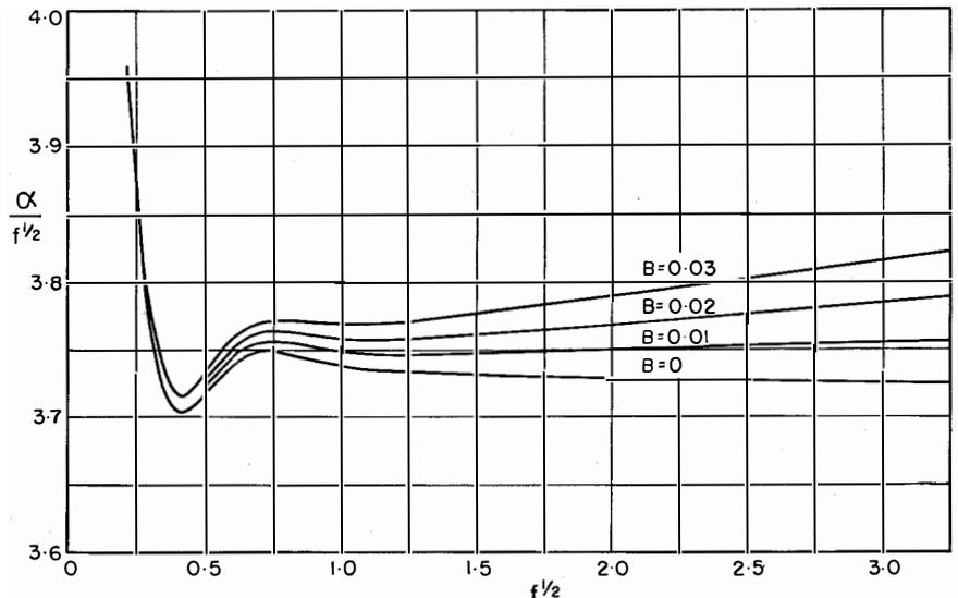
Figure 19—Here,  $\alpha/f^{1/2}$  is plotted against  $f^{1/2}$  for 0.375-inch (9.5-millimetre) coaxial pair having an outer conductor of 0.010-inch (0.25-millimetre) thickness.
