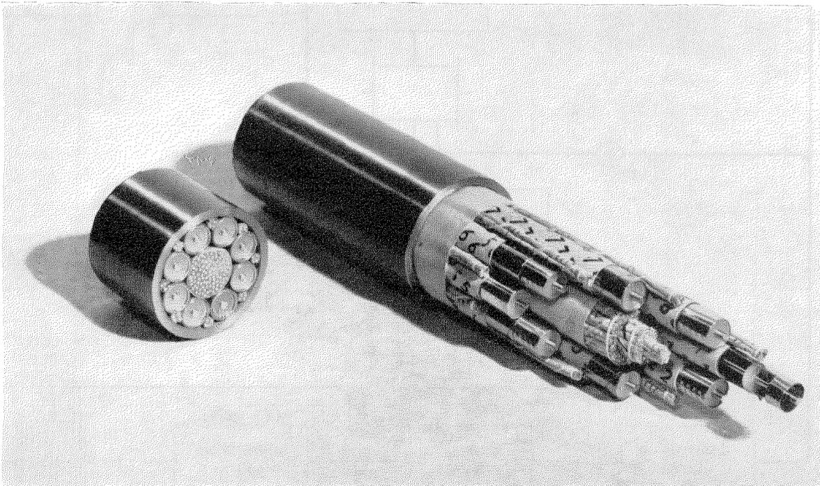
Figure 4—In this cable the 8 coaxial pairs surround 24 paper-insulated quads and there are 8 more quads in the outermost interstices.
