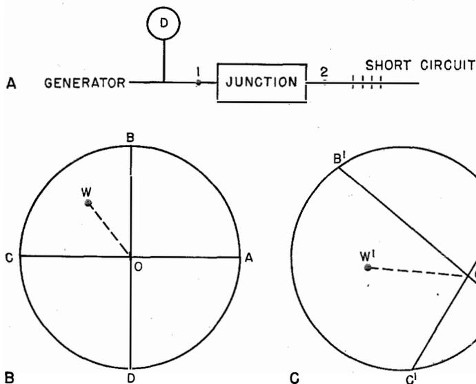
Figure 8—Reflectance measurement through a lossless junction.
