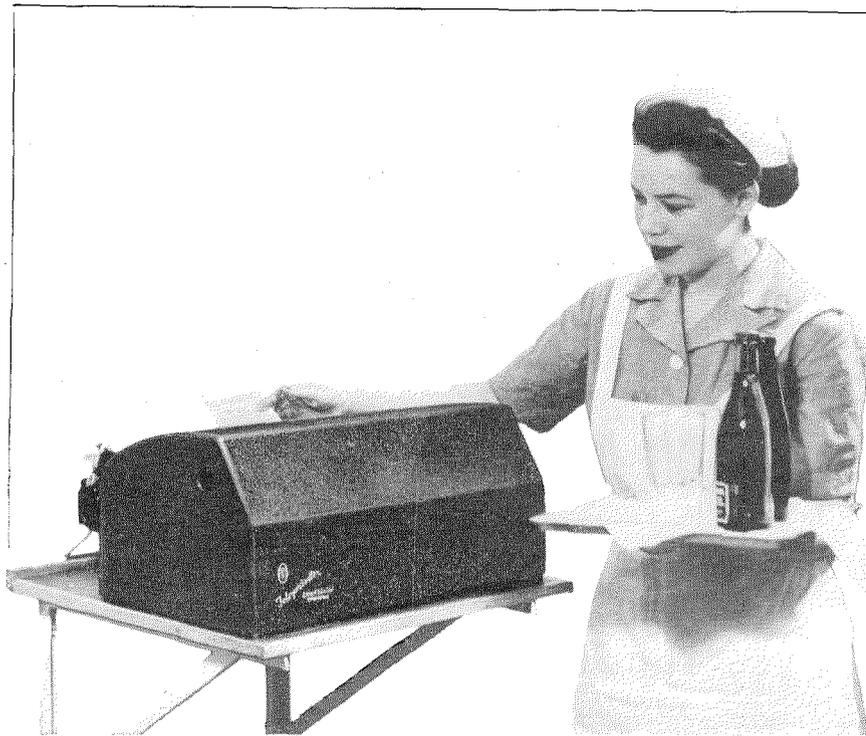
Figure 4—A waitress removes an order from the receiving teleprinter at one of the room-service stations on an upper floor.
