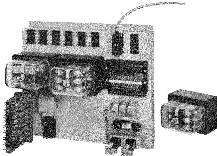
At left is shown the apparatus frame that is mounted in the rear of the control desk and contains the sockets for the plug-ended connections from the sender switches. This rack accommodates the relay apparatus necessary for operation of the system. All relays are housed in special plug-in mountings fitted with glass covers to render the apparatus dustproof.
