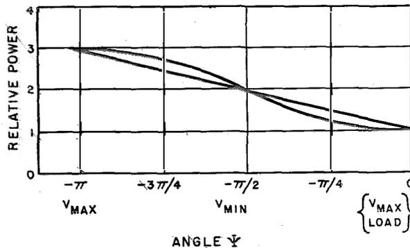
Figure 4—Power flow along line. Straight line is computed power neglecting  $B_0/G_0$  term in (12). Curved line is according to complete formula for case of negligible dielectric loss.
