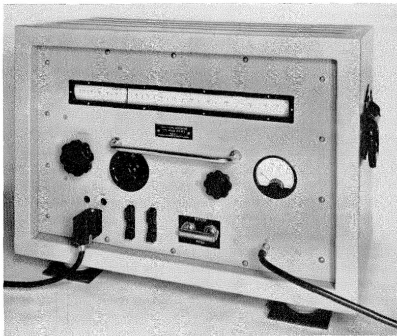
Figure 16—Signal generator of high output power for making attenuation and crosstalk tests in the field.
