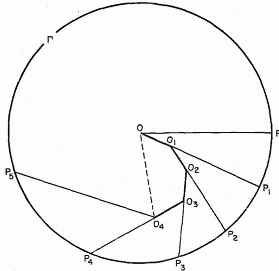
Figure 7—Transformation of reflectance through a stratified medium.
