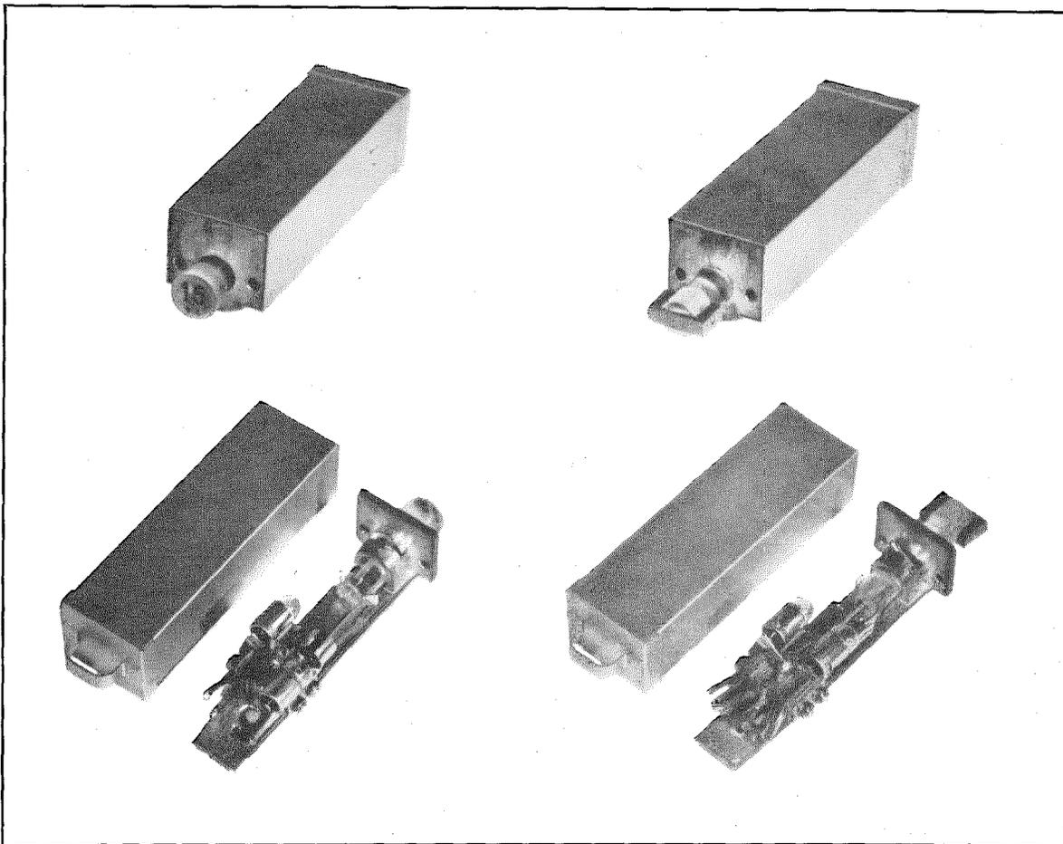
Figure 16—The smaller switch is at the right and a light indicator for signalling only is at the left. These are used in the Lyons control room.
