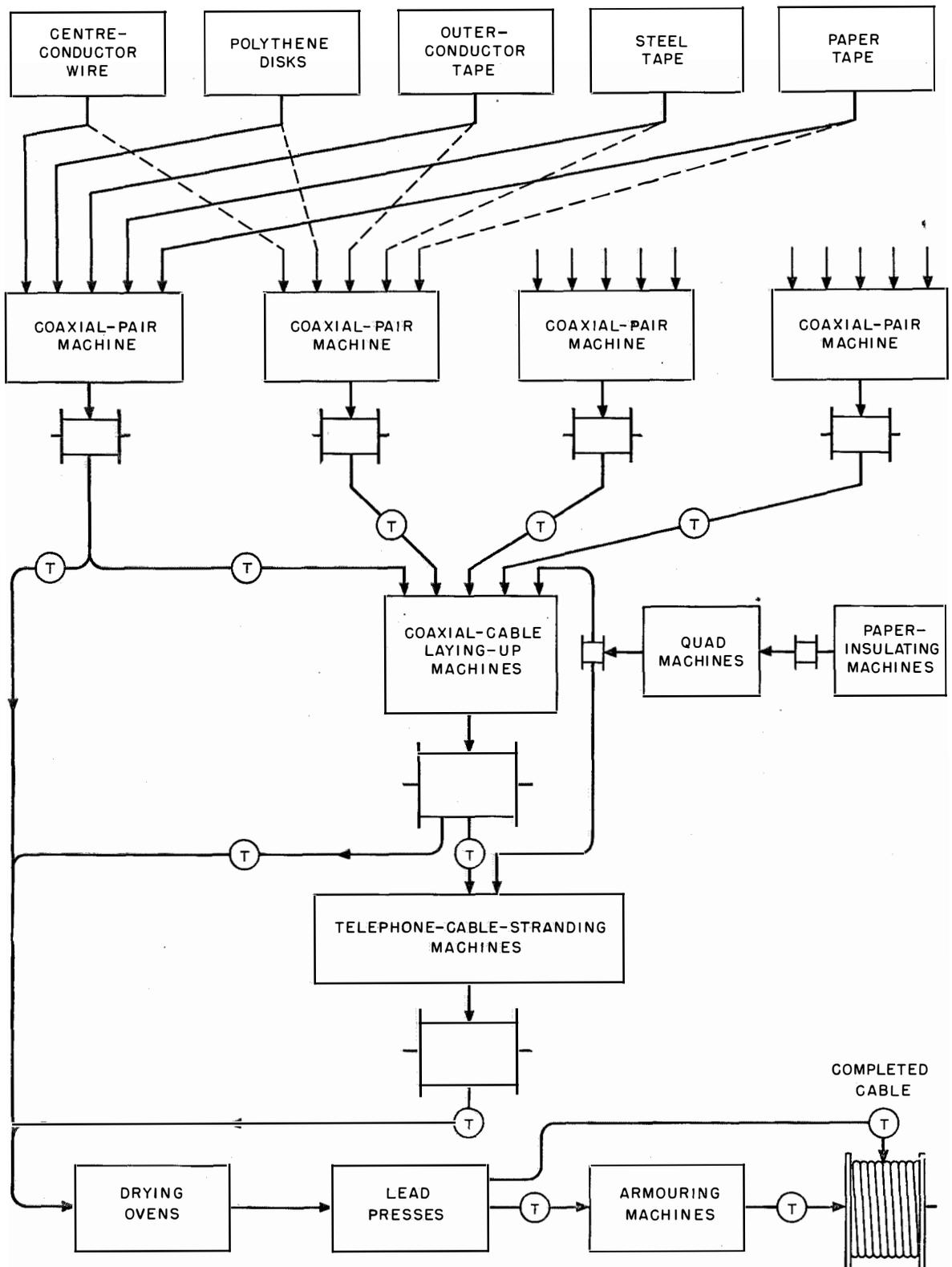
Figure 5—Manufacturing operations required for producing various sizes of composite cables including design-6 coaxial pairs.
