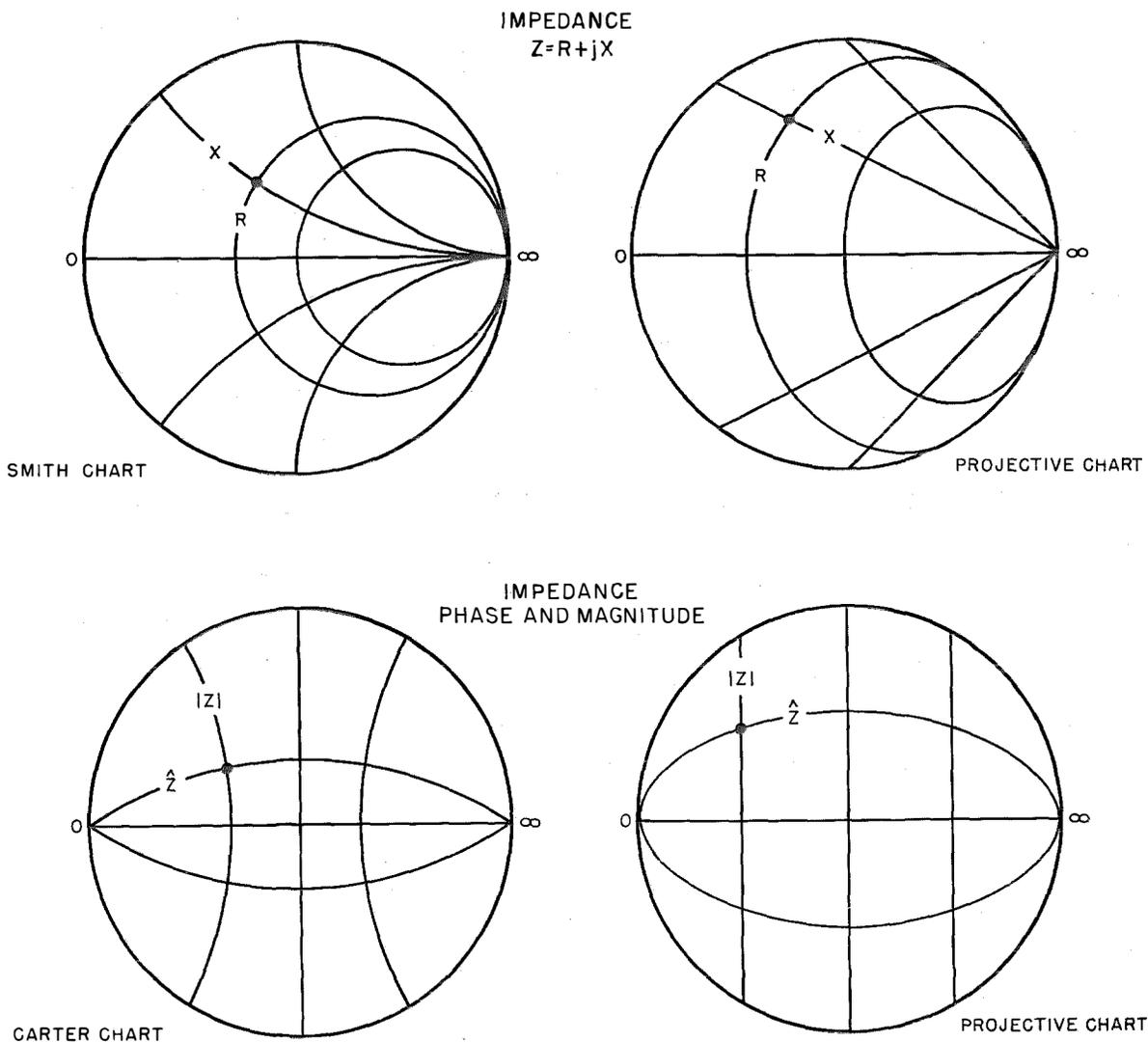
Figure 3—Loci on the projective chart and on the Smith and Carter charts of constant resistance  $R$ , reactance  $X$ , impedance magnitude  $|Z|$ , and impedance phase  $\hat{Z}$ .
