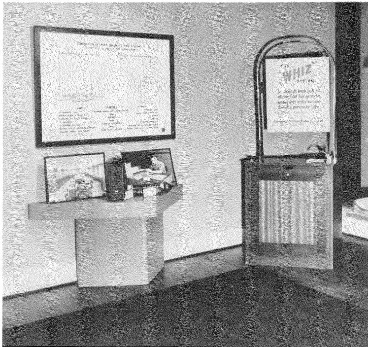
At the left are examples of a pneumatic-tube system that automatically routes each carrier to its indicated destination and of the "Whiz" carrierless ticket transporting system developed by Mix and Genest in Germany. Several installations have been made in the United States.
