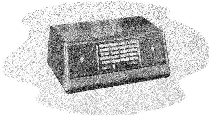
The Select-O-Phone executive station (left) is a new device developed by Kellogg Switchboard and Supply Company. Entirely separate from the regular public telephone system, as many as 55 extensions may be called by push-button individually or in conference groups. At the right below is the cabinet housing the automatic switching equipment for the system.
