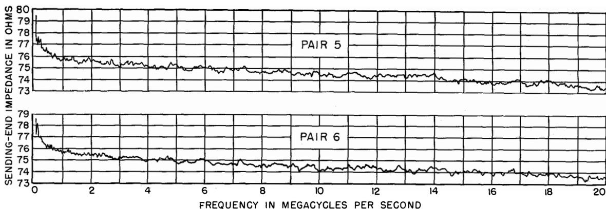
Figure 21—Impedance plotted against frequency for a 6-mile (9.7 kilometre) repeater section of a 6-pair coaxial cable.
