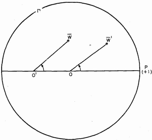
Figure 6—Change of reference level—ideal transformer.
