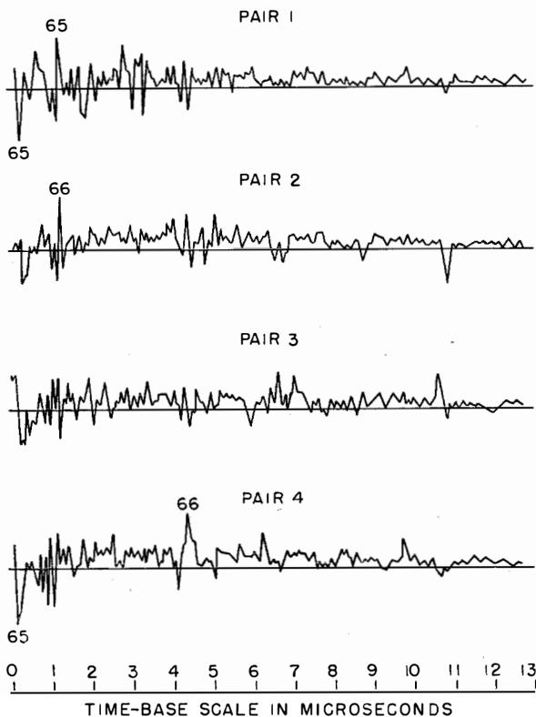
Figure 14—Pulse-echo test oscillograms from a 2000-yard (1829-metre) length of coaxial cable installed in 1951. A direct-current pulse of 0.1-microsecond width was used and the magnitudes of the strongest reflections are indicated in decibels below the incident pulse level.
