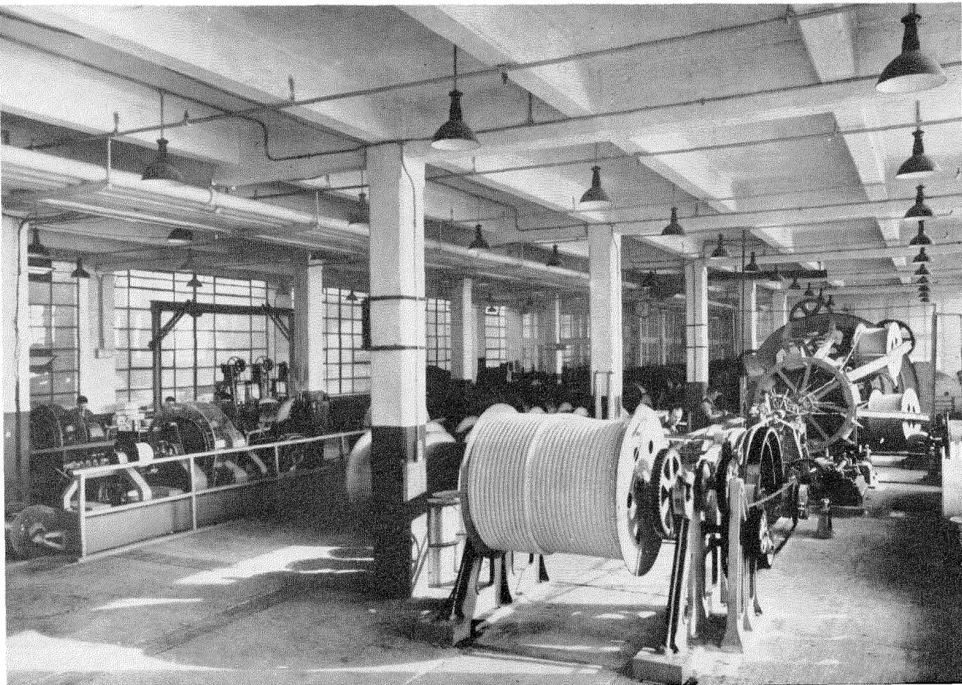
the larger guard housing the paper-tape head. From this, the completed coaxial pair passes round a capstan and through an automatic flaking device on the take-up cylinder, which is visible in the top left of the picture.
