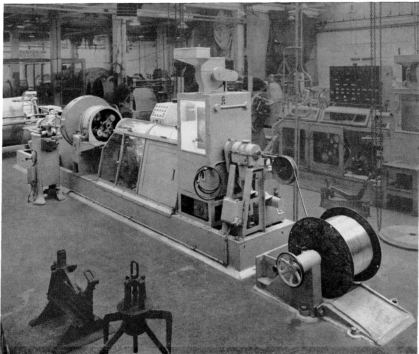
position on its stand. The wire is taken up to the main longitudinal axis of the machine, passes through a cleaning device, and enters the rectangular cabinet containing the polythene-disk applicator head.<sup>10</sup> Except for minor changes, the disks are applied to the centre conductor in the manner outlined in Section 2.5. Part of the applicator wheel may be seen through the perspex panel of the cabinet.
