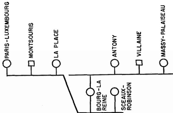
Figure 2—Two control stations at Montsouris and Villaine supervise the Sceaux and Massy-Palaiseau lines of the Paris Metropolitan Railroad.
