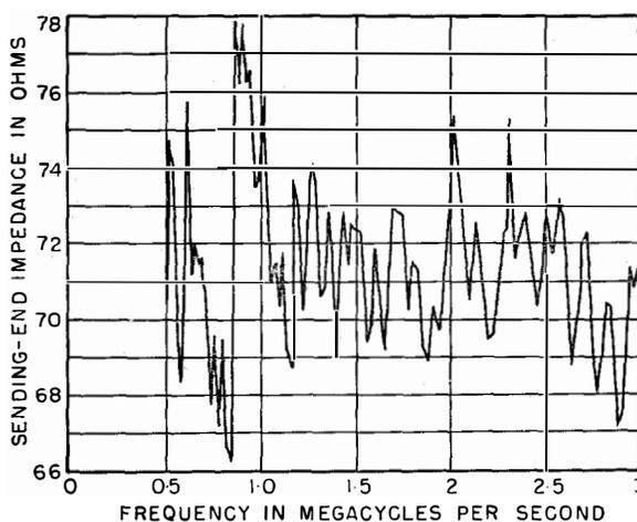
Figure 22—Impedance curve for repeater section of design 2 installed in 1937.
