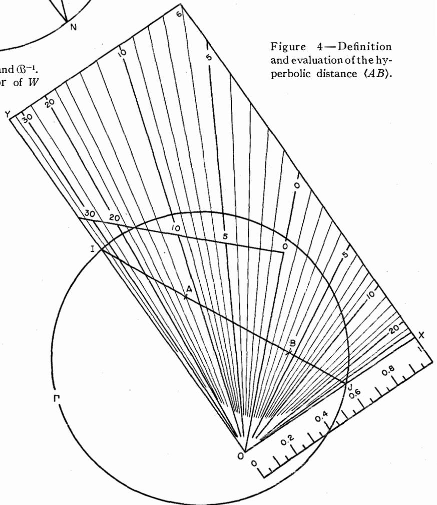
Figure 4—Definition and evaluation of the hyperbolic distance  $(AB)$ .
