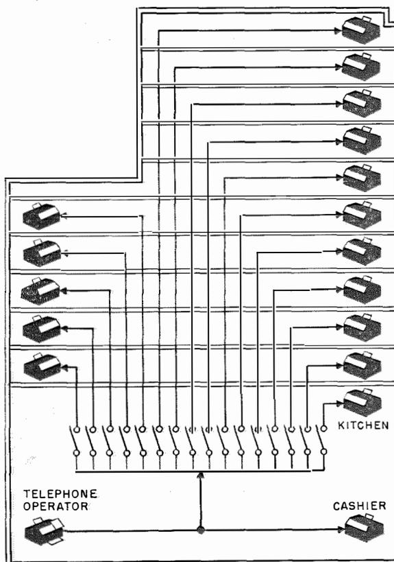
Figure 2—The system incorporates a sending-receiving teleprinter in the telephone exchange and 17 receivers located on various floors of the building.
