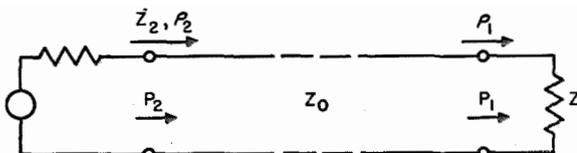
Figure 1—Transmission line of length  $h$ .
