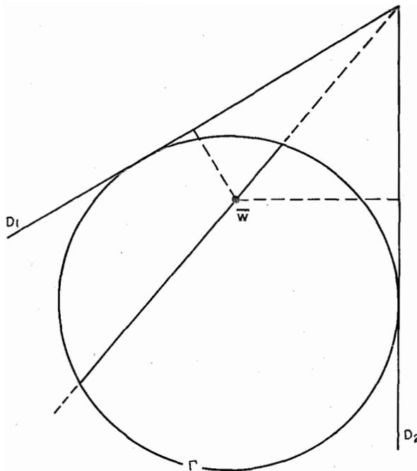
Figure 11—Locus of  $W$  for a given ratio of powers picked up by two probes in a slotted line.
