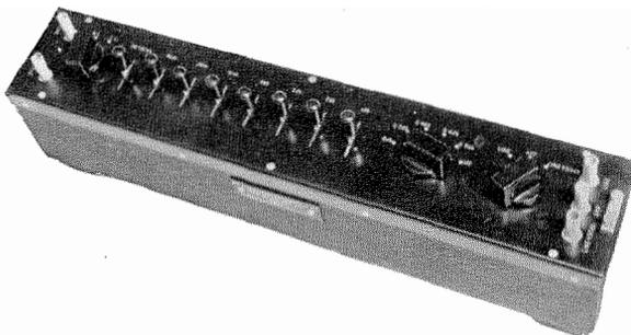
Figure 17—Attenuator used for crosstalk and attenuation measurements in the field.
