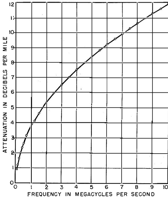
Figure 18—Attenuation as a function of frequency for a 6-pair coaxial cable installed in 1951. The measurements were made on a 6-mile (9.7-kilometre) repeater section and corrected to a temperature of 10 degrees centigrade (50 degrees Fahrenheit).
