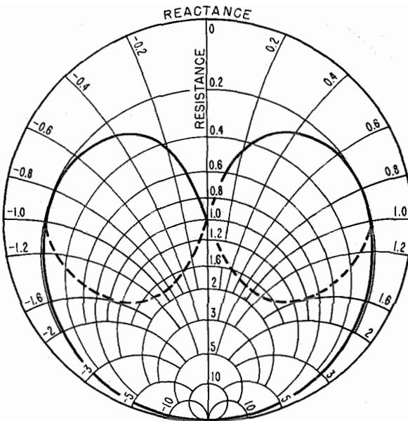
Figure 2—Permitted region for use of formula  $S = (1 + x^2)/r$ . Area outside solid heart-shaped curve drawn on Smith chart is where formula is accurate to within one percent. Area outside dashed curve is where reciprocal of  $r + jx$  lies in permitted region; see Section 6.1
