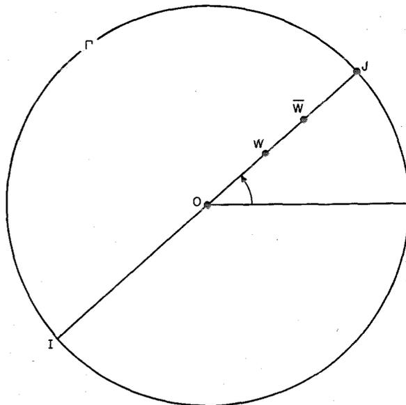
Figure 1—Relation between the representations of a reflection coefficient (or a polarization ratio) on the Smith chart ( $W$ ) and on the projective chart ( $\bar{W}$ ).
