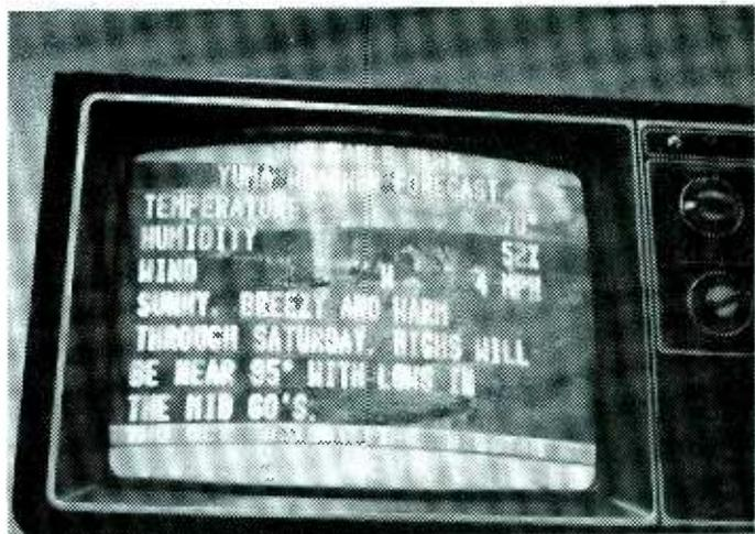
Pictured above is a scenery slide reproduced with a flying spot scanner with character generator words over. Bottom stripe is left to right crawling words advertising a pay movie channel. Small next stripe up is continuous time and date.
