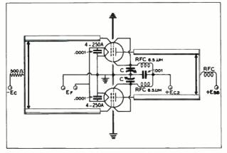
Screen-tuning neutralization circuit for use above 45 Mc. C --- Approximately 100μμfd. per section, maximum. entering the amplifier in order to minimize grid-plate coupling between these leads external to the amplifier.
