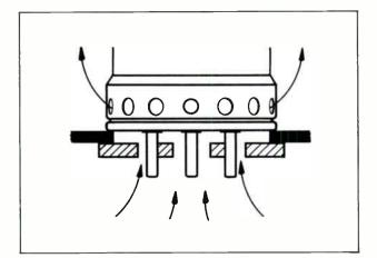
4-125A mounting providing base cooling, shielding and isolation of output and input compartments.
