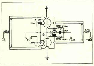
Screen-tuning neutralization circuit for use above 45 Mc. C — Approximately  $100\mu\mu$ fd. per section, maximum.
