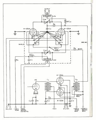
Typical high-level-modulated r-f amplifier circuit, with modulater and driver stages, 750 watts plate input.
