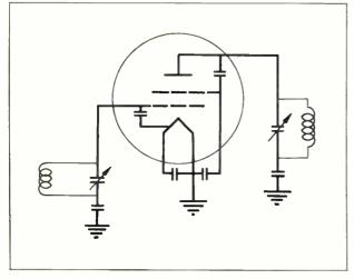
Fig. 23 Usual circuit supporting VHF parasitic oscillation in HF r-f amplifiers.
