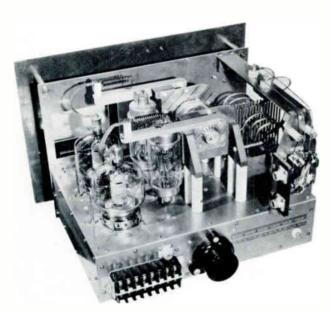
Fig. 2 Push-pull r-f amplifier employing 4-250A tetrodes. Designed and built by C. F. Bane (W6WB)<sup>3</sup>.
