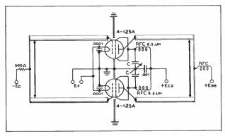
Screen-tuning neutralization circuit for use above 100 Mc. C is a small split-stator capacitor.  $C(\mu\mu fd) = \frac{640,000}{f^{t} (Mc.)}, \text{ approx.}$
