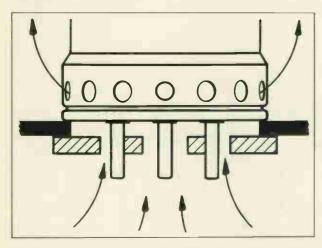
4-250A mounting providing base cooling, shielding and isolation of output and input compartments.
