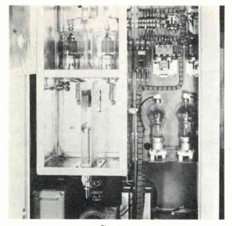
Fig. 4 Push-pull 110 Mc. amplifier employing 4-1000A tetrodes, Gates Radio Co. Model BF 3 kw trasmitter.
