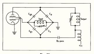
Fig. 28 Single-ended plate neutralization showing capacitance bridge circuit present.
