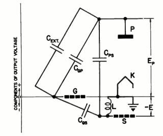
Fig. 31 Components of output voltage of a tetrode when neutralized by added series screen-lead capacitance.
