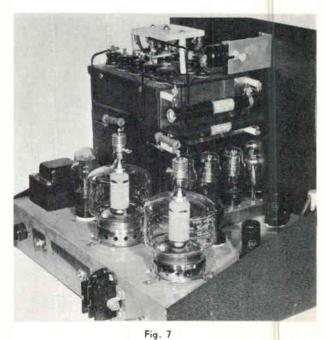
Experimental 500 watt Class-AB, audio amplifier. Designed and built by Eitel-McCullough Laboratories'.
