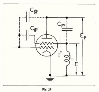
Tetrode characteristics involved in feedback circuit.
