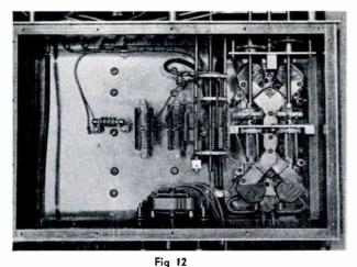
Fig #2 Underside of push-pull multi-band r-f amplifier employing 4-250A tetrodes. Designed and built by C. F. Bane (W6WB)<sup>3</sup>.
