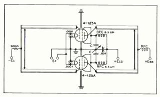
Screen-tuning neutralization circuit for use above 100 Mc. C is a small split-stator capacitor.  $C(\mu\mu fd) = \frac{640,000}{f^{r} \text{ (Mc.)}}, \text{ approx.}$
