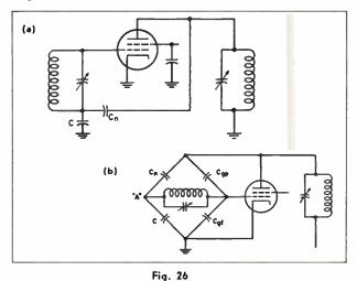
Single-ended grid neutralization described by Bruene<sup>®</sup>. a) Basic Circuit. b) Arranged as capacitance bridge.
