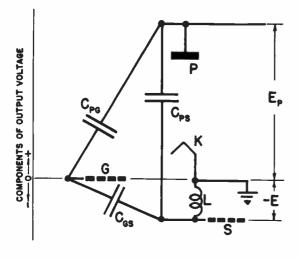
Fig. 30 Graphical presentation of components of output circuit voltages in tetrode when self neutralized.
