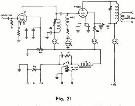
Tetrode amplifier keying circuit used by B. O. Ballou (W6BET)".
