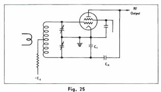
Push-pull grid neutralization, basic circuit.
