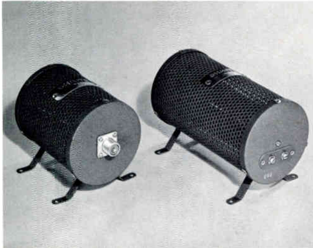
Fig. 44: Dummy antennas with coax and terminal strip connections.
