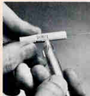
Fig. 9: Markings are integral with coatings — are unaffected by abrasion with glass fiber brush.
