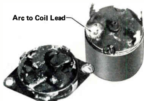
MIL-R-5757 Design After Being Used to Switch 115/200 Volts 3Ø (On-Off Control) for which Service It was Neither Designed nor Tested.
