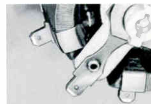
Fig. 65: Typical rheostat with terminals for push-on connection
