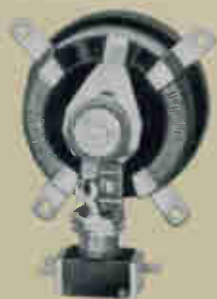
Fig. 80: A reversing-type, speed control rheostat
