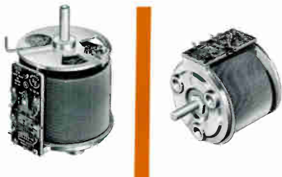
Fig. 4: On VT4, VT8 and VT20 types, shaft can be moved from brush side (left) to base side (right). Socket head screws (left) in radiator hub of VT4 and VT8 hold shaft. (See Fig. 33 for VT20 shaft lock.)
