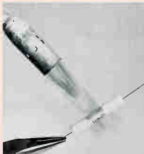
Fig. 7: 1500°F — Red Heat! Series 99 resistors show no deformation; vitreous markings remain legible.
