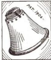
(Outside Thread Measurement of Mouth Piece 15-16" dia. x 30 Thread)
