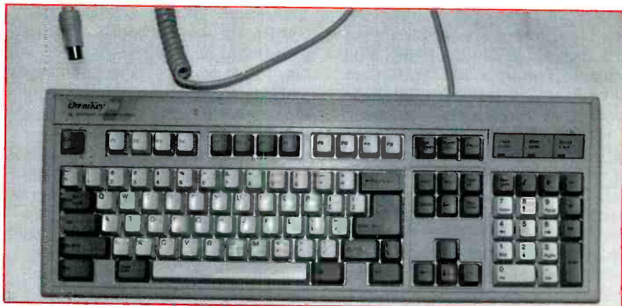
Another necessity is an AT-compatible keyboard, like the Northgate OmniKey model shown here.
