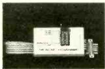
of your PC instead of an internal card. The software has 24 functions and programs 27/28/25/68764, Cmos, EEproms & Flash from 16K - 4Meg (2K-256K x 8) with a 32 pin socket. Adapters available for 874X MCU's, 40-Pin Eproms, 5-Gang, 16 Pin X4 & X8 Prom, Serial Eproms and Eprom Emulator to 32K x 8.
