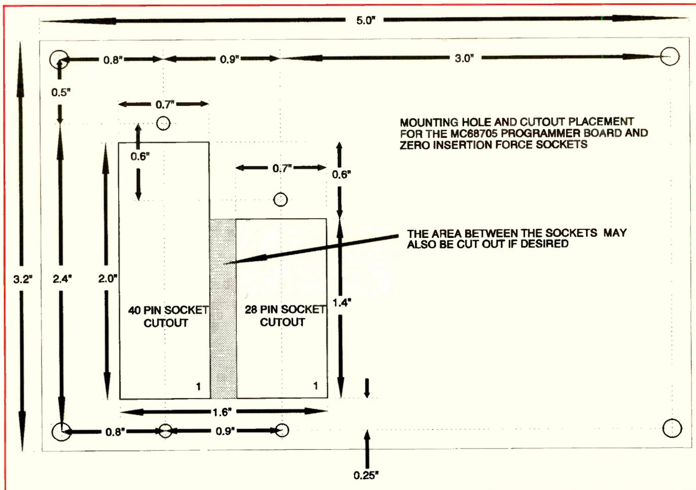
Fig. 4. Socket/pc-board mounting template.
