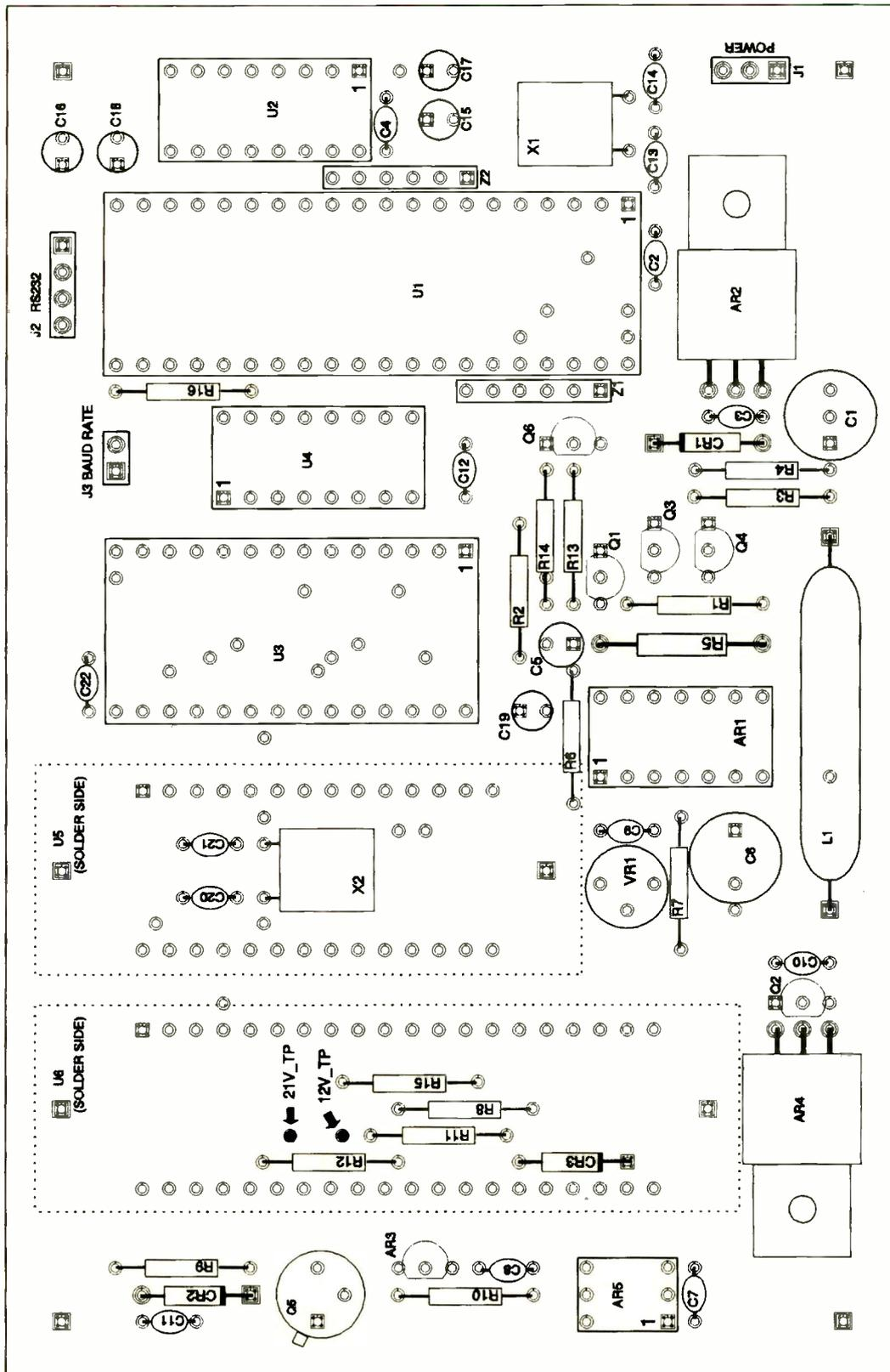
Fig. 3. Wiring guide for printed-circuit board. Note that ZIF sockets plug into standard solder-tail DIP sockets on *solder* side of board.
