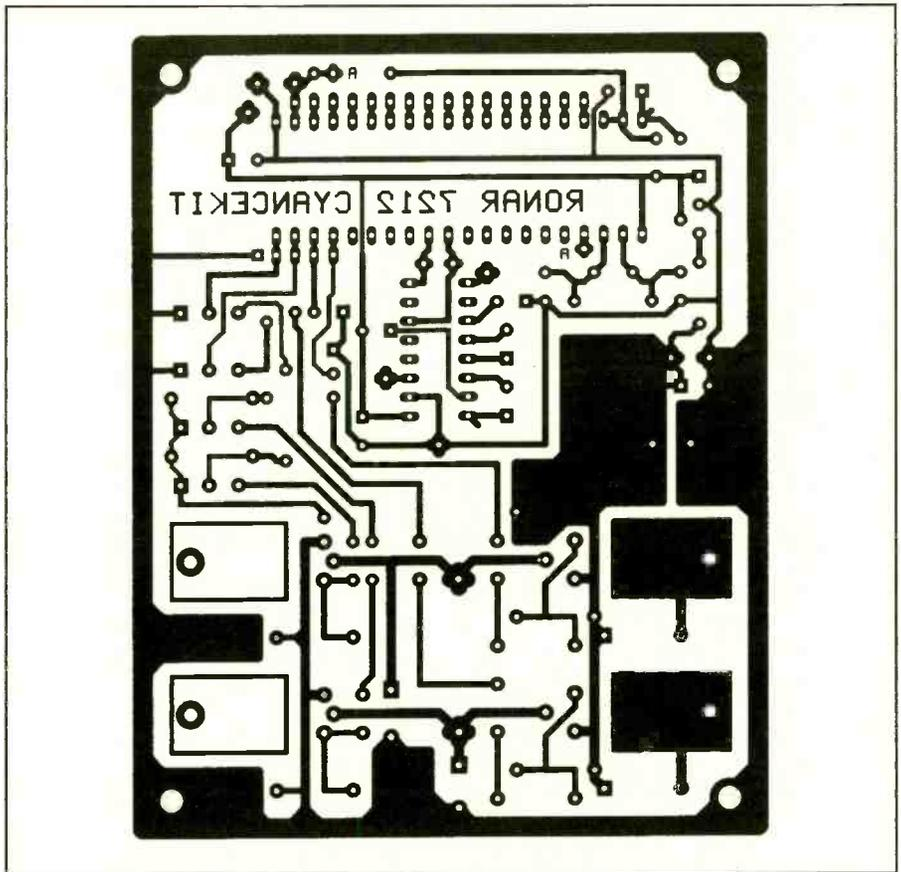
**Fig. 2.** Use this actual-size artwork for fabricating your own printed-circuit board on which to wire the motor-drive circuit.
