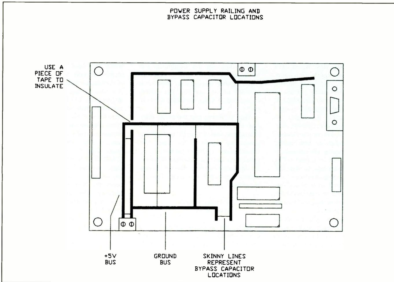
Fig. 3. Bottom view of board shows power-supply buses and locations of bypass capacitors.
