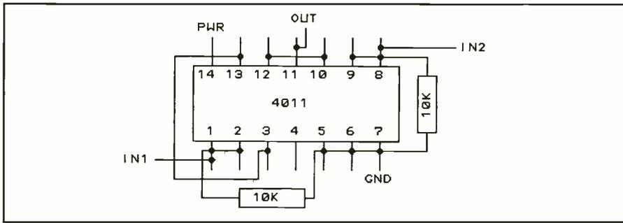
Fig. 2. Wiring details for the add-on IRQ-sharing circuit.
