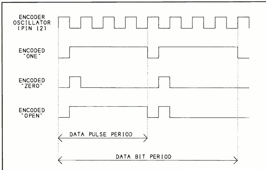
**Fig. 3.** The MC145026 trinary encoder outputs these pulse patterns to indicate logic 1, logic 0 and open-circuit conditions at its data and address inputs. Each bit requires eight oscillator cycles to transmit.
