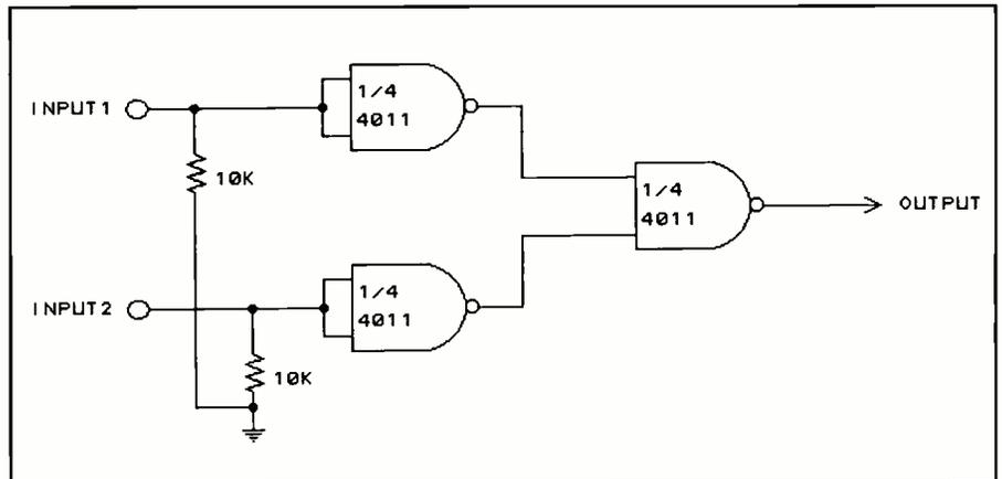
Fig. 1. Schematic details of a circuit you can use to have two devices share the same IRQ.
