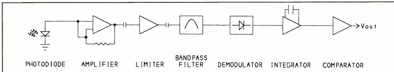
**Fig. 4.** The GP1U52X infrared receiver module is a detector, amplifier and filter in a three-pin package. When the module detects infrared energy pulsed at 40 kHz,  $V_{out}$  goes low.
