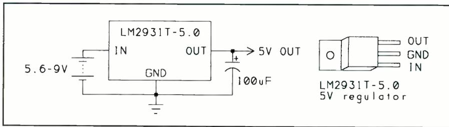
**Fig. 5.** The LM2931T-5.0 low-dropout voltage regulator creates a stable +5-volt supply with an input of 5.6 volts or greater.
