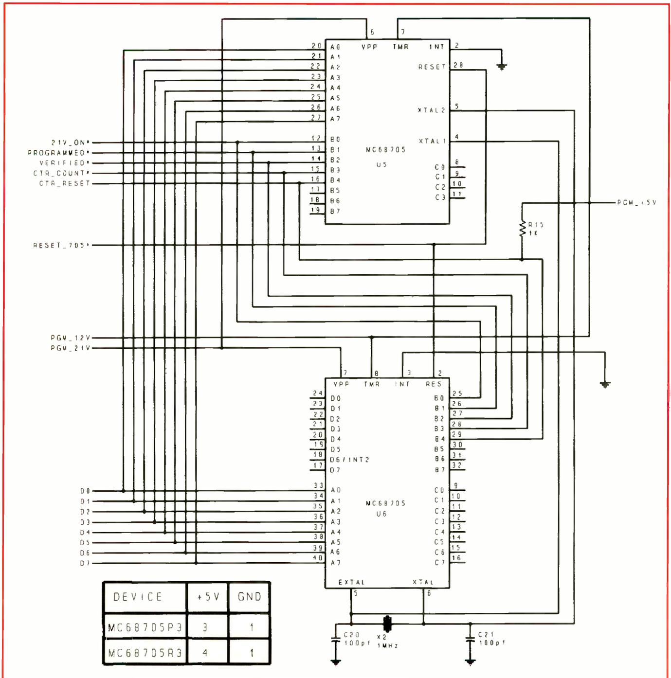
Fig. 1(C). Wiring details for Programmer's socket connectors.
