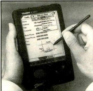
Built-in infrared transceivers provide wireless communication between two Xoomer units. In addition, an RS-232-compatible serial port allows information to be transferred to a personal computer, printer or other serial device. With an optional modem, you can retrieve data from America Online. Electronic mail can be sent and received. \$699. *Tandy Corp., 1800 One Tandy Center, Fort Worth, TX 76102.*
