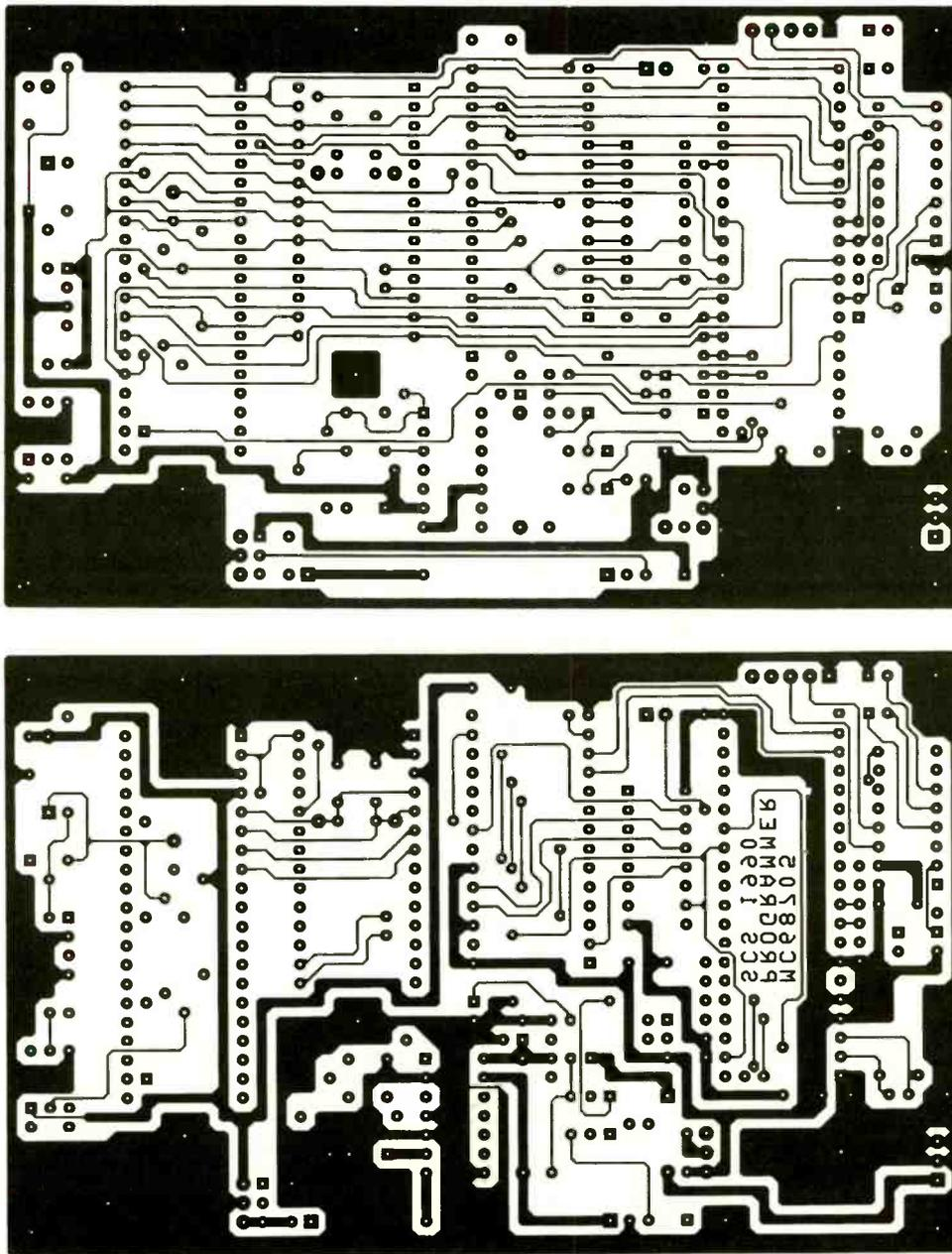
**Fig. 2.** Actual-size etching-and-drilling guides for Programmer's double-sided printed-circuit board. This board should have plated-through holes; otherwise, you must solder all connections on *both* sides of board and use short wire vias in areas where component leads/pins do not bridge from one side of board to other.
