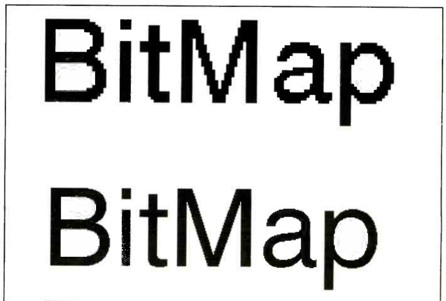
Fig. 1. “Jaggies” become more pronounced and are especially noticeable at larger sizes with bitmapped fonts, as illustrated by the characters in the upper half of this illustration. Outline-based font technologies like Adobe’s PostScript , Bitstream’s Speedo and TrueType in Windows “describe” the characters to the printer and use algorithms to produce smoother curves and better symmetry, as shown in the lower example.
