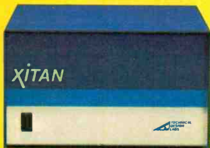
Technical Design Labs' Xitan Alpha 2 is built around the Z-80 microprocessor, a more powerful version of the 8080.
