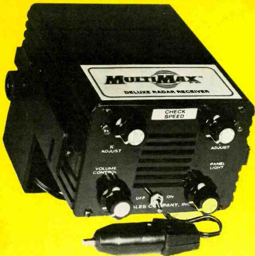
One of the newer detectors to emerge on the market is the Multi-Max dual band unit. The Multi-Max boasts separate antennas and circuitry for each band, individual fine-tuning, and standard or magnetic mount. APO Sales Co., 5201 S. Hampton Rd., Dallas, Texas 75232.
