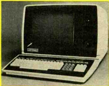
The Zentec ZMS line of desktop computers gives you in a single package everything you need in a computer—processor, memory, input keyboard and output video terminal.
