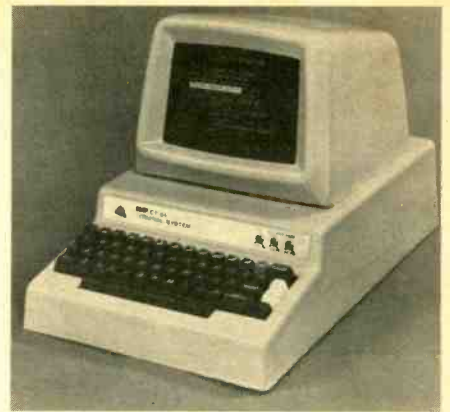
Combining a low-cost mainframe such as Southwest Tech's 6800 or the PolyMorphic Poly 88 and a video terminal with input keyboard, such as this Southwest Tech CT-64, gives you a full-function active computer for less than $1000.
