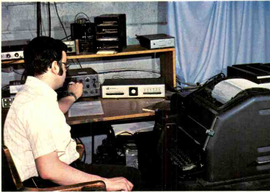
Teletype model 19, right foreground, sends and receives typed conversations in amateur radio station WB3ADI.
