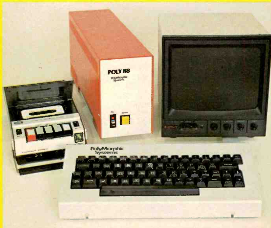
PolyMorphic Systems' Poly 88 is a very low cost mainframe computer. Adding plug-in memory boards and the peripheral equipment shown here gives you a fully functional, reasonably powerful computer system.
