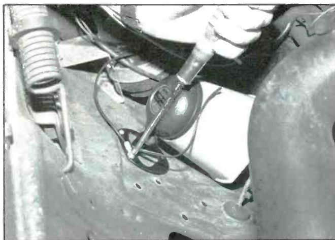
6. Drill holes for and mount the trumpet speaker in a location inside the engine compartment where it won't be accessible from outside the vehicle. Secure it in place with three screws or rivets. Use one of the mounting screws or rivets to make the system's ground connection.
