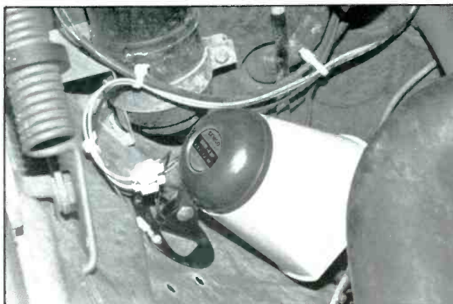
7. Route the gray conductors coming from the wiring harness and attach them to the terminals on the trumpet speaker with insulated connectors. This done, dress the wires away from other wiring and hoses in the engine compartment and secure them in place with plastic cable ties.
