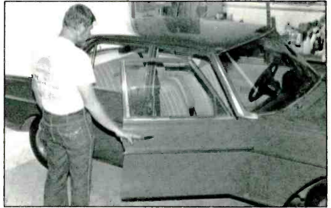
11. To test the operation of the alarm system, turn on and then off your vehicle's ignition system. Shut all doors and wait a bit more than 60 seconds to allow the system's exit delay to expire. Then open a door. When the preset entry delay time runs out, the alarm sounds.
