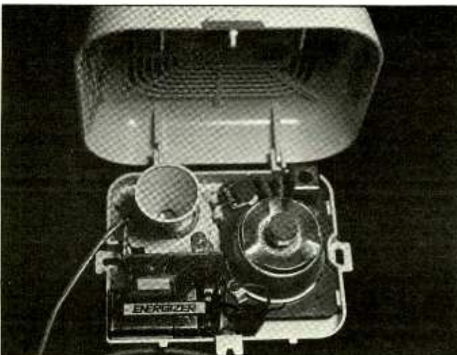
Fig. 5. Circuit-board assembly mounted inside smoke detector (at lower-left, just above battery). Cable at left goes to external remote LED/switch box.
