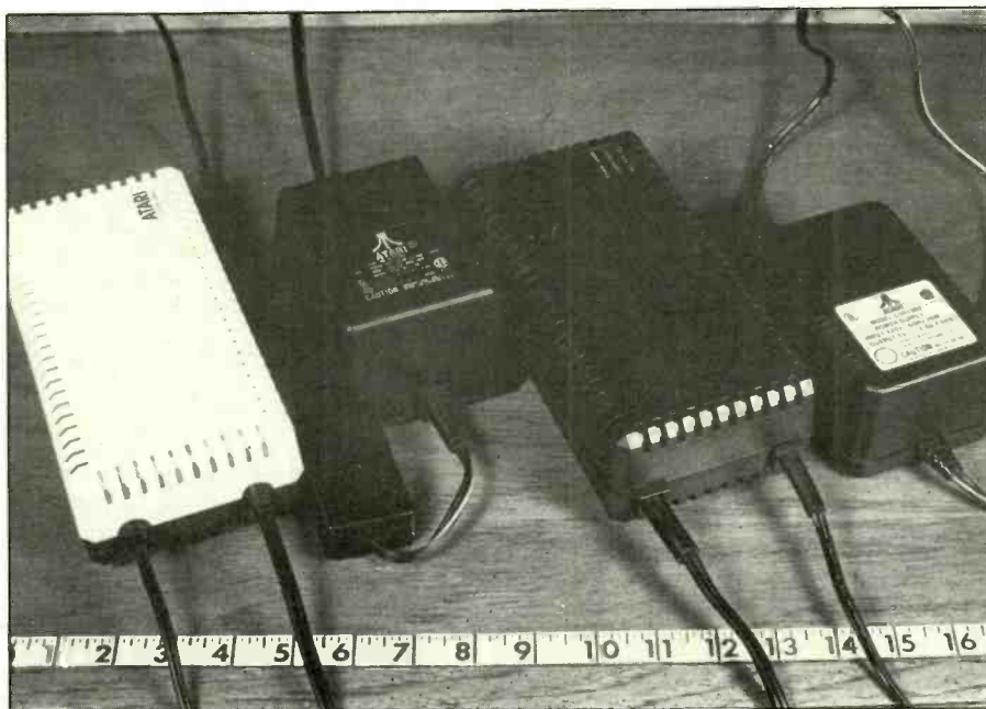
Fig. 1. Pictured here are the four major configurations of power supplies supplied with Atari XL computers arranged from Type I through Type IV left to right.
