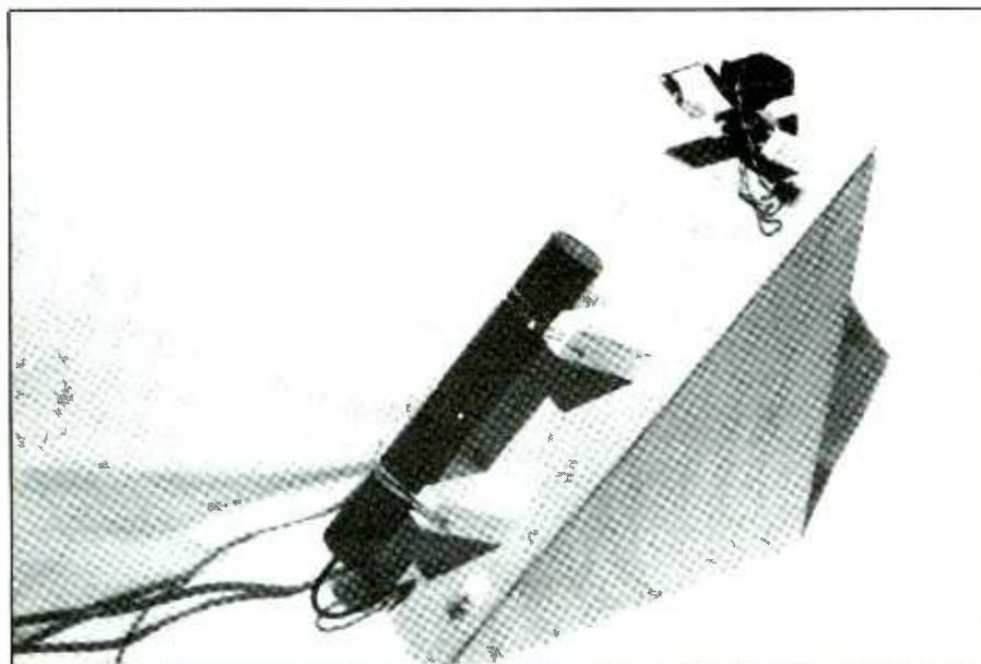
Fig. 5. In this photo of the assembled project, note how the laser tube is mounted in V blocks and is held in place with rubber bands. If an integrated laser/power supply is used, blocks must be larger and heavy-duty straps must be used.
