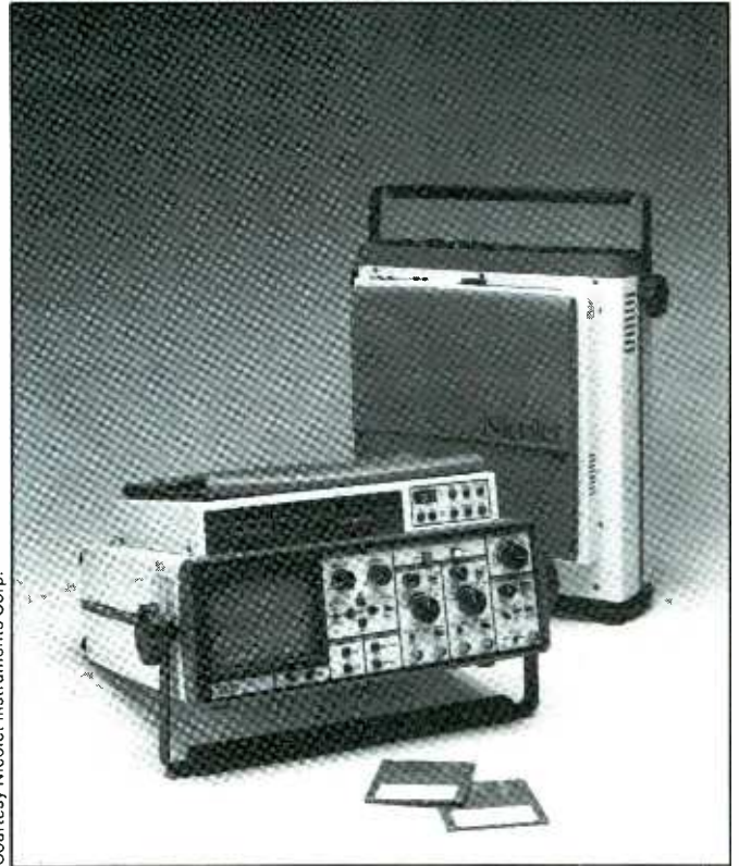
At the lofty-priced end of the performance spectrum is this new LeCroy Model 9450 DSO that features a 350-MHz bandwidth, 200 MS/s sampling rate and 50K-byte memory system.
