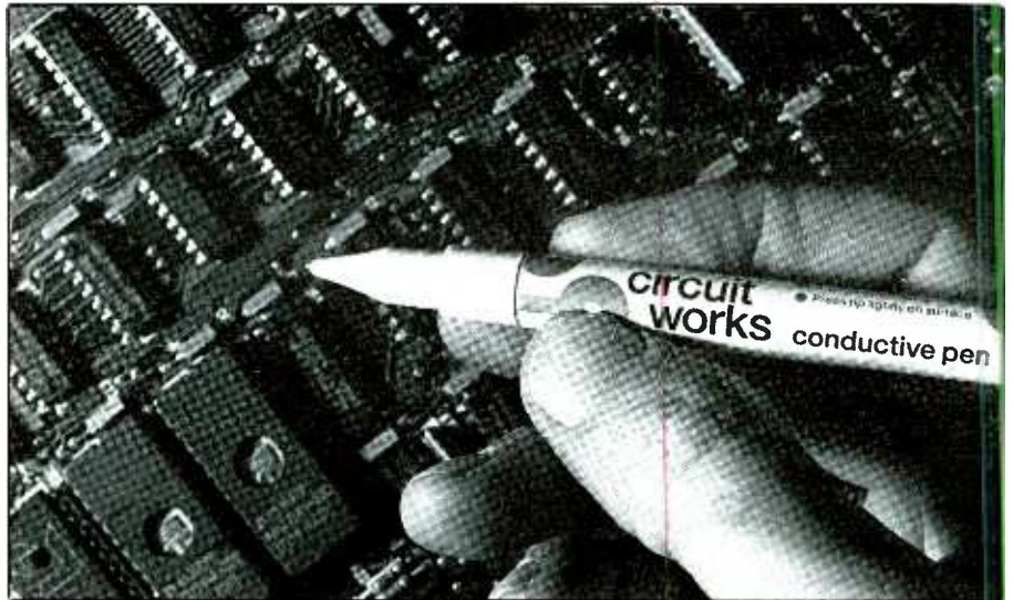
Fig. 1. Circuit Works conductive-ink pen. (Photo courtesy of Planned Products)
