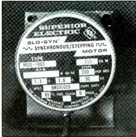
Fig. 3. An example of specifications plate that is typically affixed to stepping motors.
