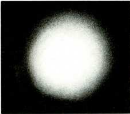
Fig. 8. Beam cross-section of Sharp LT9512U oversize LED.
