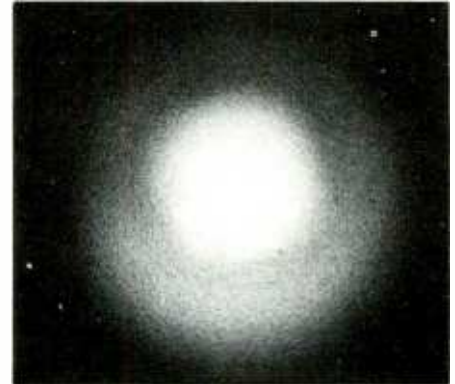
Fig. 7. Beam cross-section of International Devices ID 3000-UR LED.
