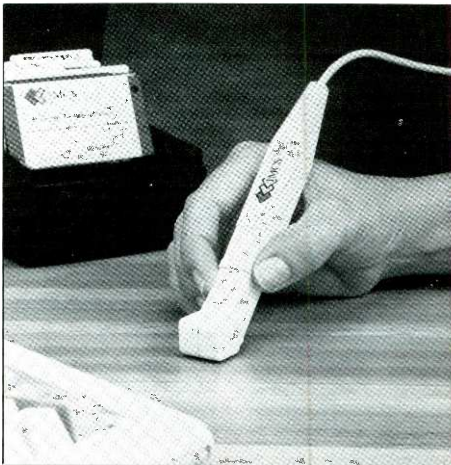
Appoint's MousePen, as its name implies, is a mouse pointing device housed in a pen-like enclosure. Handled in much the same manner as you would a pen marker, this device requires very little desk space to operate and hardly any learning time at all.
