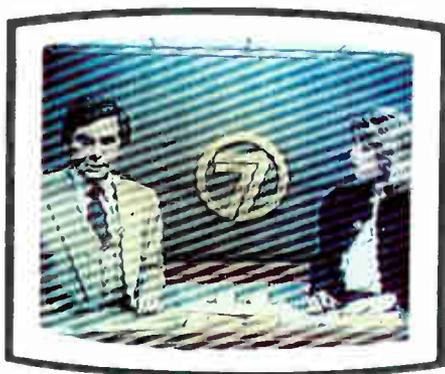
This pattern may appear on your television screen when your set is receiving signals from a CB, amateur, police, or other two-way radio transmitter. The pattern will only appear when the operator transmits. It may vary according to the type of signal being received. You may also hear the operator's voice.
