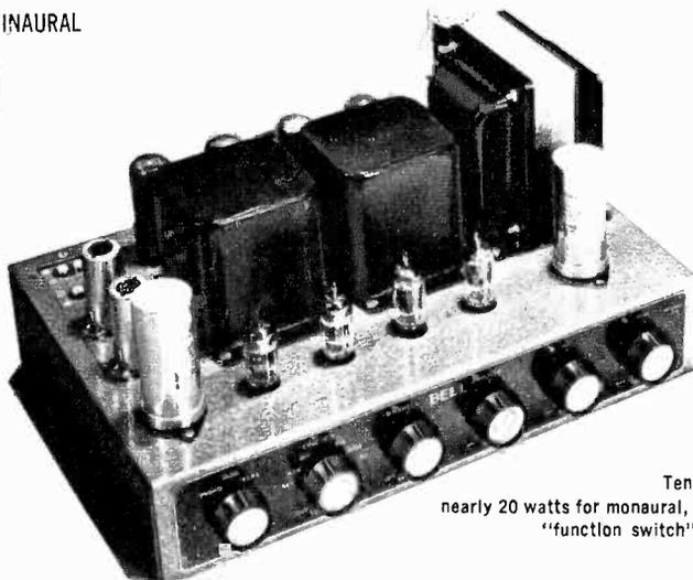
Ten watts for each channel, or nearly 20 watts for monaural, is available by a flick of the "function switch" on this Bell 3-D amplifier
