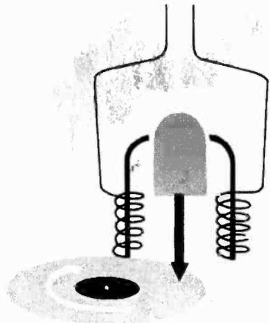
Cup-shape stylus assembly can be lifted out by your fingernail, features high-output German-made Miratwin magnetic pickup
