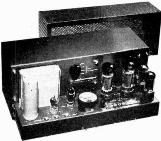
New Marantz has built-in meters for continuous testing of tube performance, produces 40 watts or 20, depending on circuit used. Rugged, conservative construction explains price of \$198
