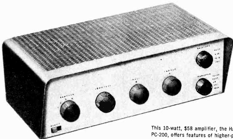
This 10-watt, \$58 amplifier, the Harmon-Kardon PC-200, offers features of higher-priced units: separate rolloff and turnover controls, tape preamp
