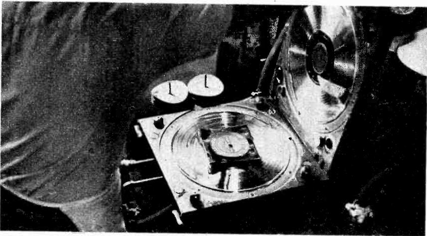
Forty seconds later a finished record emerges. The rough edge of surplus vinylite will be sliced away later by an automatic knife while the next record is being pressed
