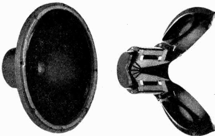
British-made Tannoy coaxial mounts the high-frequency horn behind the apex of the low-frequency cone, uses the curvature of the cone to assure adequate dispersion of high-frequency sounds
