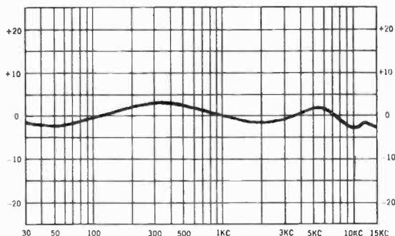
Records are cut with treble boost and bass de-emphasis—a line running up on the graph from left to right. Sonotone pickup equalizes by constant-amplitude response, to produce almost level response line, as shown
