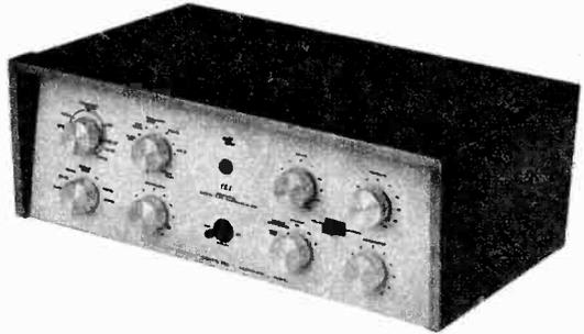
McIntosh preamp, matched to big McIntosh amplifier, has push-button choice of turnover and roll-off curves, variable rumble filter
