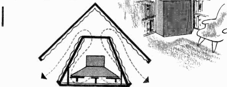
Klipsch design blocks the front of the speaker, brings front waves around to reinforce rear waves. Sound emerges from sides; corners of room form mouth of the horn
