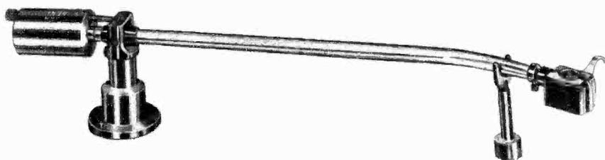
Electro-Sonic tone arm, made to be used with the same manufacturer's pickup, is one of the longest in the stores. Tracking weight is adjusted by means of a spring balance in the cylinder at the rear
