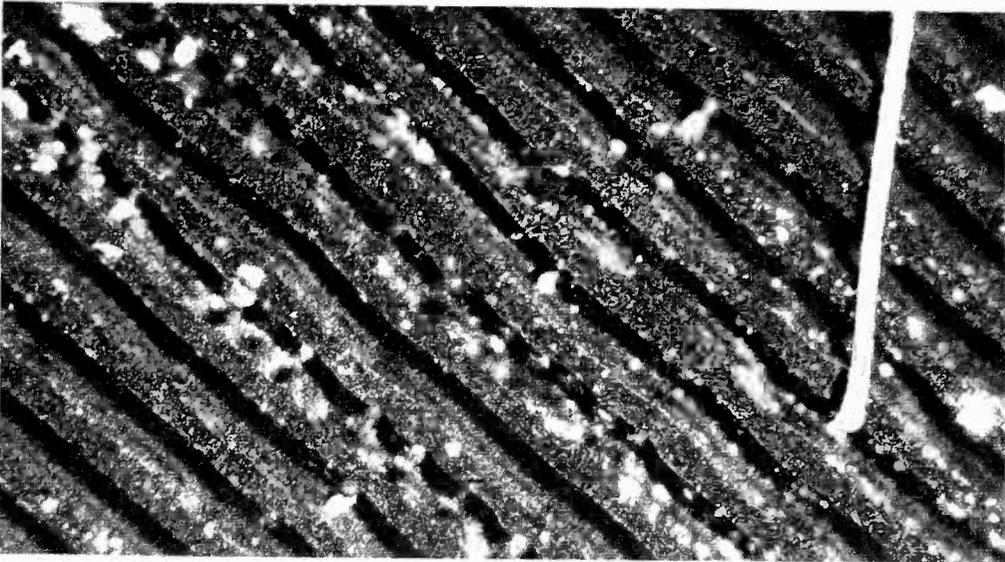
Here is an old and mistreated record, seen through same microscope. Note the dust on the surface of the grooves, and the chipping away on the walls of high-frequency wiggles
