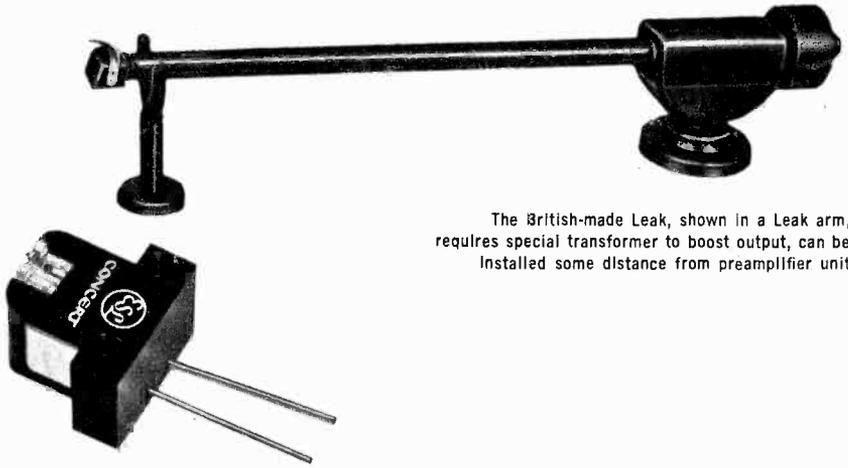
The British-made Leak, shown in a Leak arm, requires special transformer to boost output, can be installed some distance from preamplifier unit
