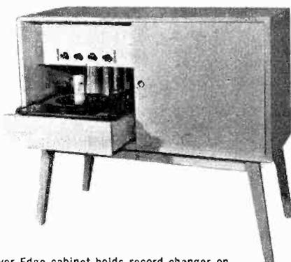
River Edge cabinet holds record changer on low sliding drawer, preamp-control unit above, power amplifier behind the closed door
