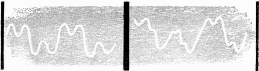
Here, graphically shown, is intermodulation distortion. At left is the correct pattern. At right is the uneven pattern produced when two frequencies, fed simultaneously into the system, distort each other
