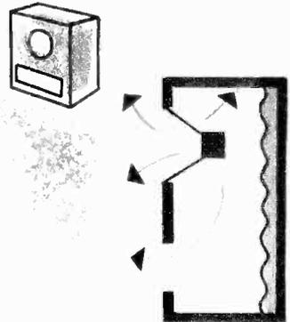
Bass-reflex box, most common kind of enclosure, brings rear waves around through port to reinforce the bass sounds from the front. Padding absorbs high-frequency rear waves
