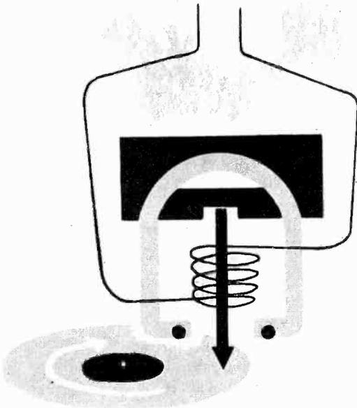
Above is schematic of dynamic pickup. As the stylus swings back and forth between the magnetic poles, the moving coil feeds out an alternating current
