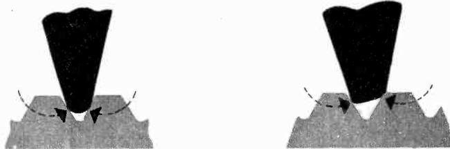
New stylus rides on only two points at its rounded tip. Flats wear on the two points, and eventually the shape of the tip changes.
