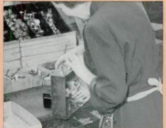
Assembly line employee attaches necessary operating controls to radio receiver chassis.
