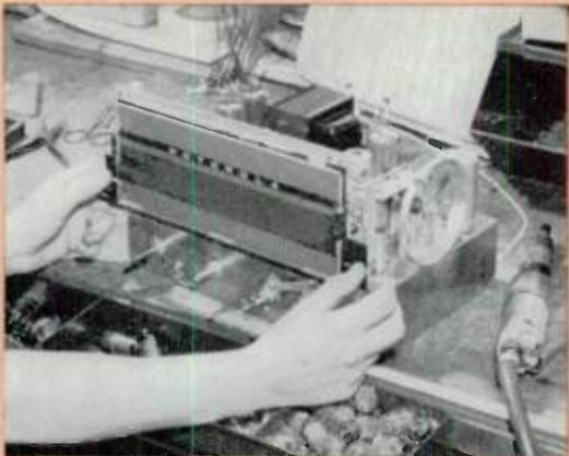
Radio dial scale is put together by skilled employee on assembly production line.
