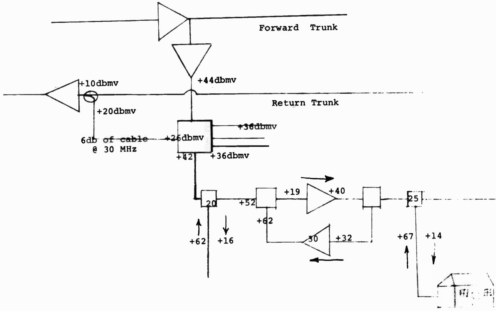
Figure 6 Bi- Directional Feeder System
