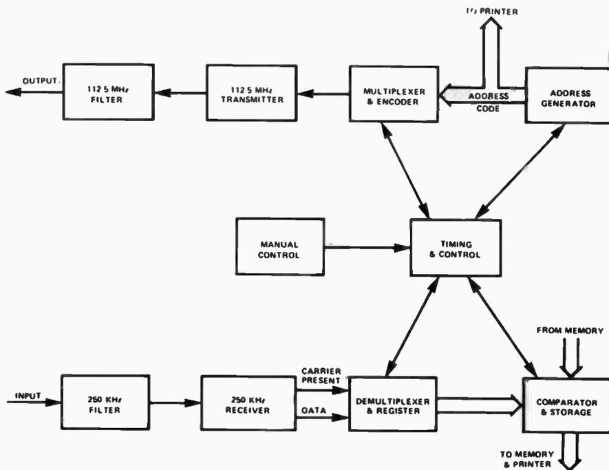
Figure 13 Control Unit Block Diagram
