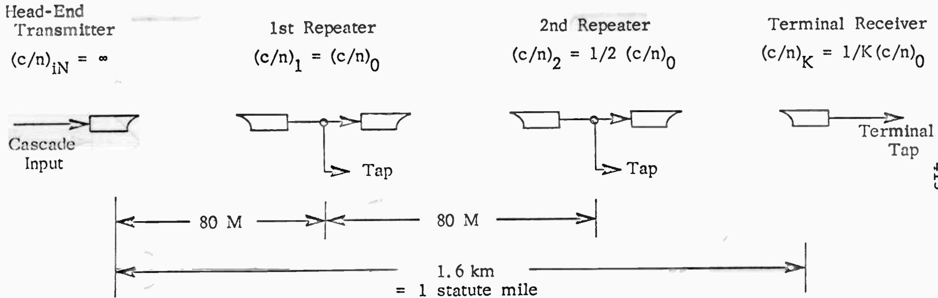
FIGURE 1. ONE MILE CASCADE OF K OPTICAL LINKS
