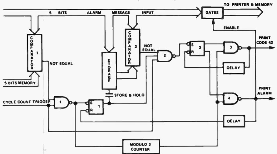
Figure 16 Alarm Comparator
