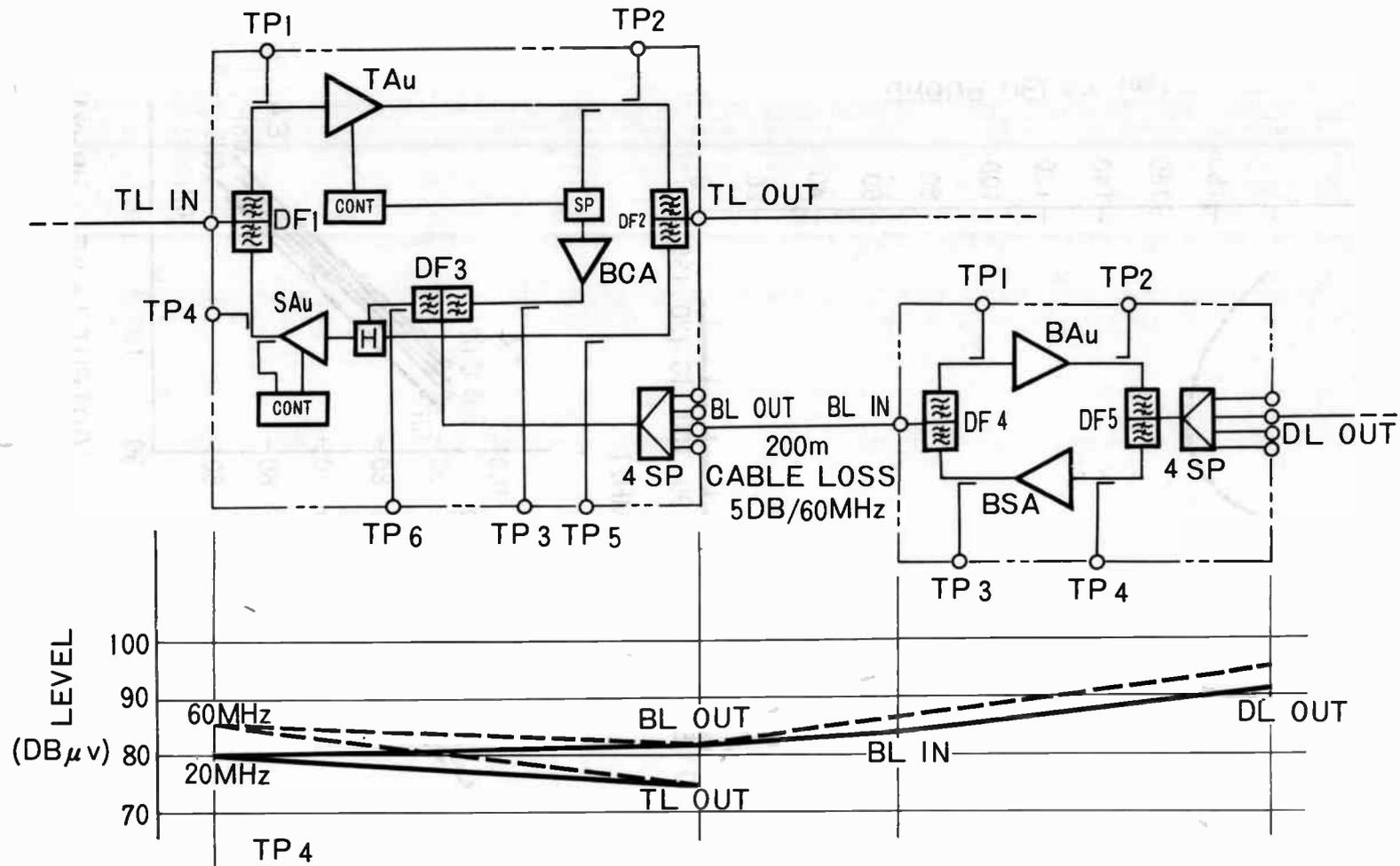
Fig-9 BLOCK DIAGRAM & LEVEL OF BI-DIRECTIONAL TRUNK & BRIDGING AMPLIFIER
