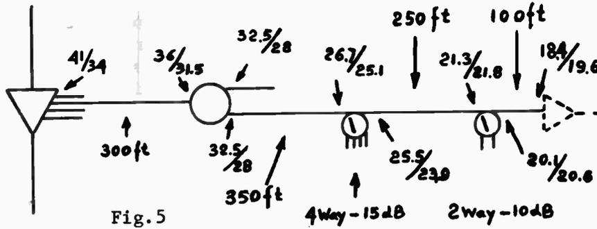
The first 300 ft. cable piece is represented by a straight line between it's input levels of 41/34 and it's output levels of 36/31.5. The 2 way splitter is represented by a straight line between it's input levels of 36/31.5 and it's output levels of 32.5/28. The other levels are represented similarly. It should be noted that the lines representing the flat losses of the splitter and taps have a 45 degree slope on the graph, while the lines representing cable are nearer 30 degree.
