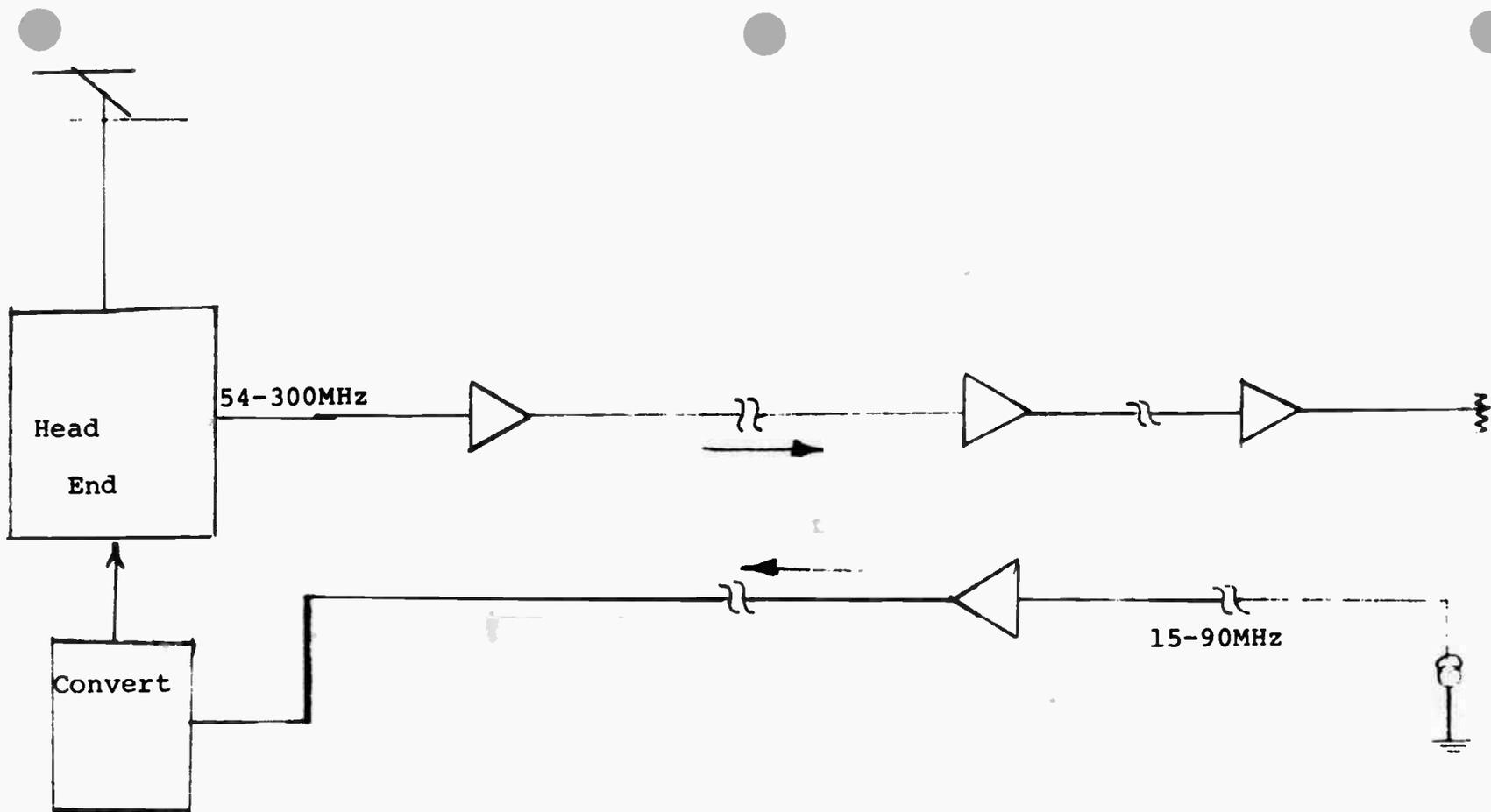
Figure 4 Dual Cable Bi-Directional System
