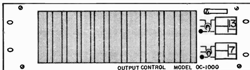
The output Control Chassis, Model OC-1000, provides output switching capability. Front-panel switches are provided to allow operator manual override selection of either the "Normal" or "Alternate" input, or the automatic mode of operation.
