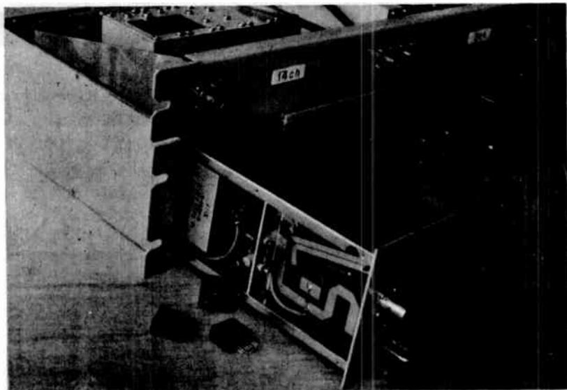
Photo 2 UHF RECEIVING UNIT OF IC DESIGN SIGNAL PROCESSOR ,
