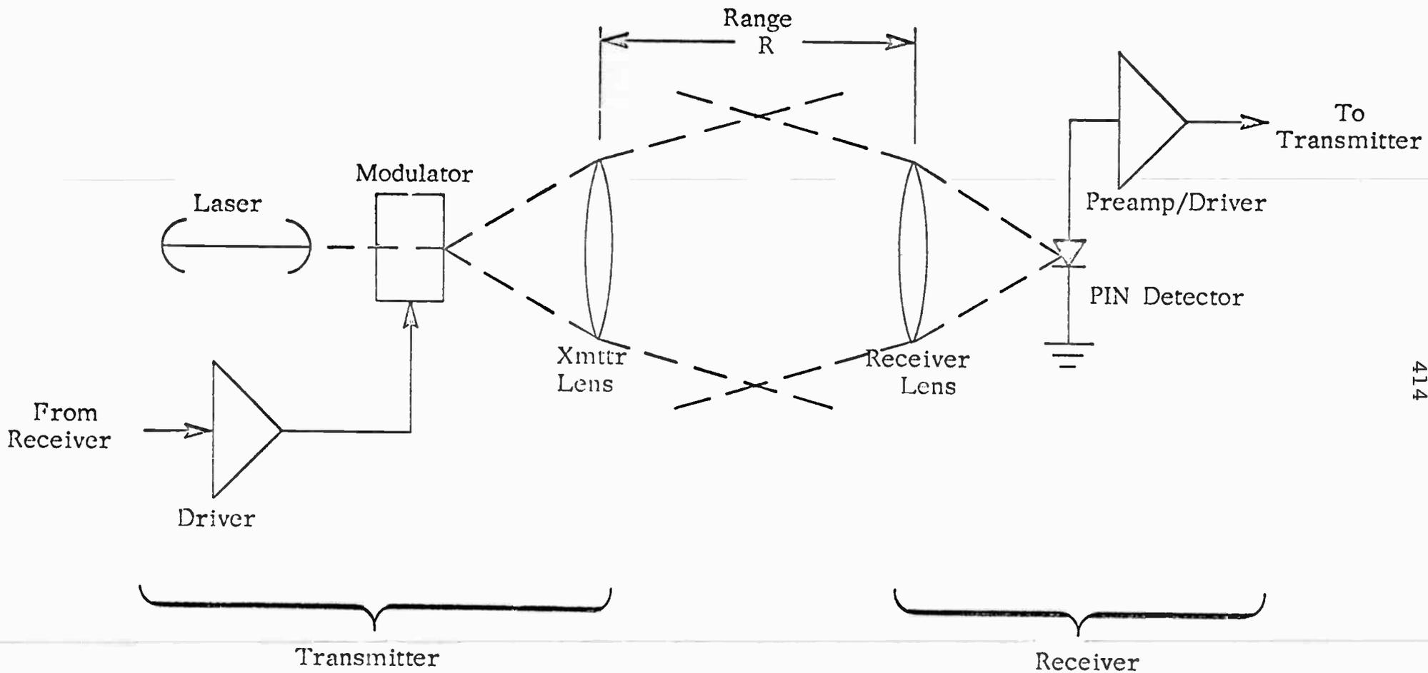
FIGURE 2. SCHEMATIC FOR ONE CASCADE LINK ELEMENT FOR CATV
