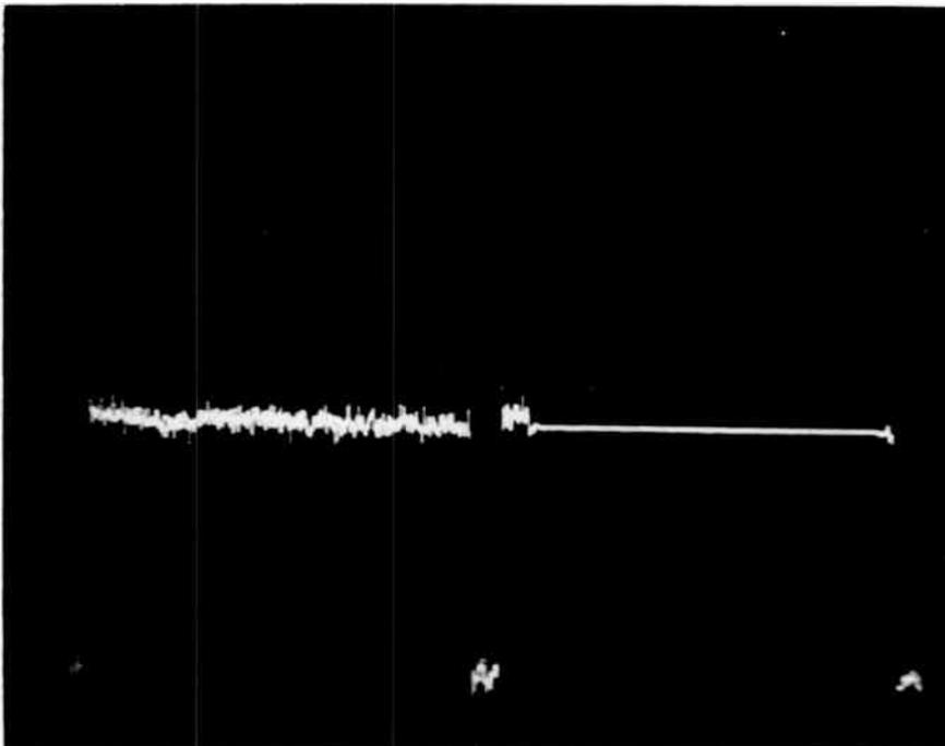
Display shows two successive lines in vertical blanking interval as shown on waveform monitor using the line selector.
