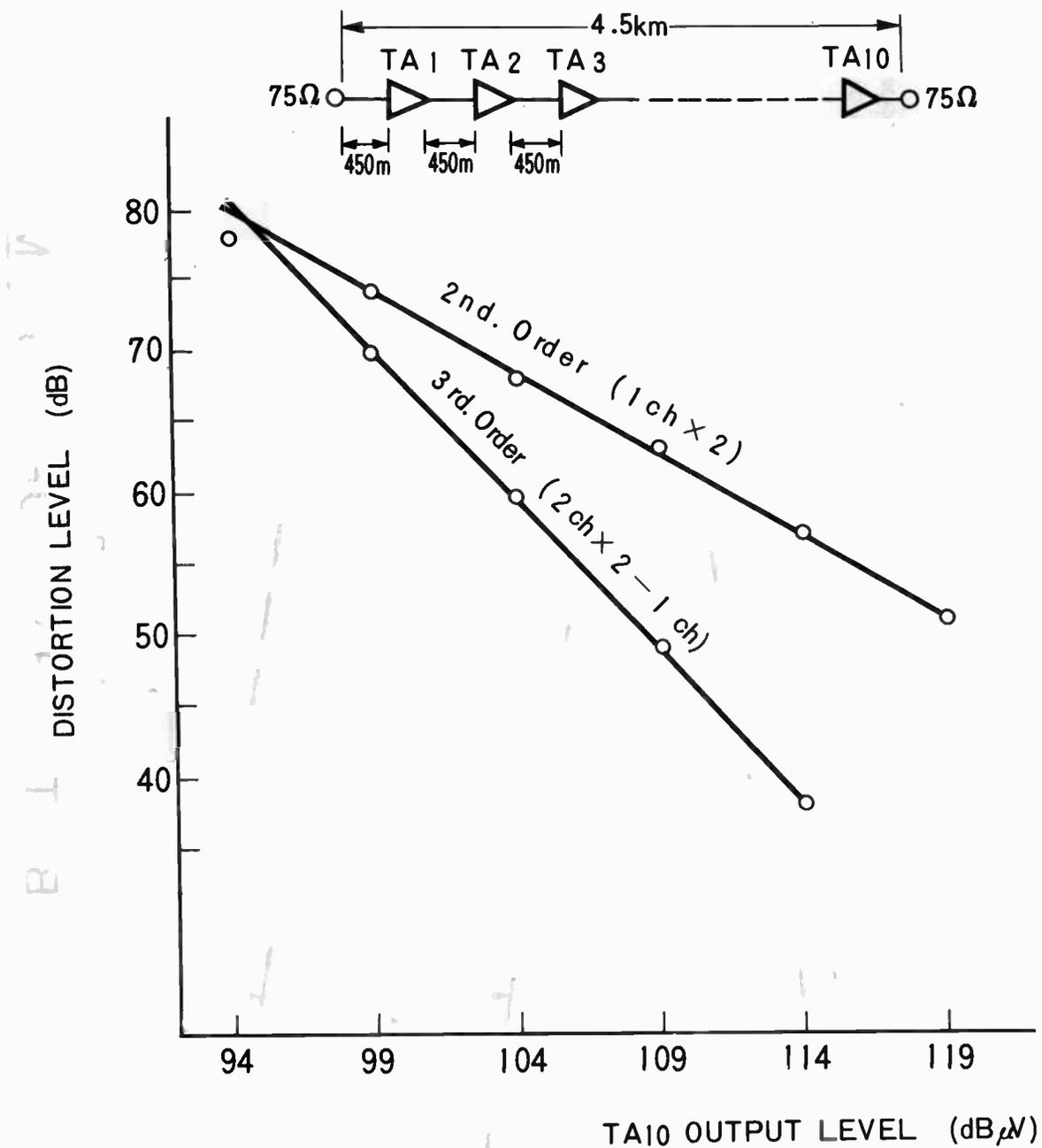
Fig. 7 MEASURED DISTORTION CHARACTERISTICS FOR 10 CASCADED TRUNK AMPLIFIERS.
