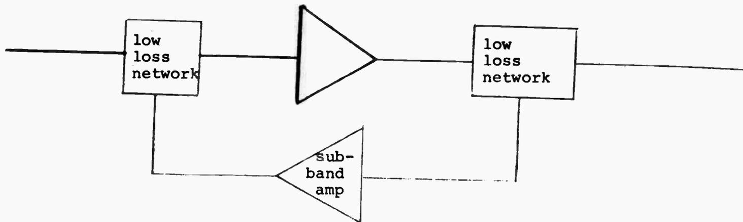
Figure 3 Single Cable System using loss filter networks
