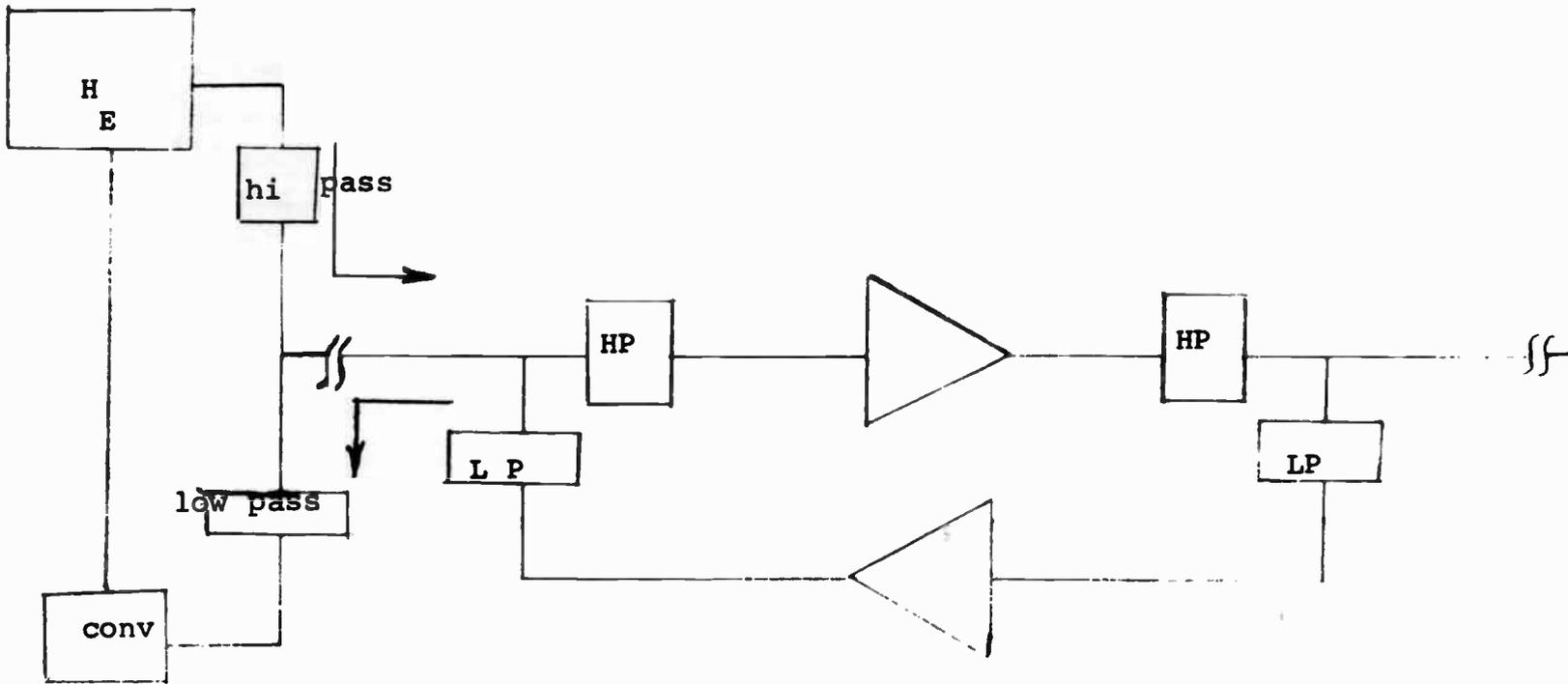
Figure 2 Single Cable System using standard diplexing filters
