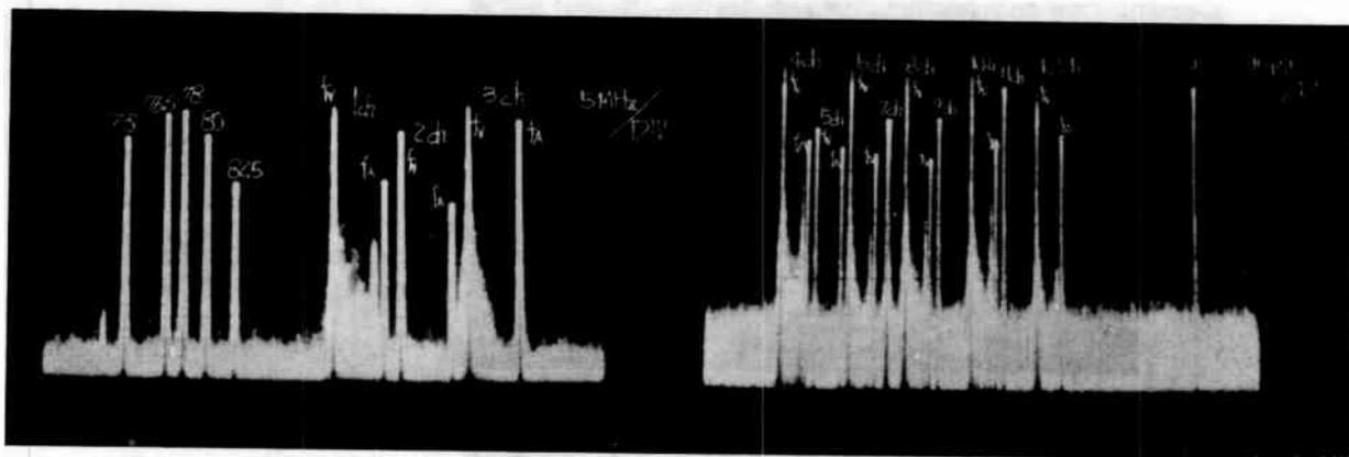
Photo 3 FREQUENCY SPECTRUM OF MULTI-CHANNEL TRANSMISSION
