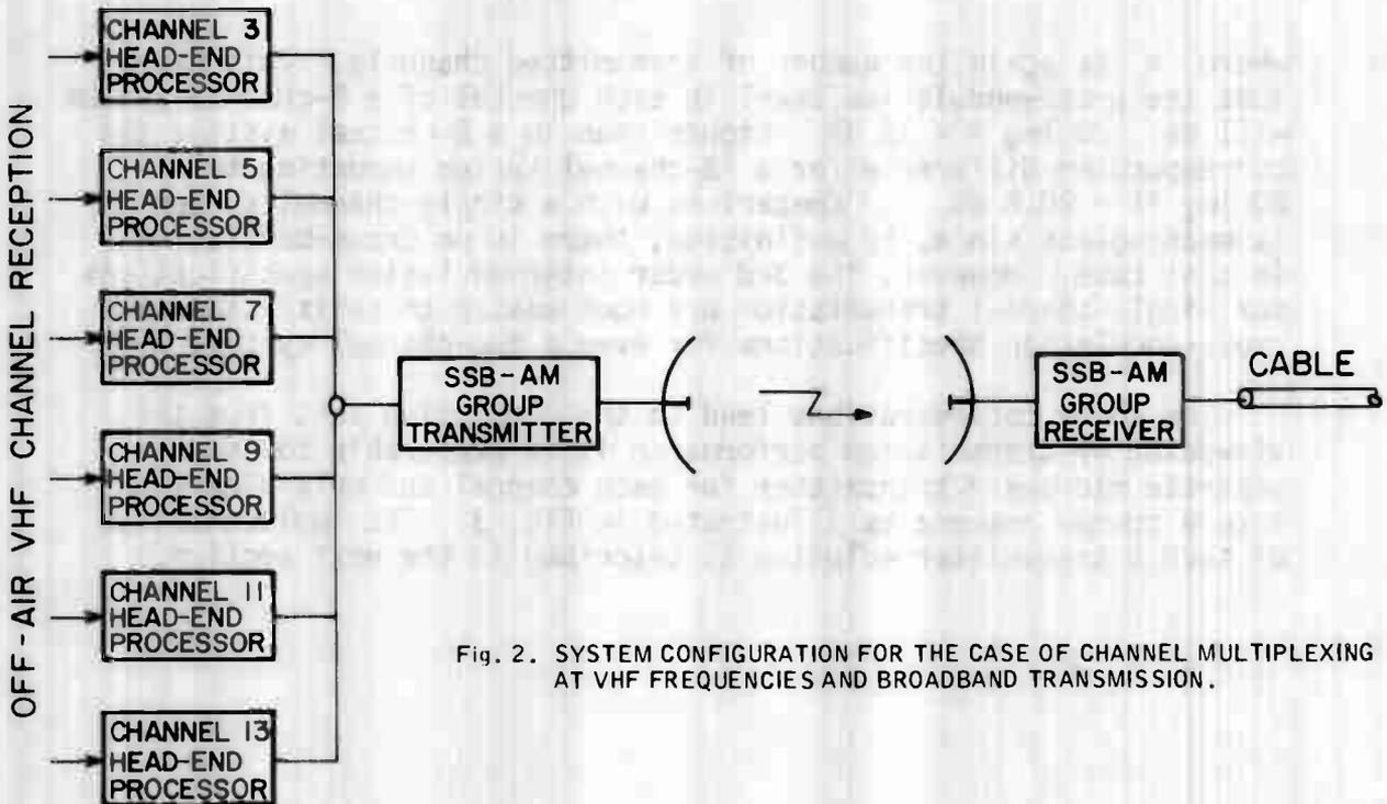
Fig. 2. SYSTEM CONFIGURATION FOR THE CASE OF CHANNEL MULTIPLEXING AT VHF FREQUENCIES AND BROADBAND TRANSMISSION.
