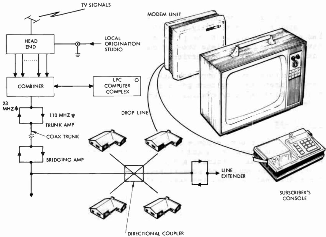
Figure 1. Overall CATV Two-Way System
