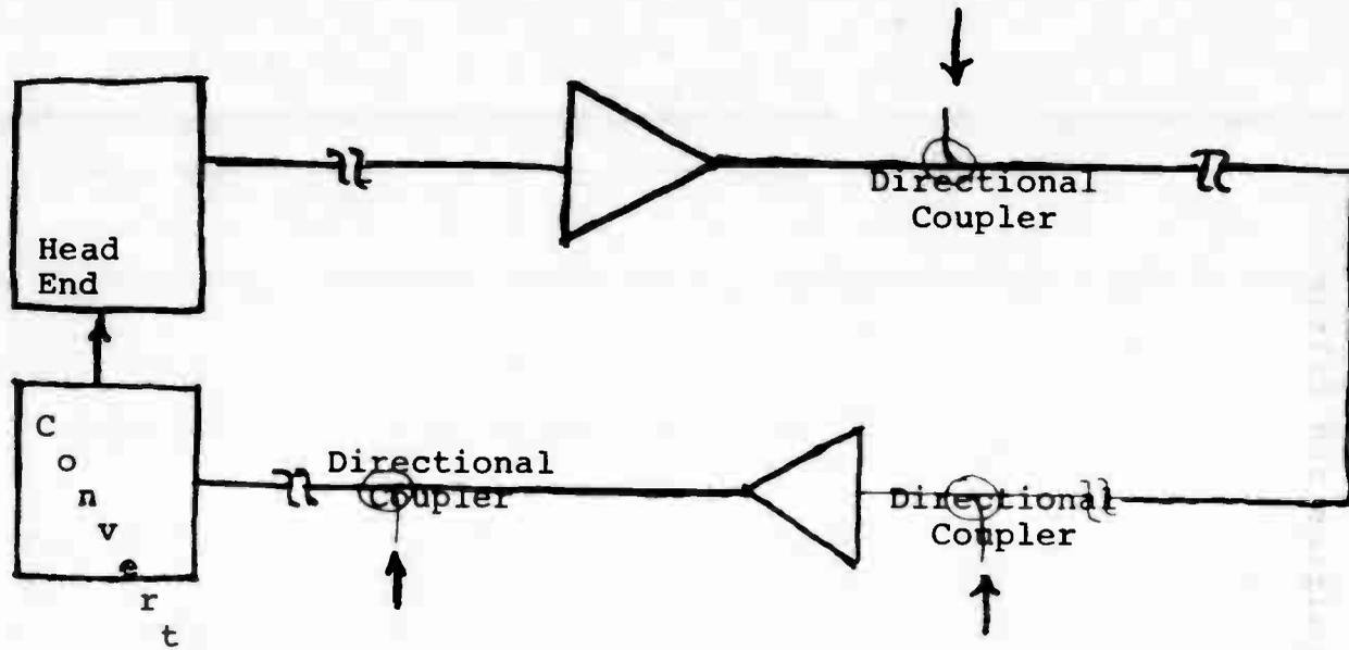
Figure 1 Closed Loop System
