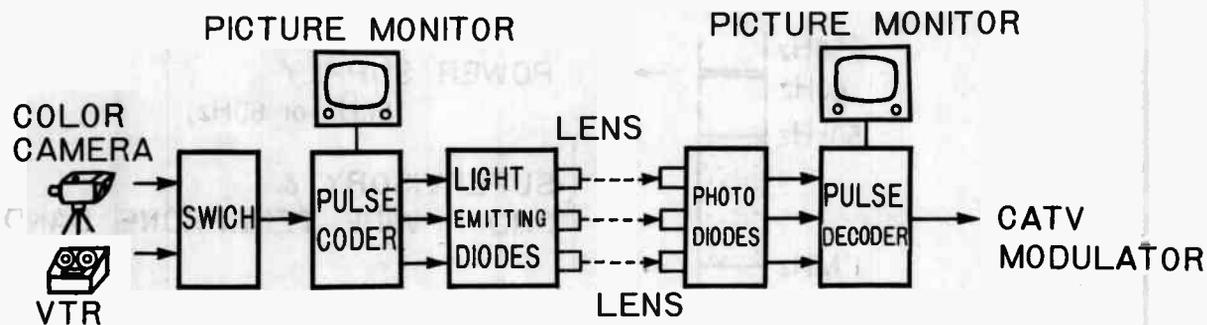
Fig. 3 OPTICAL COMMUNICATION LINK
