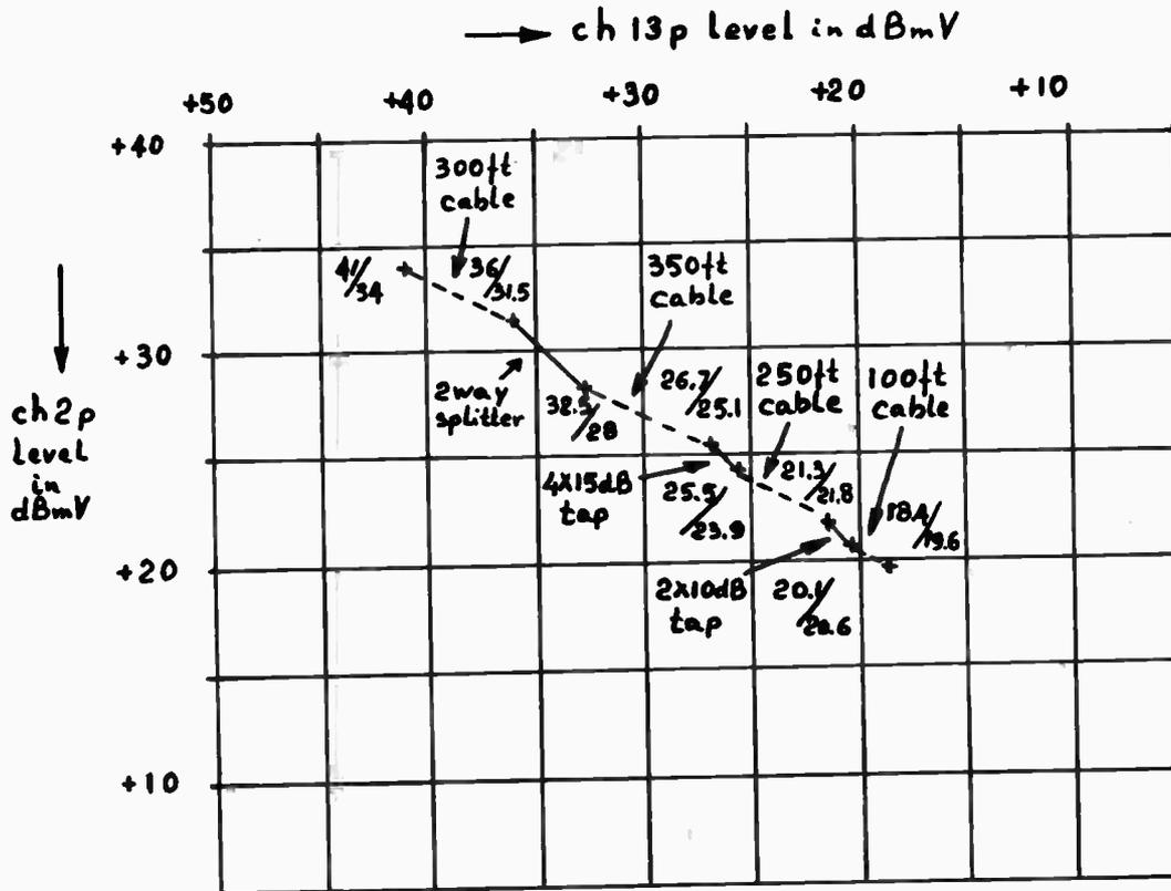
The graph can contain more information. Figure 7 shows the 2 way 10dB tap again; the horizontal dimension of that square represents the through loss at ch 13p; the vertical dimension represents the through loss at ch 2p.
