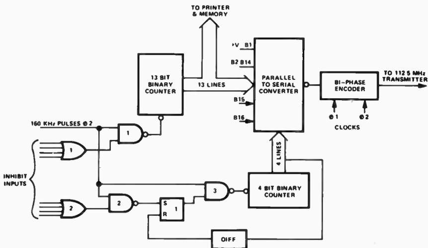
Figure 14 Address Generator & Multiplexer
