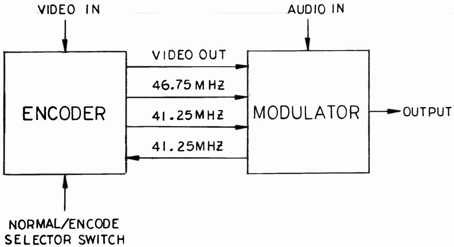
FIGURE 2-INTERCONNECTIONS BETWEEN ENCODER & MODULATOR
