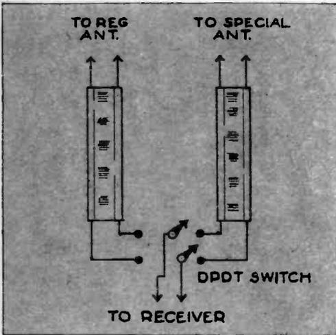
Where an extra antenna is used to bring in a weak station, use a separate transmission line and connect it to the receiver as shown. The antennas below and at right are indoor types for use in strong-signal localities.
