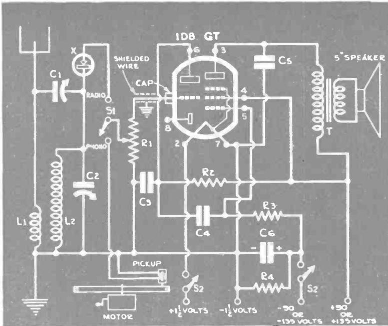
This one-tube circuit actually includes a two-stage amplifier fed either by the pickup or by the tuned circuit and detector. Parts are keyed to the list at the bottom of the next page.
