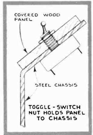
The chassis is a 6" by 6" metal sheet bent to conform with the slope of the wood panel. The cabinet is covered with artificial leather both inside and out.
