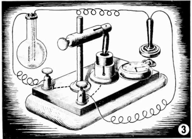
granules in a quiet room. Note, too, how they react to different letters in the alphabet. Such a mike is erratic at various frequencies and is hardly of high fidelity. Held in different positions, it varies in sensitivity, and frequently its granules pack. But in spite of drawbacks, the carbon mike has reached a good stage of development in telephones, walkie-talkies, and tank and plane radios.
