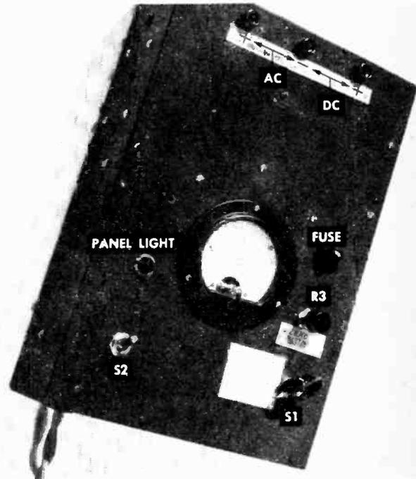
5. Range switch, test-prod jacks, and zero adjustment must be located on top of the panel.
