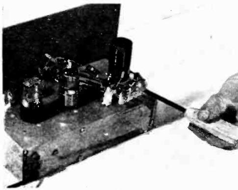
Pretune the set with a neutralizing tool or a bakelite shaft ground to a screwdriver tip.
