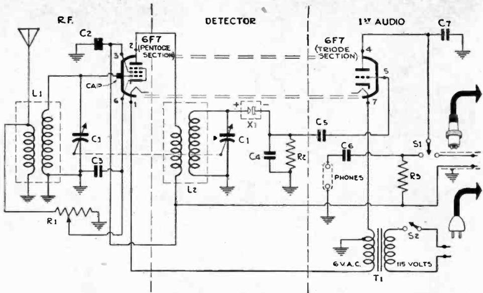
The cathode-regenerative circuit employed in this one-tube tuner is free of whistles and howls, and causes no interference with other radios. A tiny new crystal used in wartime radar equipment acts as the detector, replacing the more conventional diode.
