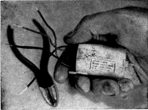
Many components can be purchased with tinned wire leads, all ready to solder into the set. Push about  $\frac{3}{8}$ " of insulation back from end.
