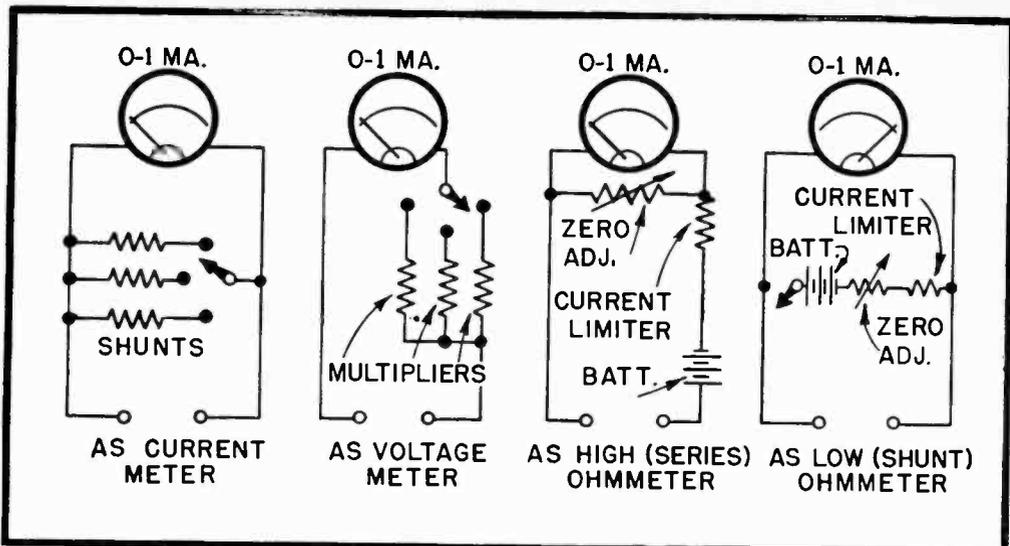
**Basic Principles of V-O-M meters.** Any fairly sensitive current meter will register higher values of current as well as volts and ohms if
