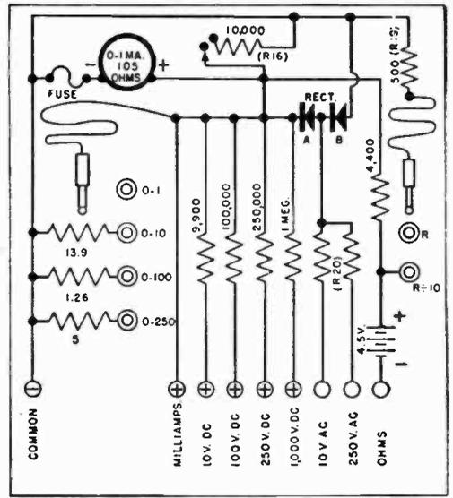
For portability the high-ohms range has been omitted, doing away with the 45-volt battery.
