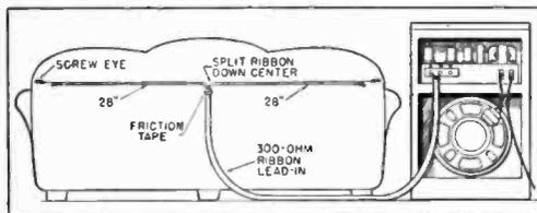
IF EITHER YOU or the landlord objects to your hanging an FM antenna on the roof, this indoor rig may help you get reception. Antenna and lead in are of one-piece construction, consisting of a length of 300-ohm ribbon lead-in. Wrap a few turns of tape around the wire 28" from one end and split it down the center. Drive hooks or screw eyes into the frame of a davenport and fasten the ends of the ribbon to them. The other ends go to the antenna terminals on the receiver.
