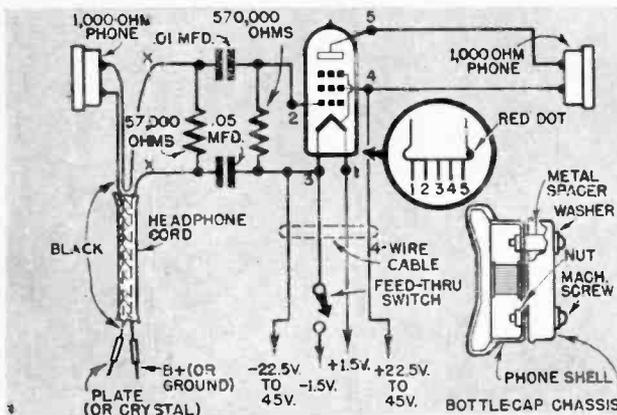
Tube connections are soldered directly to the pins. Use a small iron and try to solder each joint quickly; too much heat may cause damage.
