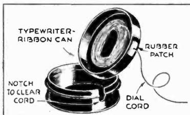
**DIAL CORD** won't snarl up in a serviceman's kit if it is carried in a dispenser such as that shown above. Drill a hole about  $\frac{1}{8}$ " diameter in the upper part of a typewriter-ribbon can and cut a corresponding notch in the lower piece. Cement a small rubber patch over the hole, and when the cement has dried, punch a pinhole and draw the cord through. The patch acts to prevent the cord from slipping back inside.—R. P. TURNER.
