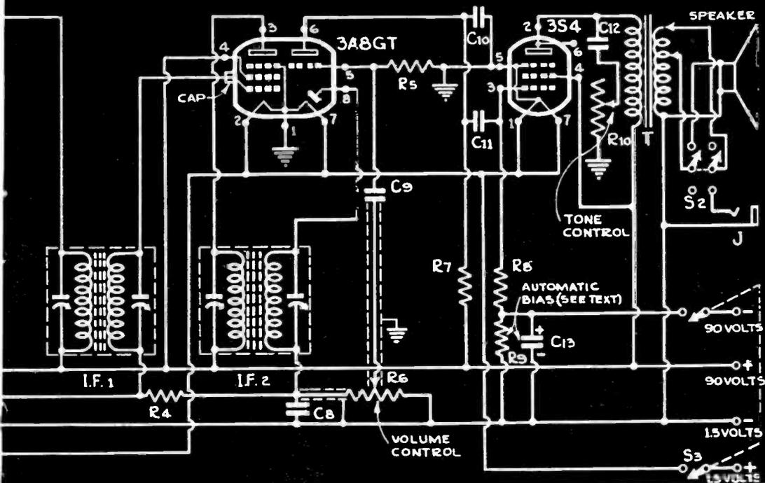
selected because it has room for a 1,000-hour power supply. Battery packs that deliver 1.5 volts for the filaments and 90 volts for the plates are now available in a variety of sizes and shapes. Where portability is a factor, a small pack may be used, in which case the cabinet can be much reduced in size. The larger of the so-called "farm" packs are estimated to be good for a full year of service with this low-drain circuit, based on average daily use of about three hours.
