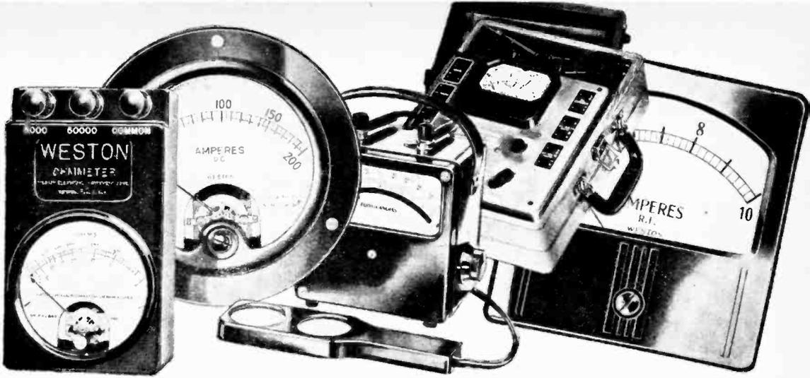
Two delicate hairsprings carry current to the coil and also serve to position it so that the pointer is normally at zero on the scale. When current flows in the coil, interaction of the lines of force produces a torque. This torque rotates the coil and its pointer to a position where it balances the opposing torque of the springs.
