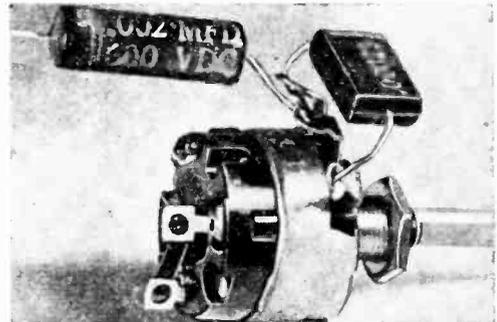
**Soldering** can be simplified by making all convenient connections before mounting parts.
