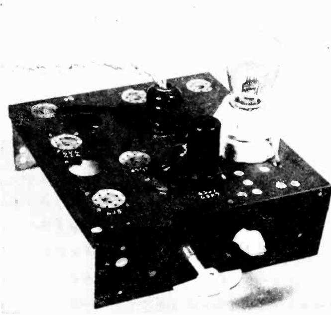
Extra sockets can be added. This chassis has one for testing 6SQ7's
