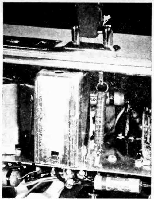
Here's part of the spring-suspension system that helps protect this set from the jolts and bumps that shorten the life of most portables. Anchored between soldering lugs on the chassis and case, two tension springs provide a "floating" or shock-absorbing support for one edge of the chassis.
