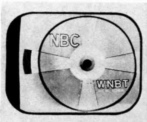
**Horizontal centering**, like the vertical, brings the picture frame inside the limits of the mask. Misadjustment of this control could also push the picture to the left. Usually a rear adjustment.
