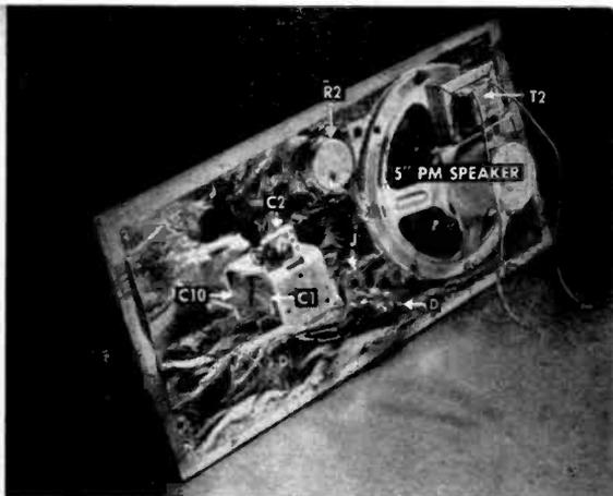
Aluminum foil stapled to the front panel acts as a common ground or chassis and also provides shielding for the variable condenser.
