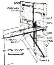
FIG. 22. When open, the lower door supports this ironing board.
