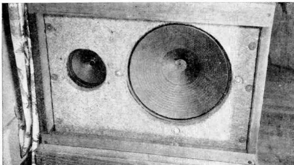
Speakers are mounted behind openings cut in a baffle made of soft fiber board. They are then
