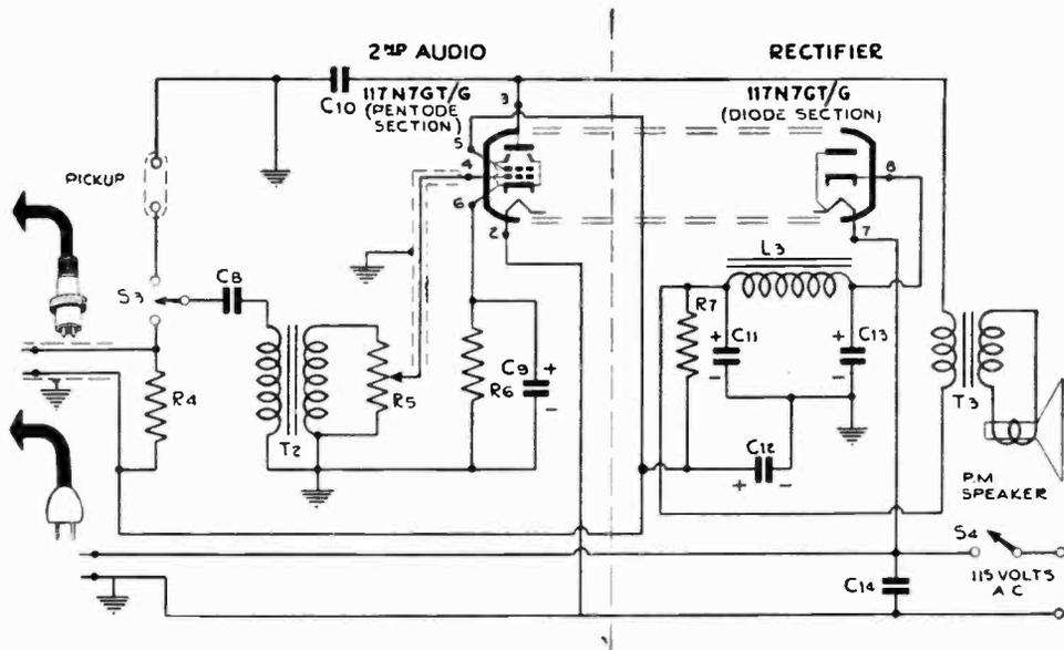
One stage of amplification is enough to drive a 12" speaker at comfortable volume, but a smaller unit can be used if preferred. When operating with a phonograph, the amplifier gives best results if coupled to a crystal pickup of the high-output type.
