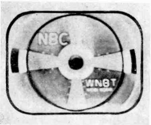
**Focus** is important to a good picture. A clear picture is obtained by sharpening the cathode-ray spot. Most sets have a variable focus adjustment. Sometimes it's in front, often in back.
