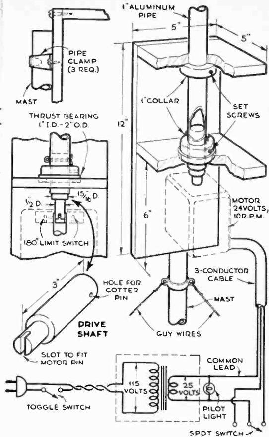
Electrical controls, consisting of an on-off switch, an SPDT reversing switch, a pilot light, and a 25-volt transformer, are incorporated in a box. Outdoor parts are boxed in with sheet copper for protection against the weather.
