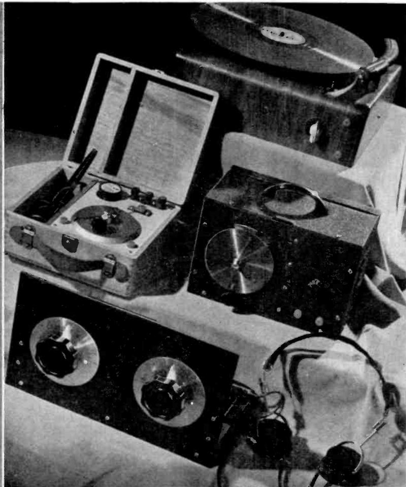
Radio-phonograph combinations strike a new note in crystal-set construction. The complete yet extremely simple unit shown at the right depends upon two relatively recent developments. First is a high-output pickup that can operate headphones directly without amplification; the second is a preset, fixed-crystal detector. Because this crystal requires no manual adjustment of its cat's whisker, the entire radio can be tucked out of sight inside the cabinet.
