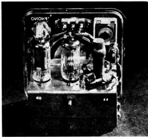
The plastic cover (removed in this view) is held to the chassis by the protruding screw.
