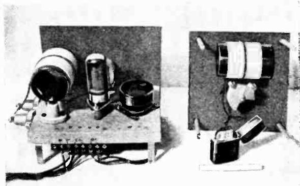
Legs for the transmitter are formed by two metal angles in back, and the bottom of the panel in front. The two stand-off insulators at the far left support the link-coupling coil, which is made of two turns of insulated wire around the center of the plate coil. Underneath the baseboard, mount the two R.F. chokes, the two by-pass condensers, and the 5,000-ohm cathode resistor, as shown at the right.
