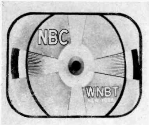
**Height control** is misadjusted. Notice the elongated circle showing that the picture is stretched out vertically. The adjustment is one of the "fixed controls" at the back of set.
