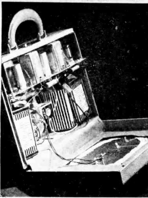
A piece of flat brass, cut to fit snugly across the upper part of the case, is used as a chassis. The lower portion of the cabinet is given over to the speaker and batteries. One 1.5-volt A and two 45-volt B batteries supply the set with power. The loop antenna slips under the lid of the case.
