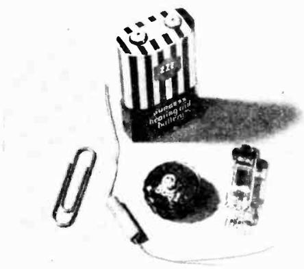
A few of the tiny components. Note the small condenser, volume control, tube, and battery.
