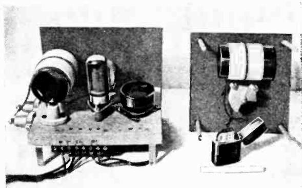
Legs for the transmitter are formed by two metal angles in back, and the bottom of the panel in front. The two stand-off insulators at the far left support the link-coupling coil, which is made of two turns of insulated wire around the center of the plate coil. Underneath the baseboard, mount the two R.F. chokes, the two by-pass condensers, and the 5,000-ohm cathode resistor, as shown at the right.
