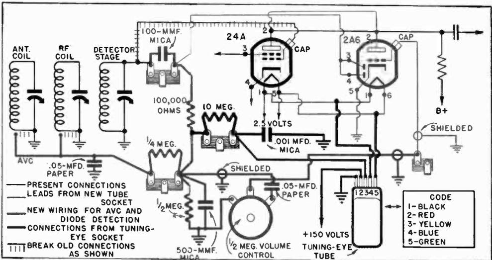
Fewer than a dozen wired connections are needed to add an eye to a set that has AVC. But what about the other ones? Here the job is slightly more complex, but it is even more worth while in terms of improved performance. Adding a diode detector and tuning eye should reap dividends in improving tone quality as well as ending blasting and off-station tuning.
