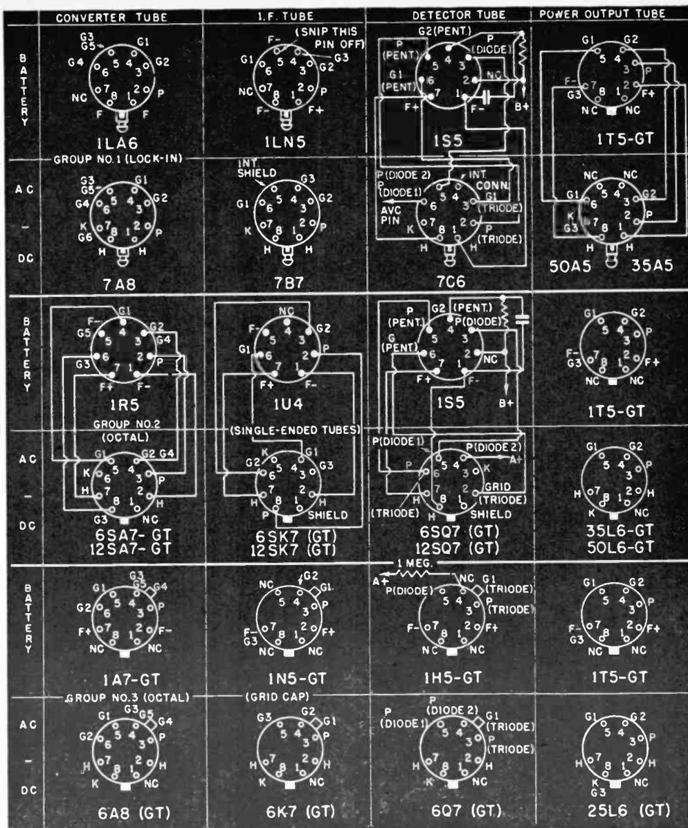
Pick your tube lineup. Battery substitutes or adapter sockets are given. All are top views.
