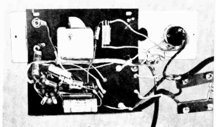
Wiring must be kept reasonably compact, but if small parts are used, no special crowding is necessary. Note the small 360-mmf. tuning condenser, and the miniature fixed crystal detector on its right.
