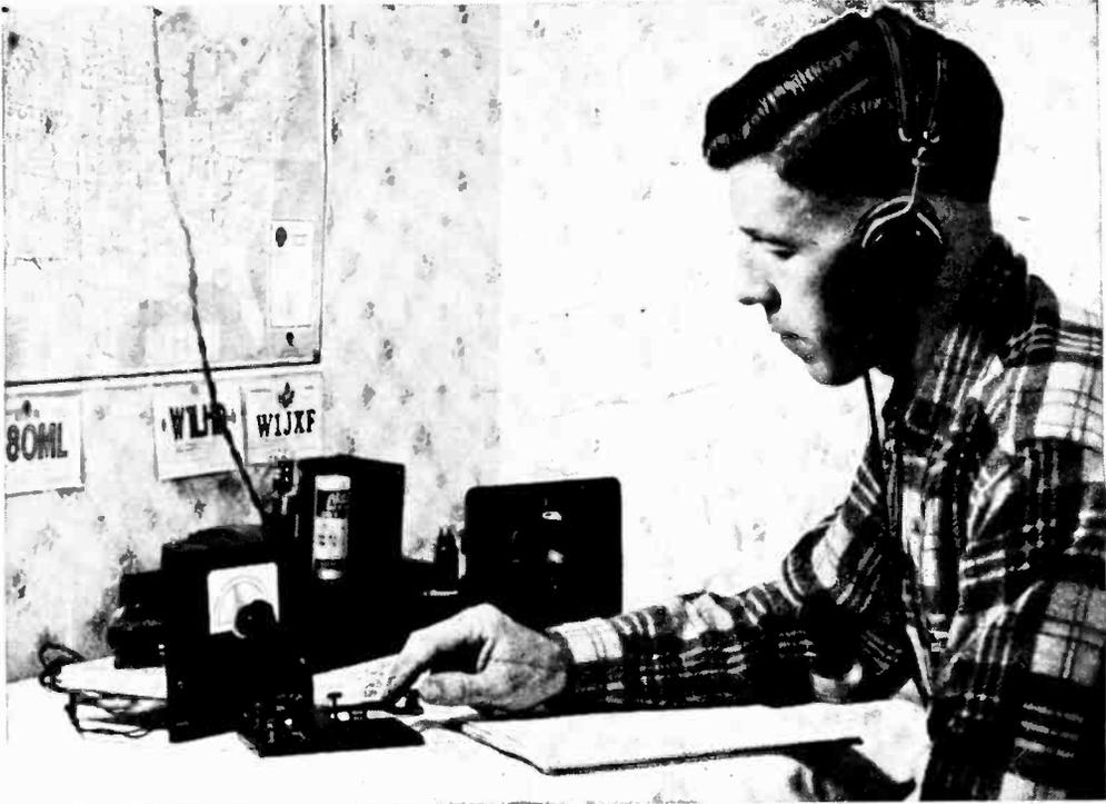
To check the frequency of your signal, separate your receiver and transmitter, and listen in on yourself.
