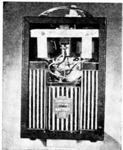
but does away with the C battery; the filaments of the tubes are wired for 1.4-volt operation. Place a small shield over the tube to reduce R.F. pickup from the tank coil.
