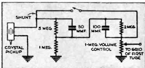
used to disconnect the filter when old-style records—still the most common—are being played.—JOHN W. CAMPBELL, JR.
