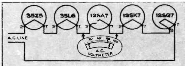
gives a reading of about 110 volts. If the filament should close during the test, the voltage will drop to its normal value for the tube.—G. BOLTON.
