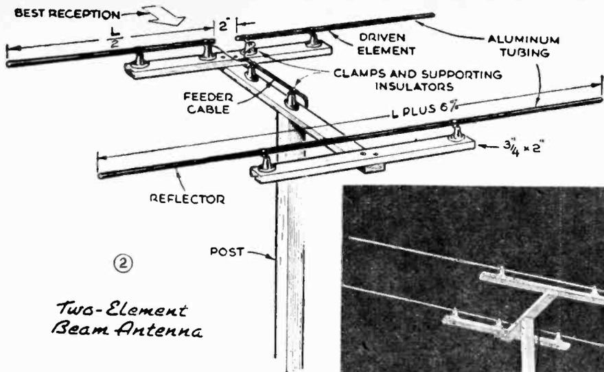
Two-Element Beam Antenna
