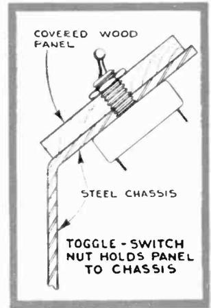
The chassis is a 6" by 6" metal sheet bent to conform with the slope of the wood panel. The cabinet is covered with artificial leather both inside and out.
