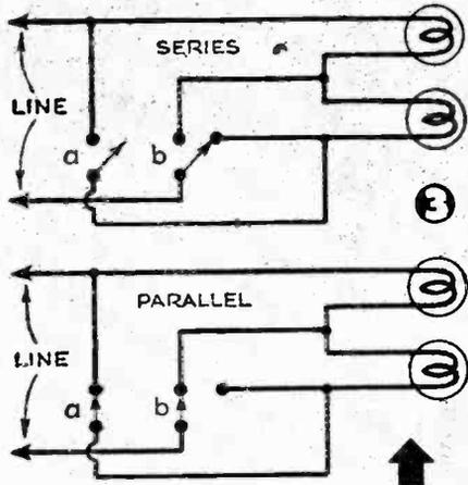
NOT having a double-pole, double-throw switch on hand, a photographer connected a S.P.S.T. switch *a* and a S.P.D.T. switch *b* as above to throw two flood lamps from series to parallel or vice versa. As all worked well in the positions shown, he considered himself lucky. Why was he even luckier than he thought?
