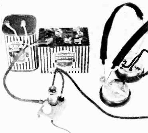
For test purposes standard  $1\frac{1}{2}$  and  $22\frac{1}{2}$ -volt batteries were used, but a penlight cell and a miniature B battery would provide a power supply hardly larger than the radio itself.
