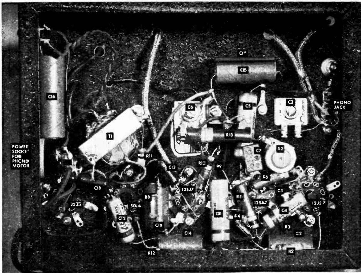
Although there is ample room on both sides of the chassis, parts should be closely grouped.
