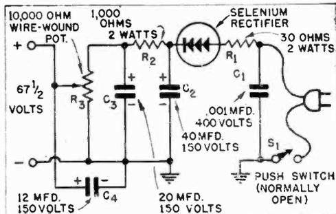
Wiring shown is for a metal chassis. To make the unit still safer, use a plastic panel, a DPDT switch, and connect all grounds together.
