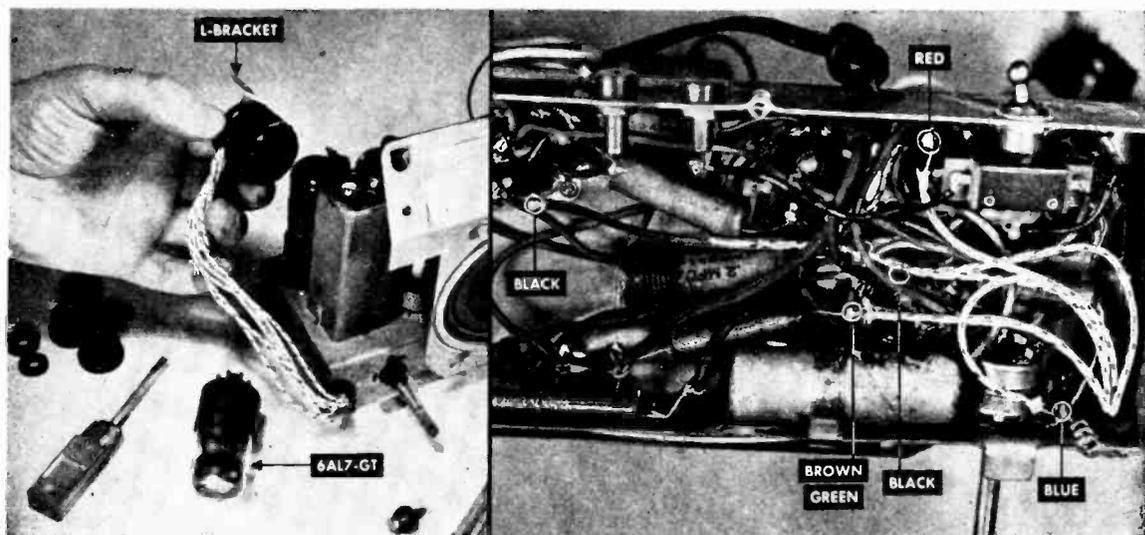
An indicator-eye assembly consists of a wired socket and mounting hardware. The L-bracket was used here instead to save cabinet space.
