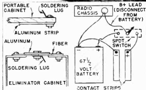
Contact strips are added to the bottom of the radio. These must line up with the contacts on the eliminator. The outer one is negative.
