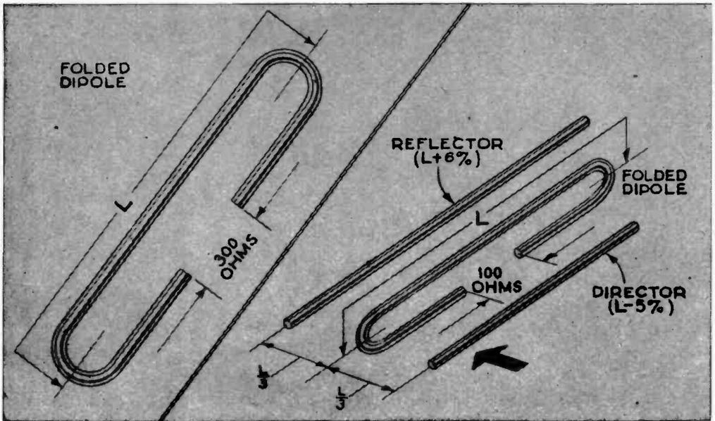
The folded dipole has a broad directional pattern, which is desirable in localities that have
