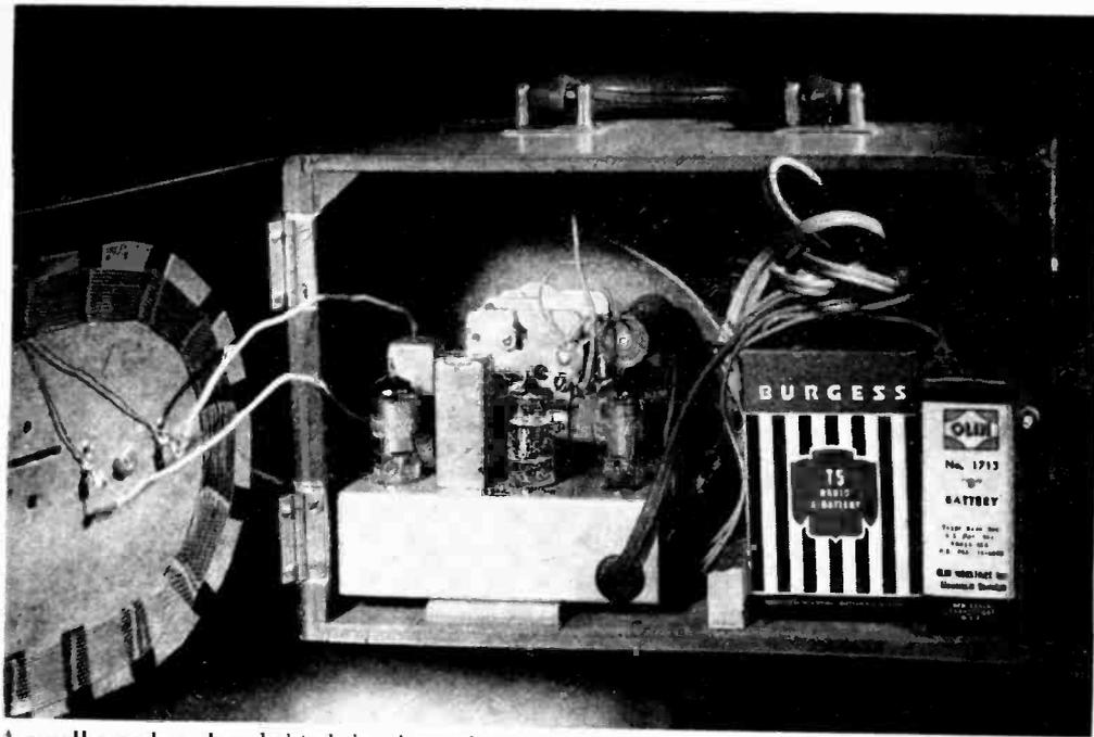
A small wooden cleat behind the chassis keeps it from sliding back in the cabinet. Cleats are
