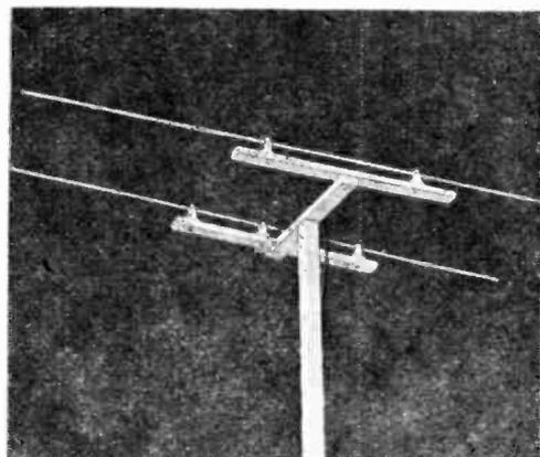
As can be seen in the drawing above, the two-element beam antenna consists of a half-wave dipole, now called the driven element, and a reflector. The latter isn't connected.
