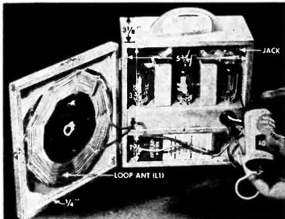
**A grid cap** snaps on the positive contact of the single A cell. Slid between cardboard tube and case, a split paper clip takes the other lead.
