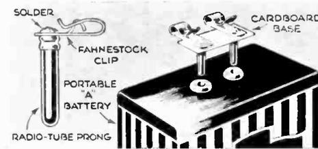
**PLUG-IN ADAPTERS.** Prongs from burned-out radio tubes secured to a cardboard base enable you to connect plug-in type portable radio batteries anywhere. Three prongs are needed for a "B" battery having a 22-volt terminal. Make sure the leads can't be accidentally shorted.—C. E. WARD III.
