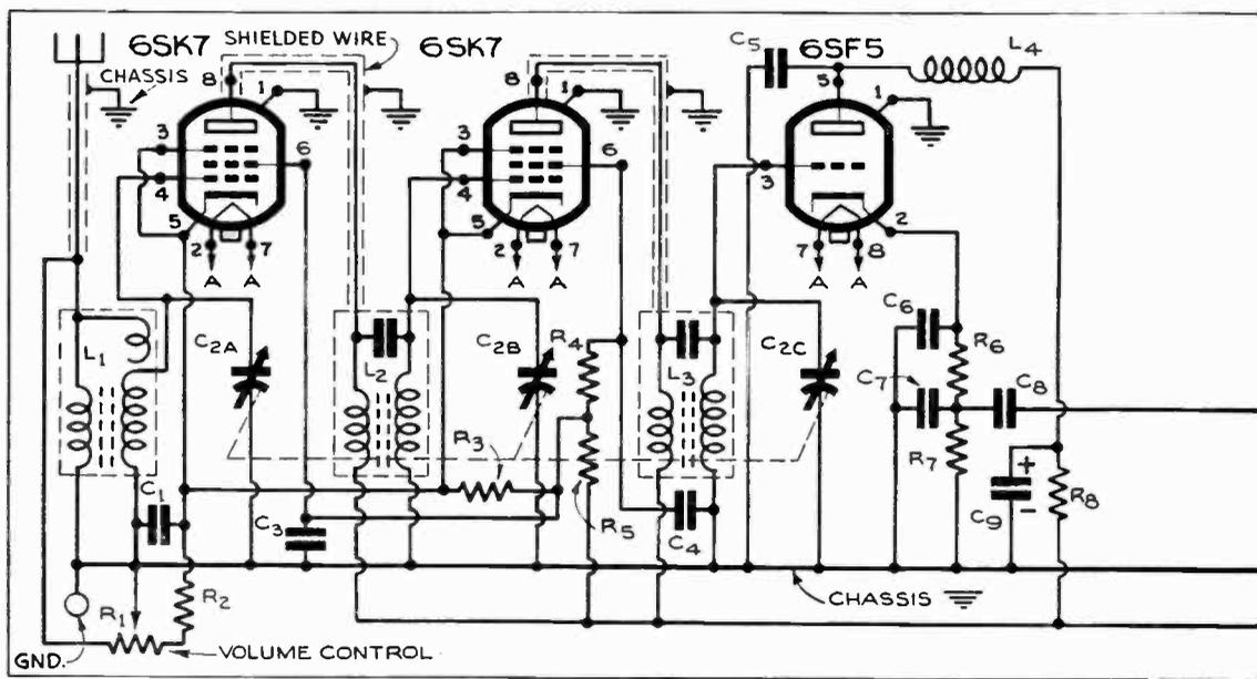
in the photographs that the three basic sets of components—RF, power supply, and detector-audio—are grouped and placed at maximum distance from each other. Especially in a circuit of this sort where detection and amplification give such faithful reproduction of the signal that passes the RF stages, it is important that stray pickups be held to a minimum. In addition to spacing, therefore, shielded conductors are used
