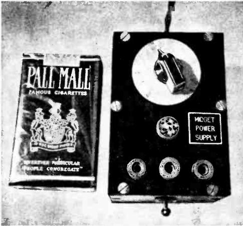
A small bakelite box houses the midget rectifier. The voltage control, pilot light, and output jacks are conveniently placed on top of the cabinet.
