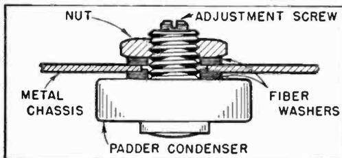
The paddler condensers must be insulated from the chassis. Use two fiber washers as shown.
