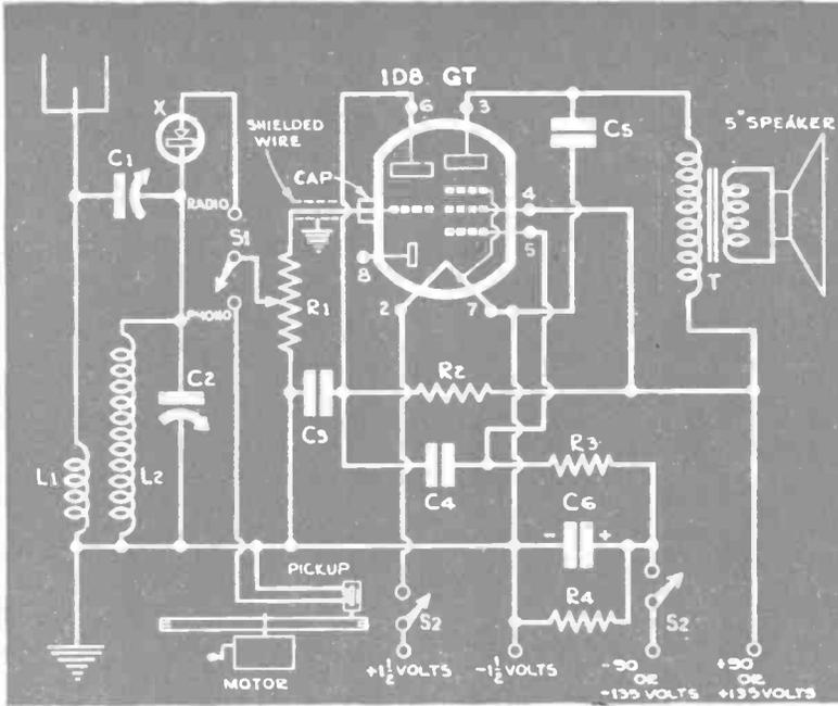
This one-tube circuit actually includes a two-stage amplifier fed either by the pickup or by the tuned circuit and detector. Parts are keyed to the list at the bottom of the next page.
