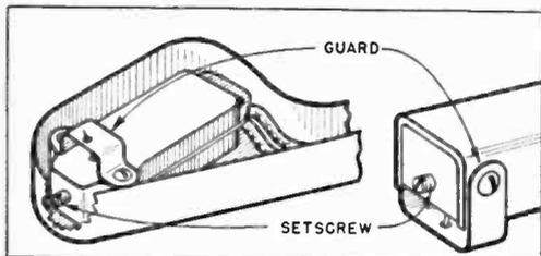
PHYSICAL abuse is a frequent cause of crystal-pickup failure. This may be avoided by installing a permanent-needle type of cartridge with a guard or by building a guard for your present pickup.
