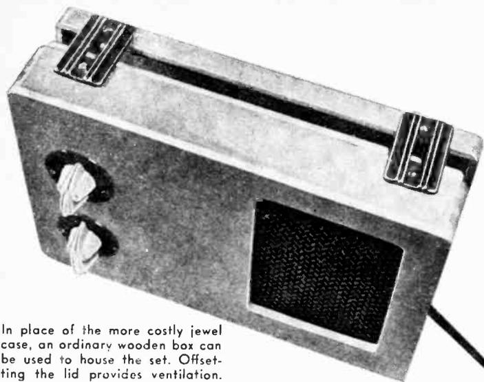
In place of the more costly jewel case, an ordinary wooden box can be used to house the set. Offsetting the lid provides ventilation.
