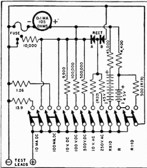
Pushbutton selector switches or individual toggles are used here to simplify switching.
