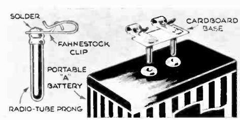
**PLUG-IN ADAPTERS.** Prongs from burned-out radio tubes secured to a cardboard base enable you to connect plug-in type portable radio batteries anywhere. Three prongs are needed for a "B" battery having a 22-volt terminal. Make sure the leads can't be accidentally shorted.—C. E. WARD III.
