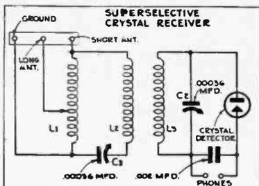
Two separate tuned circuits enable this receiver to distinguish between two or more powerful signals. The alligator clip is used to centertap the antenna coil, L1, when a long aerial is available.
