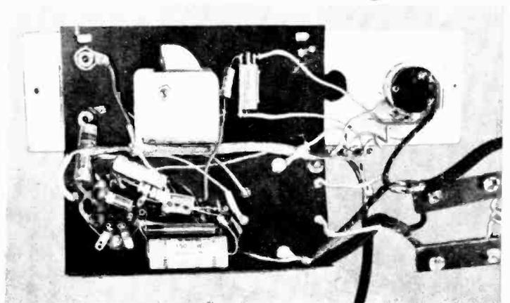
Wiring must be kept reasonably compact, but if small parts are used, no special crowding is necessary. Note the small 360-mmf. tuning condenser, and the miniature fixed crystal detector on its right.
