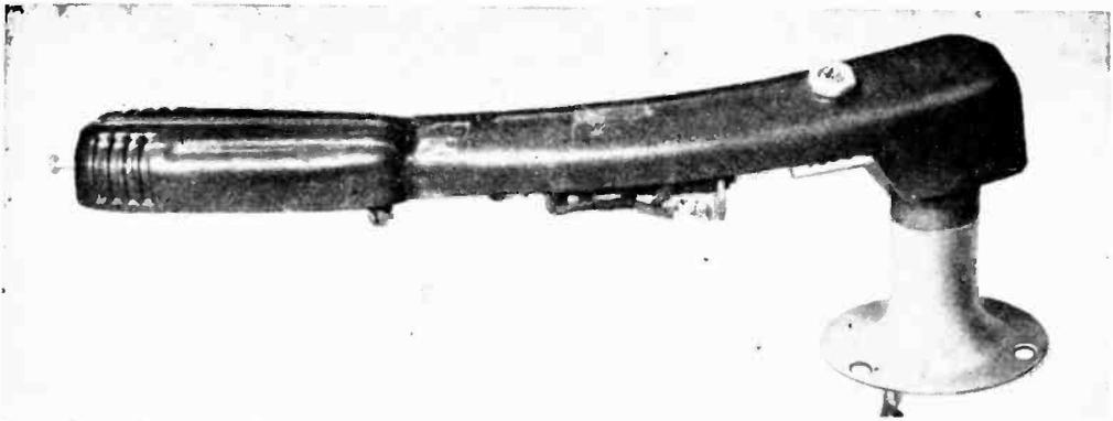
Complete phono oscillator, built into the arm of a pickup, plays records through any nearby
