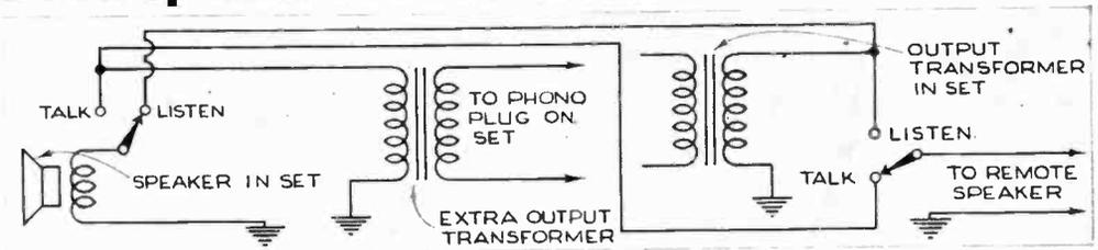
RADIO receivers having sufficiently high audio gain will double as intercoms with the addition of an extra speaker and transformer. A single wired connection to the remote speaker is sufficient, since the re-
