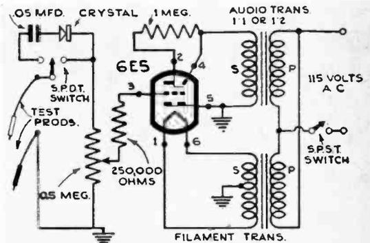
The S.P.D.T. switch on the input side cuts in a fixed crystal detector for testing A.C. circuits.
