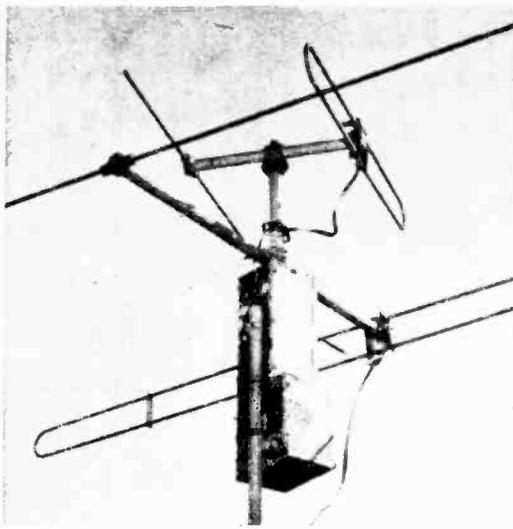
**Motor-driven antenna** is governed by a switch located at the receiver. A three-wire cable brings power to the roof; the rest of the mechanism is sealed inside a weathertight box.
