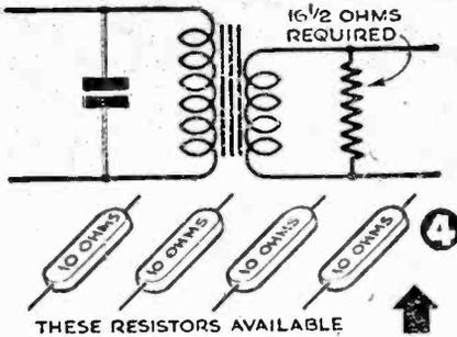
A RADIO engineer, needing a 16½-ohm resistance across an amplifier transformer for testing purposes, found he had nothing but four 10-ohm resistors in his parts drawer, which therefore had to serve. How did he connect them?
