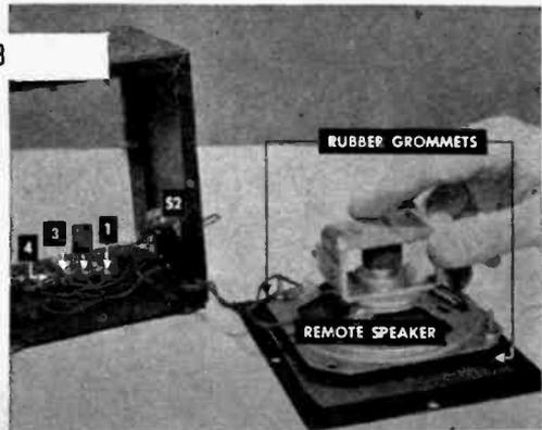
contact terminal strip housed in a 4" by 5" by 6" metal box. Stack a couple of rubber grommets or washers on the screws that hold the speaker to space it back of the panel.
