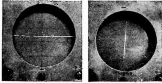
Since the oscilloscope is an enormously sensitive test instrument, it needs many controls. A useful panel arrangement is indicated at the left. The three views at the right illustrate the operation of the three amplifiers. Horizontal and vertical signals are shown above; the lower picture shows a vertical signal timed by a horizontal sweep.
