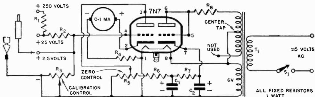
14. Half of the dual triode serves as a power rectifier, the other half as the meter tube.
