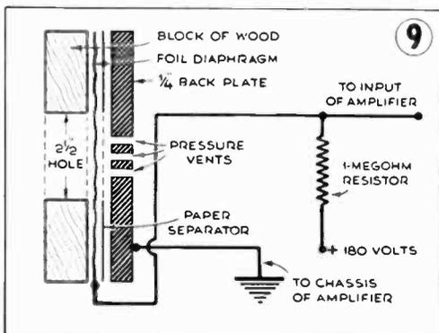
connection. Cut a  $2\frac{1}{2}$ " hole in a thin sheet of paper 5" square, lay it on the foil, and put on top of that an absolutely flat  $\frac{1}{4}$ " by 5" by 5" sheet of aluminum or brass in which two or three  $\frac{1}{4}$ " holes have been drilled near the center. Clamp the pieces, as in Fig. 7, and the mike is ready for action (Fig. 8). The wiring diagram is shown in Fig. 9.
