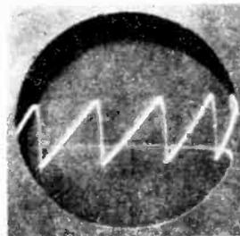
voltage applied to the horizontal-deflecting plates, then, will sweep the beam right and left at a rate equivalent to the frequency. The trace of this beam on the screen, however, will appear only as a straight horizontal line (Fig. 2) since each side motion only covers the trace of the preceding electrons.
