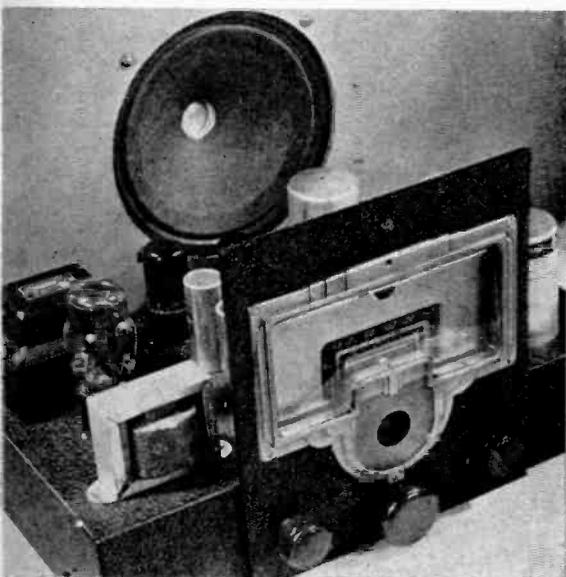
Working into a single dynamic speaker, the tuner becomes a complete, better-than-average receiver. It separates stations sharply, has ample room volume, and its fidelity and tone are excellent.
