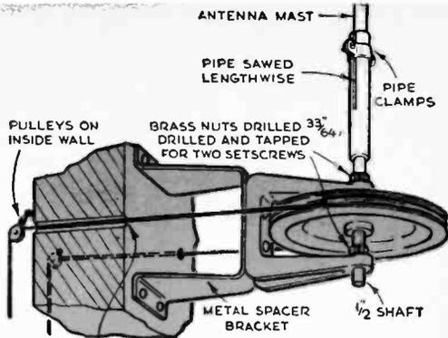
Moving the position indicator shifts the roof antenna in any desired direction. Equal pulley diameters give a 1-to-1 ratio of pointer to mast.
