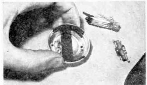
Insulate the bottle-cap chassis with tape. The holes in back are for mounting; drill two more in the rim to clear battery and phone cables.
