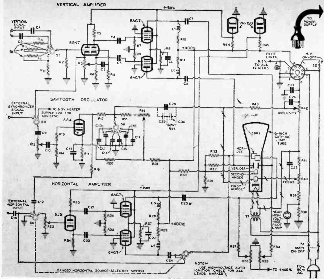
to prevent attenuation of high-frequency signals. But this also means that the cathode follower can't follow signals in excess of about 20 volts. It is in order to boost this range up to about 600 volts that the special voltage divider R1 is used.
