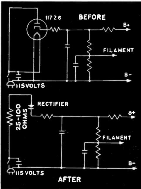
**P**RACTICALLY all commonly used rectifier tubes are now replaceable by dry-disk selenium rectifiers. They not only take the place of hard-to-get tubes, but are also smaller, cooler and quicker in operation (because they have no filaments to warm up), and they won't burn out or break under conditions that generally damage tubes.
