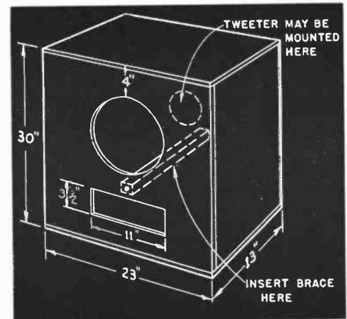
6. A bass-reflex cabinet for a 12" speaker may be made to these dimensions. Use  $\frac{3}{4}$ " plywood.
