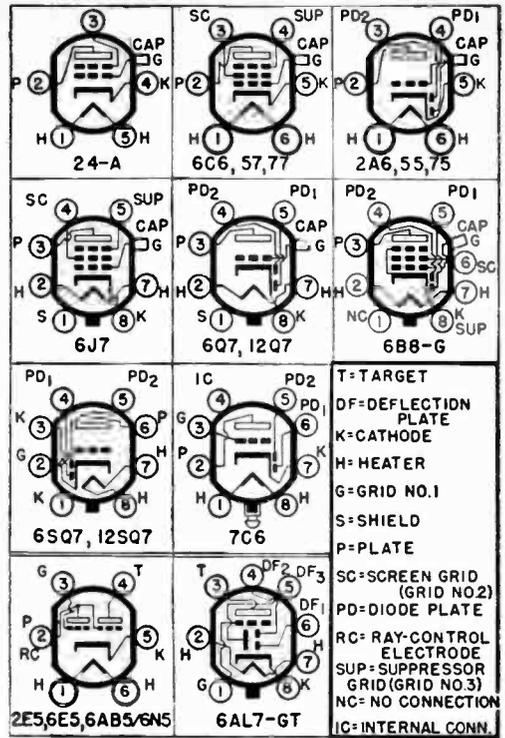
For convenience the base connections (bottom view) of most detector tubes are shown above.
