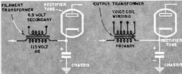
8. Filter chokes may be improvised from either filament or output transformers. One winding isn't used; it can even be open or shorted.
