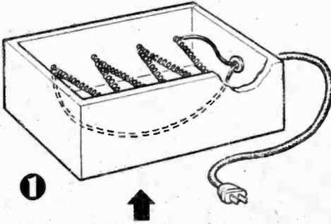
TO MAKE a photographic dryer, Smith used a 600-watt replacement coil sold for use in toasters and stretched it over a series of hooks inside an asbestos-lined box. But he found the wire heated to redness, scorched the prints, and threatened to burn the box itself. To halve the amount of heat, should he cut the resistance wire in half, add a second element in series, or connect another in parallel?
