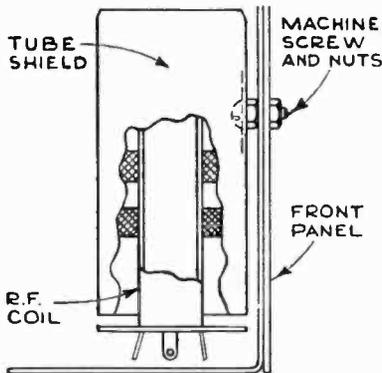
To prevent oscillation and distortion due to stray coupling, the RF coil must be shielded. A suggested method for isolating the coil is to enclose it in an old tube shield which is attached to the chassis as shown above.
