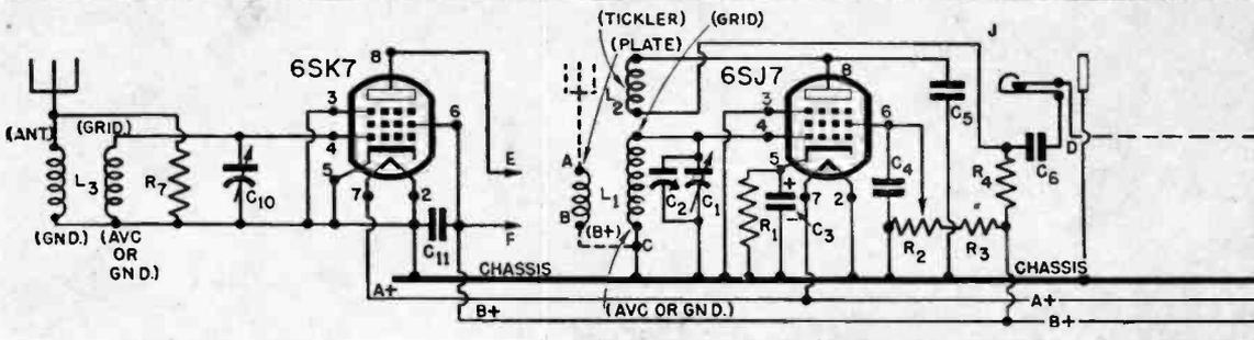
the primary winding of the RF coil. By induction the coil transfers them to the secondary winding where the tuning condenser (in parallel with this part of the coil) selects one particular signal from the jumble.
