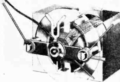
A D'Arsonval movement, shown here in phantom, indicates DC when the coil is energized.
