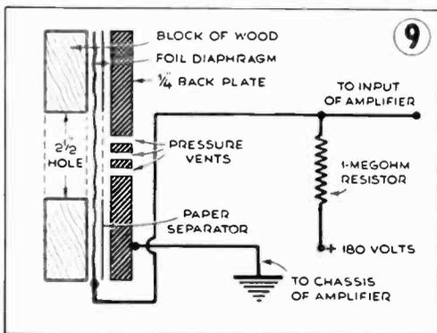
connection. Cut a  $2\frac{1}{2}$ " hole in a thin sheet of paper 5" square, lay it on the foil, and put on top of that an absolutely flat  $\frac{1}{4}$ " by 5" by 5" sheet of aluminum or brass in which two or three  $\frac{1}{4}$ " holes have been drilled near the center. Clamp the pieces, as in Fig. 7, and the mike is ready for action (Fig. 8). The wiring diagram is shown in Fig. 9.
