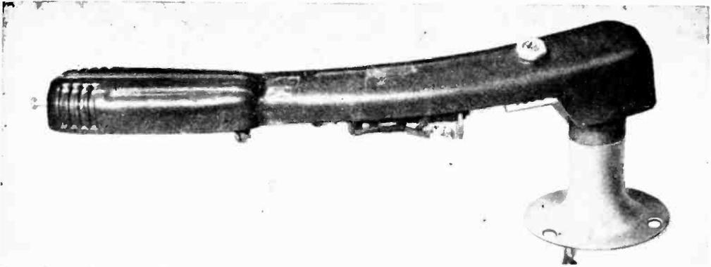
Complete phono oscillator, built into the arm of a pickup, plays records through any nearby
