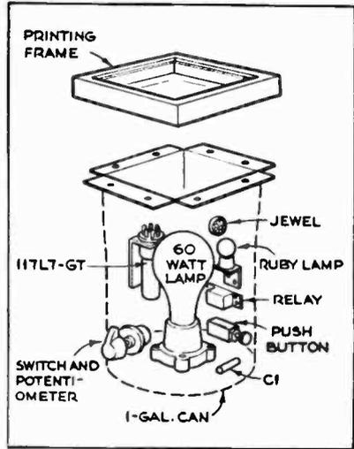
THOSE who go for canned fruit in a big way, or can get a 1-gal. fruit can from a boarding house, have a good photo accessory at hand. Such a can is lighttight and just the right size to hold this electronically controlled contact printer.
