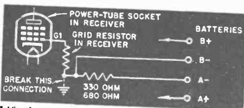
Lift the grid resistor of the output tube from ground and connect it to B-minus. Insert a bias resistor between this junction and A-minus.
