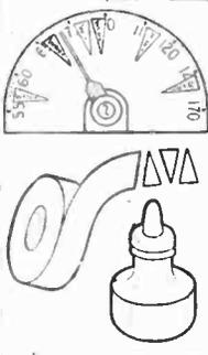
WEDGE-SHAPED bits of cellulose tape make station settings easy to locate. Lettered with India ink and placed in appropriate spots on the dial, they help you tune in where the light is poor without having to remember wavelengths of favorite stations.—G. E. HARRINGTON.
