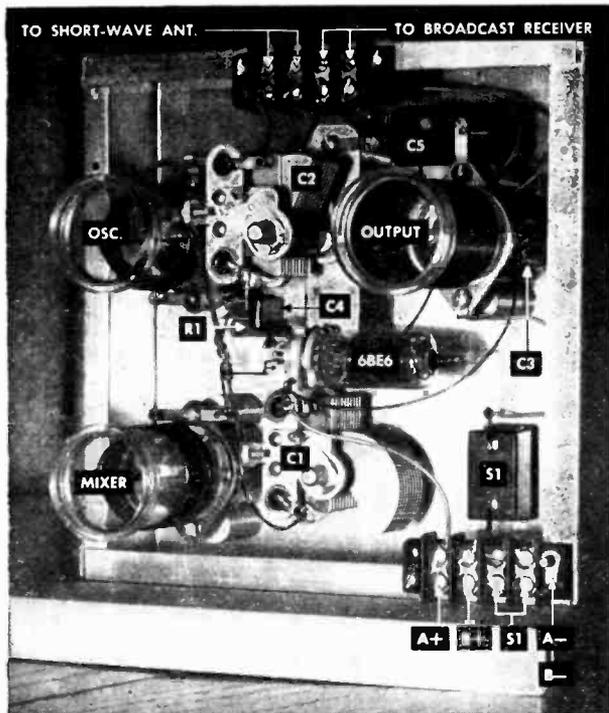
Coil sockets and the oscillator capacitor are raised from the chassis by insulated spacers. Solder all leads that go beneath these parts before you actually fasten them into position.
