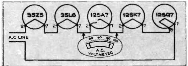
gives a reading of about 110 volts. If the filament should close during the test, the voltage will drop to its normal value for the tube.—G. BOLTON.
