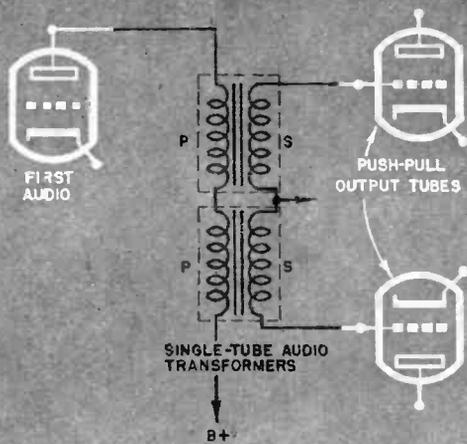
6. Two single-tube audio transformers make a neat replacement for a push-pull transformer.
