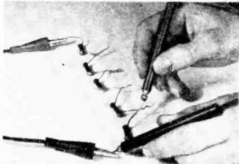
Approximate values of resistors can be determined as at B. By comparing the meter deflection after a timed wait when the condenser is shunted across an unknown resistor with that obtained from a known one, you can gauge the unknown value.
