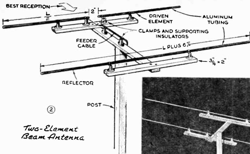
Two-Element Beam Antenna
