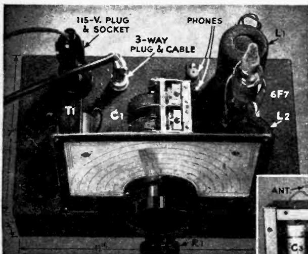
The size of the metal chassis allows ample room for neat wiring. Note the tiny fixed crystal detector X1; it takes the place of an extra tube, but is no larger than a 1/2-watt resistor.
