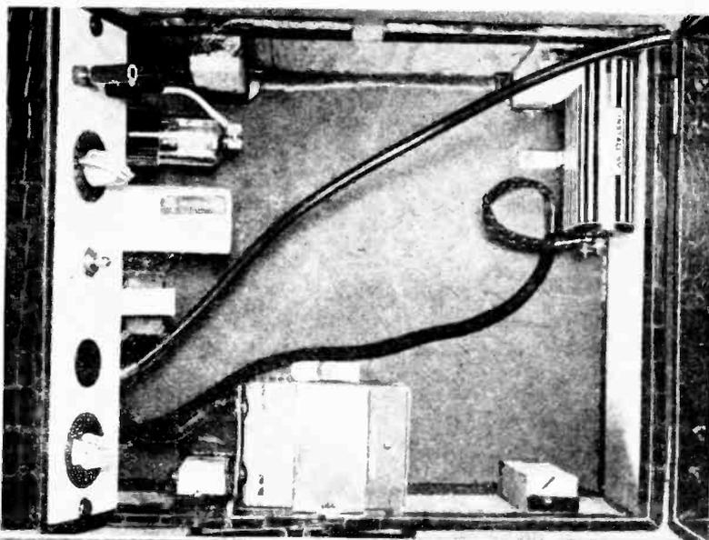
The control panel is shown below in close up. The knob on the left governs R1 and S2, the volume control and switch. To keep from draining batteries, turn off the switch when the set is not in use.
