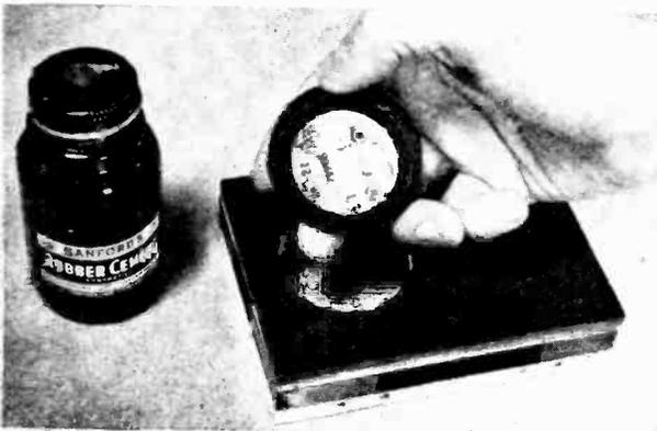
Cut a hole that will make a press fit for the rubber lip and cement the cartridge in place.
