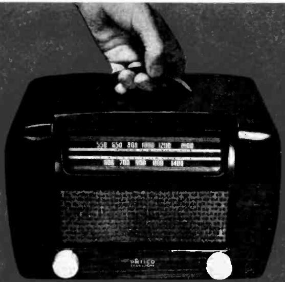
New tubes and some minor changes turn this midget radio into a self-powered portable—and back again.
