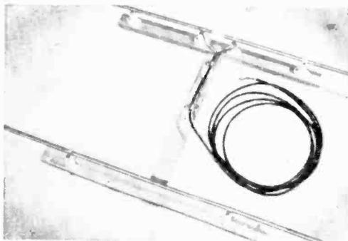
A two-conductor feeder cable is illustrated at the left. One conductor is soldered to each half of the dipole; the other ends go to set.
