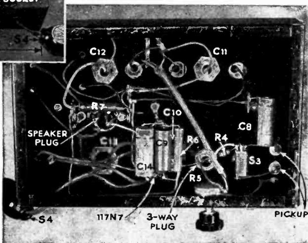
filtered through R7 and C12. Tapped off the choke, the voltage that reaches the plate of the 117N7 is higher than the one that gets to the screen.
