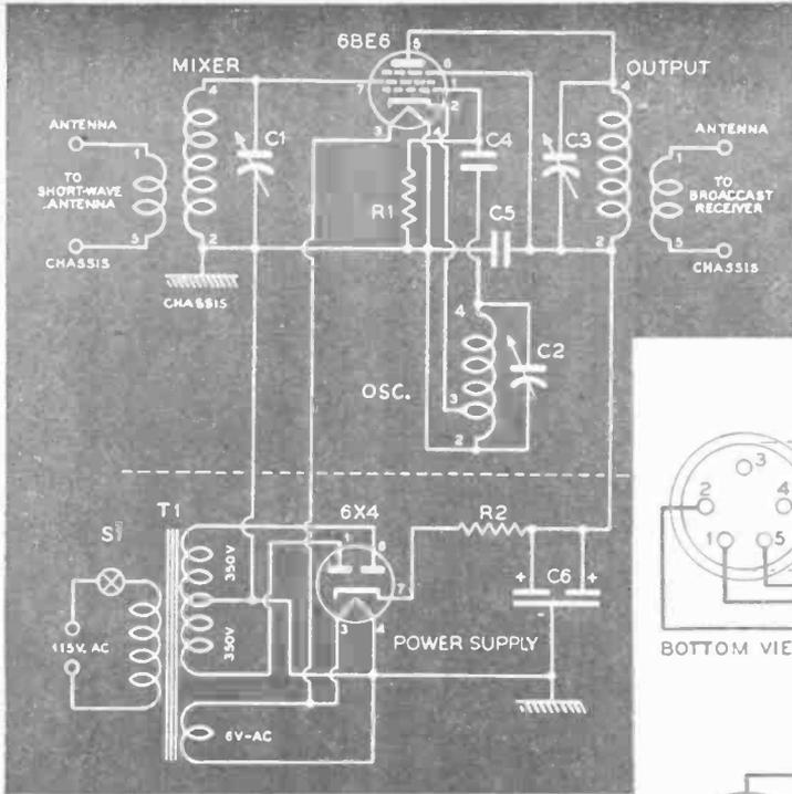
Schematic diagram shows how to wire the simple one-tube converter and its power supply. If possible, follow the parts layout shown in photos, keeping all signal leads short.
