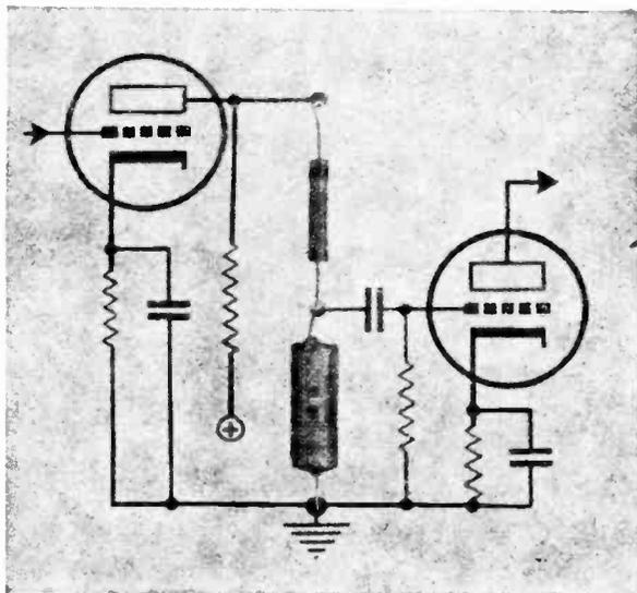
Used between amplifier stages, this type of filter requires an extra condenser-resistor arrangement in the coupling circuit.
