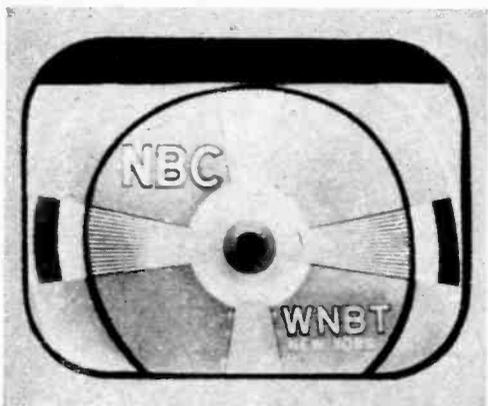
**Vertical centering** here just isn't centered. It would be the same if the picture went off screen at the top. This is also a rear control but is not made accessible on all types of receiver.
