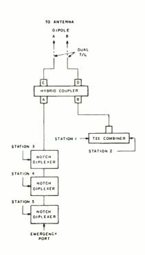
Typical five-station shared-antenna scheme for FMbroadcast stations using a Type BFB- Panel Antenna.
