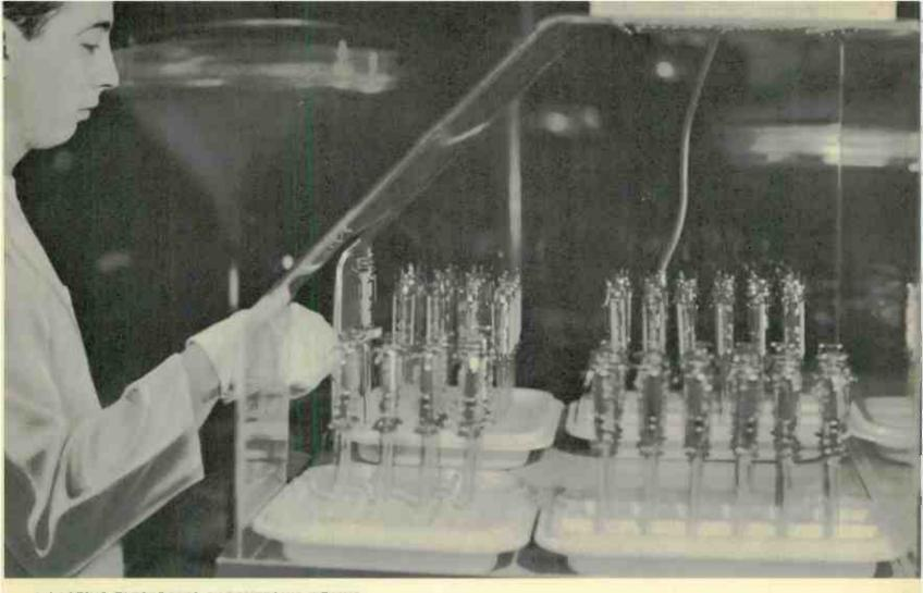
A LASTING ELECTRONIC PARTNERSHIP BEGINS Electron guns are kept dust-free in pressurized hoods after they arrive from the white room for an important and final stage: accurate positioning and saling of the gun in the neck of the bulb. As bulb and gun join forces, a lasting electronic partnership begins.
