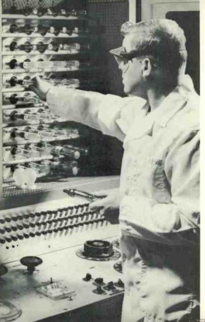
LIFE TESTS ASSURE ELECTRON GUN QUALITY Sample batches of electron guns are life tested above maximum ratings and closely scrutinized for electrical shorts, opens, and leakages. These tests provide more assurance of gun quality and long life.
