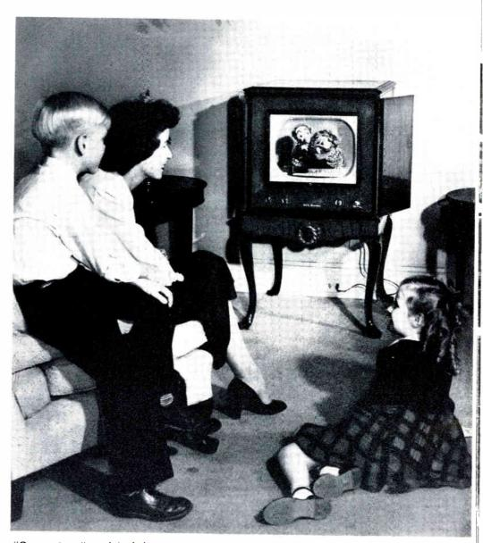
"Queen Anne" model of the RCA Victor television receiver equipped with a 16-inch metal-cone kinescope provides a direct-view picture of 126 square inches.
