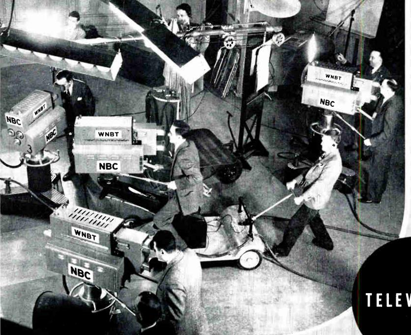
Image orthicon cameras focus on different parts of a television stage setting in an NBC studio.
