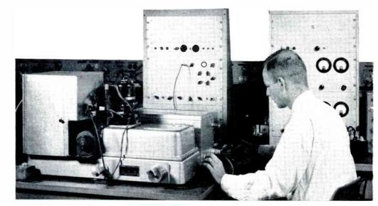
Receiving terminal of the RCA Ultrafax system of radio-television communication which is capable of handling written and printed documents at the rate of a million words a minute.
