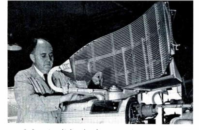
Radiomarine shipboard radar antenna being assembled.
