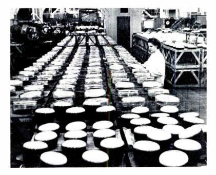
Glass television picture tubes, which are heated to almost 1300° F. in production, are given final inspection.
