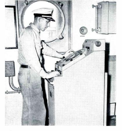
A ship's officer checks the location of other craft in the vicinity on the 12-inch scope of a Radiomarine 3.2-centimeter radar.
