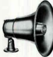
UNIVERSITY MODEL IB-A   | 25 watts<br>250-13,000 cps<br>90° dispersion<br>10 1/4" dia., 9" deep<br>In 4, 8, and 45 ohm impedances.                            |
