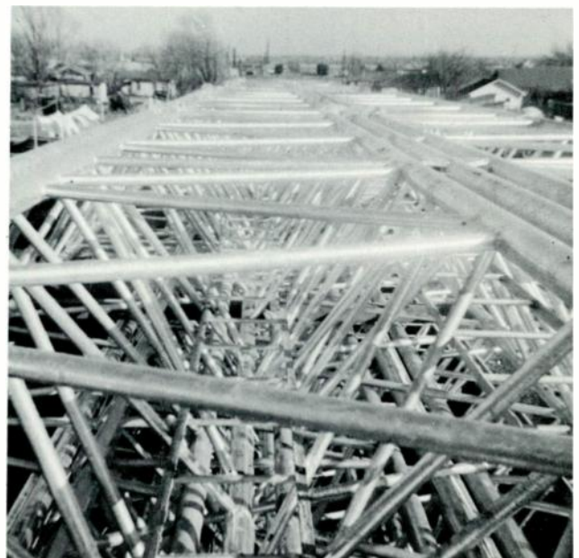
FABRICATED TOWER SECTIONS, AFTER COMPLETION OF HOT DIP GALVANIZE PROCESSING.
