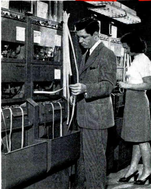
signals were made automatic through the use of paper tape to record the dots and dashes. For transmission, the ribbon of tape is perforated by a machine similar to a typewriter. A "Wheatstone" transmitter converts the perforations into dot and dash radio signals. In reception, the signals are recorded on tape by an ink stylus.
