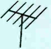
City listeners may complain of distortion, notwithstanding that the installation was made in an approved manner. Here we can suspect "multipath signal dispersion" or the interception of several signals at the antenna in an out-of-phase order. An FM yagi with 72 ohm line to tuner will minimize the trouble and the use of a rotator is recommended for locations where all of the stations received do not originate at a central location.
