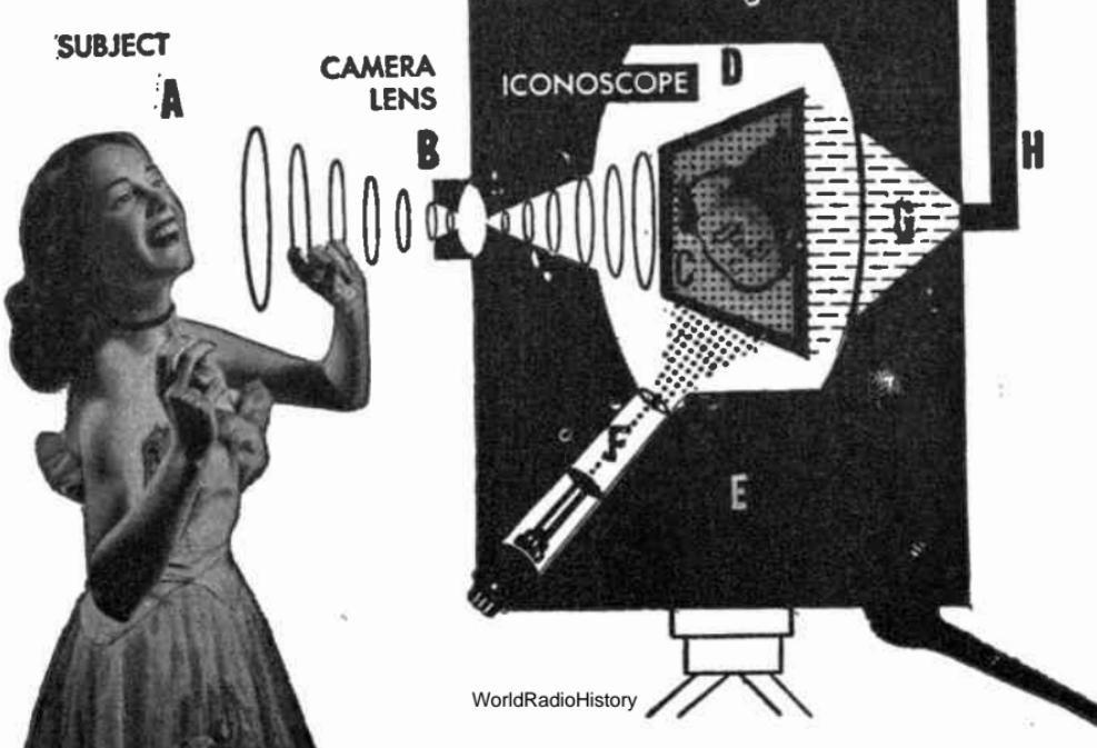
stream of electrons which plays across a fluorescent screen in the large end of a kinescope tube. Electrical impulses are converted by the tube into light. The varying degrees of light form the image of the person or scene on the screen of the television receiver. Actually a series of still pictures are being broadcast at the rate of 30 per second which, when observed, form a smooth continuity of action similar to motion pictures which operate at 24 frames a second.
