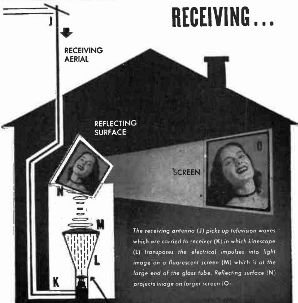
The receiving antenna (J) picks up television waves which are carried to receiver (K) in which kinescope (L) transposes the electrical impulses into light image on a fluorescent screen (M) which is at the large end of the glass tube. Reflecting surface (N) projects image on larger screen (O).
