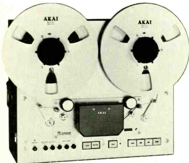
Section containing transport and transport controls.
