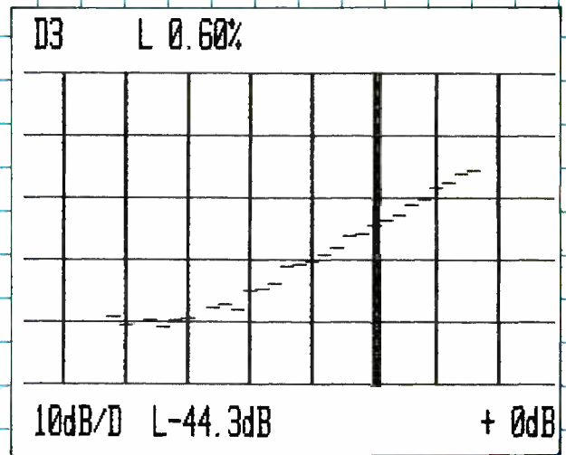
Fig. 9. Headroom for 3 percent THD using Scotch XS-11 was +12 dB; thus S/N with this tape is 87.5 dB (75.5 + 12) with dbx on.
