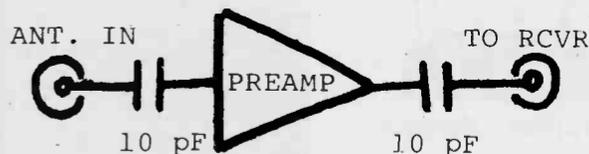
Input and output capacitors are reduced to limit low frequency response.
