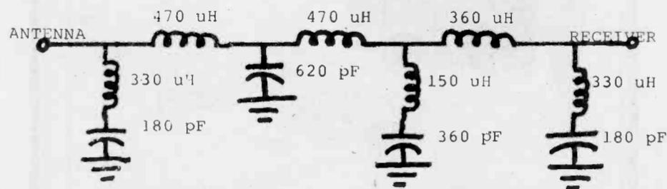
Q. Would any of your VLF enthusiasts like a diagram for a sure-fire AM broadcast band filter to put ahead of their 5-500
