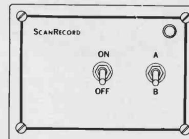
The recorder runs only when a message is received. It does not run when the scanner is just scanning. This lets you record a lot of traffic on one tape. In addition to scanners, it will work with any receiver that has a squelch control.
