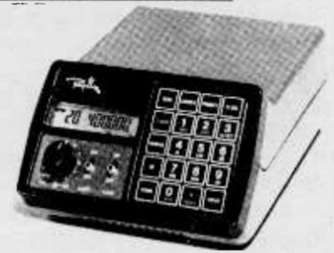
After some two years of premature announcements, the long awaited MX-7000 wide frequency coverage scanner is finally in limited distribution. Essentially the same in appearance and function as its precursor, the popular MX-5000, the 7000 includes the new 800 MHz "cellular" mobile band. Continuous frequency ranges are 25-550 and 800-1300 MHz, AM or FM on both ranges.
