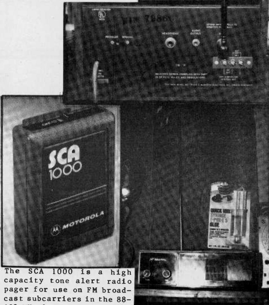
The SCA 1000 is a high capacity tone alert radio pager for use on FM broadcast subcarriers in the 88-108 MHz frequency range. The pager is activated by using Binary Digital Signaling. Photo courtesy Motorola.
