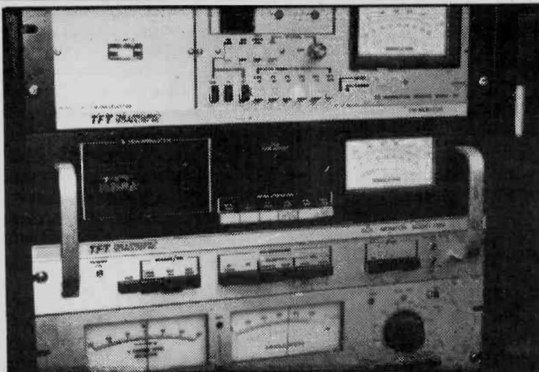
This terminal-like receiver demodulates subcarriers using FSK. Photo by Kevin Sager.
