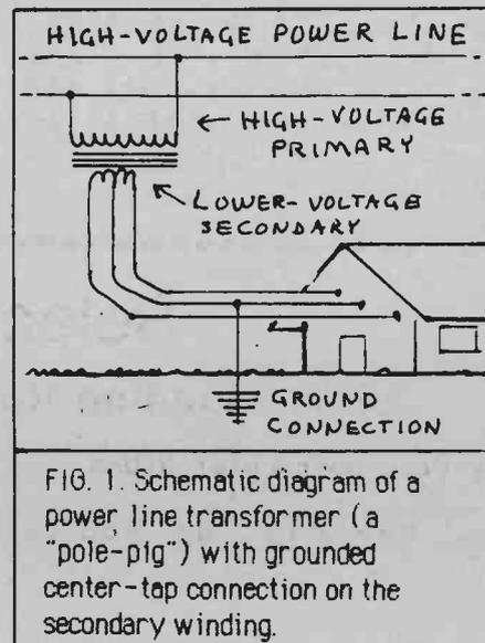
FIG. 1. Schematic diagram of a power line transformer (a "pole-pig") with grounded center-tap connection on the secondary winding.
