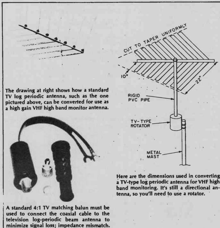
The drawing at right shows how a standard TV log periodic antenna, such as the one pictured above, can be converted for use as a high gain VHF high band monitor antenna.
