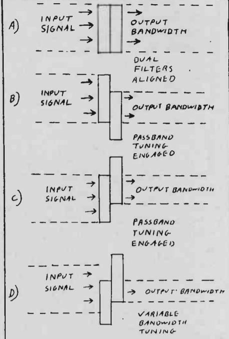
width filters in different IF stages may be adjusted relative to each other in order to obtain a continually variable bandwidth.
