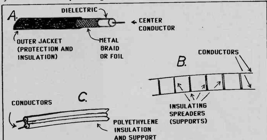
Figure 1. The three most commonly used types of transmission lines: coaxial cable (a); open-wire line (b); and twin-lead (c).
